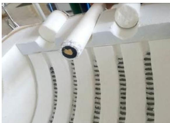
*Figure 3.6.* Assembly of the symmetric cell for EIS measurements in a split furnace.
