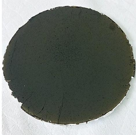
Figure 4.1. Synthesized LSC powders by thermal plasma collected on filter.
