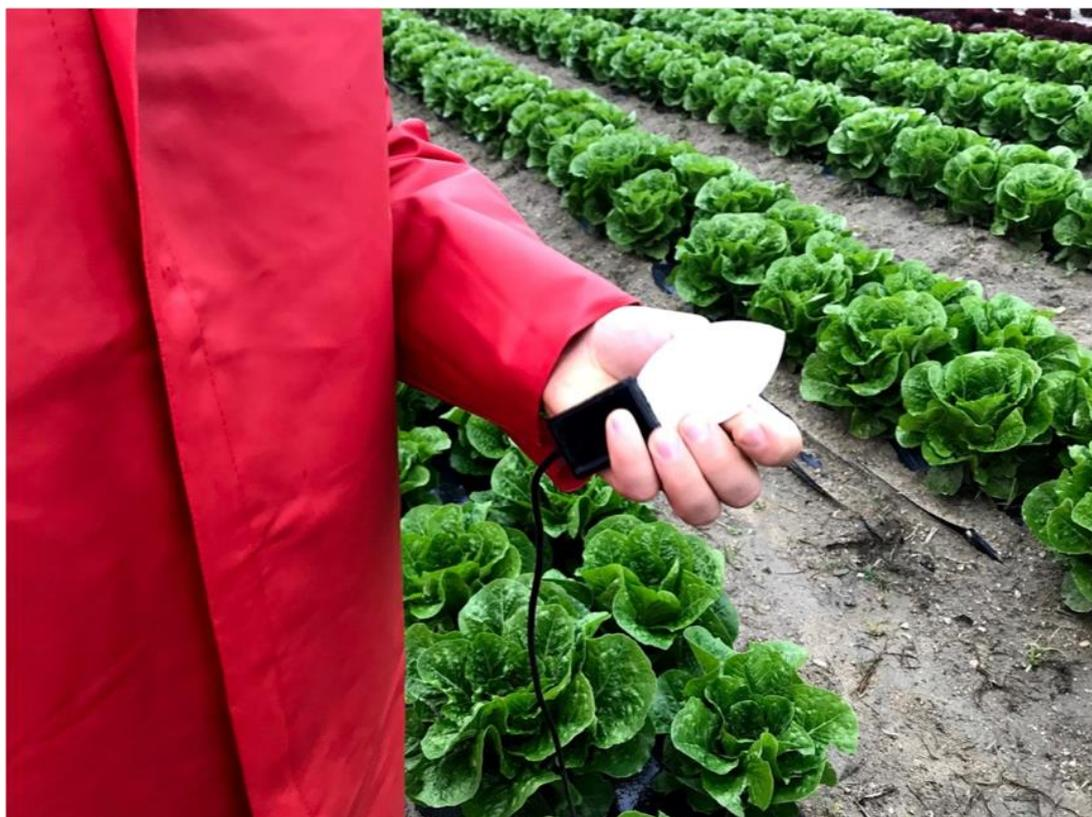
*Figure 7.1.* Humidity sensor placed inside the lettuce crops.
