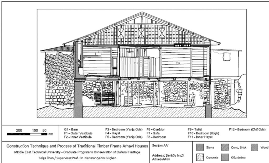
Figure 1.3. A section drawing of Şenköy 3 produced from the data taken from 3D point cloud
