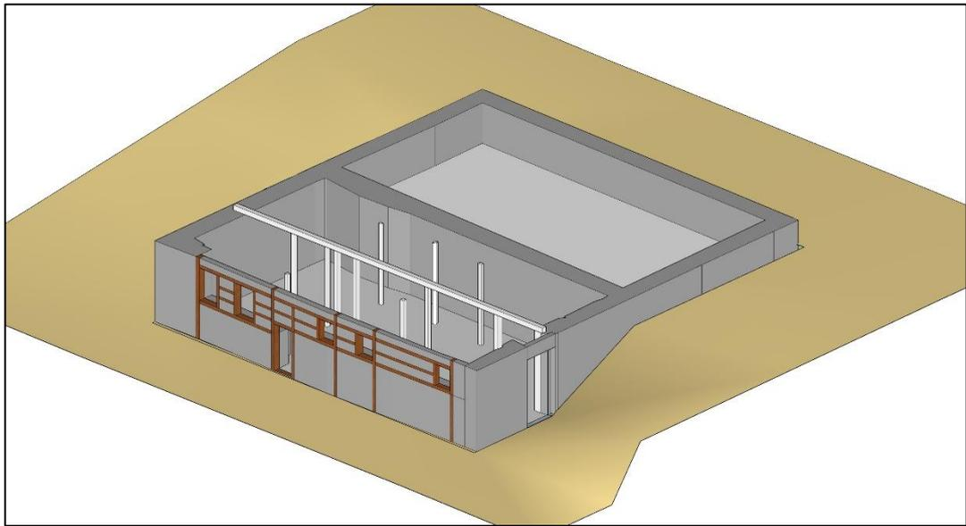
Figure 4.13. Timber frame lower wall of the ground floor of Şenköy 3
