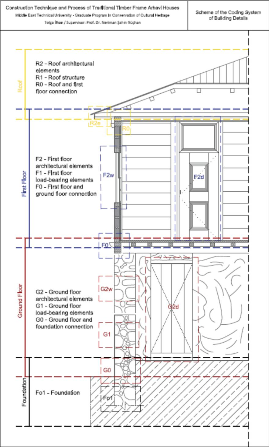
Figure 3.1. Scheme of the coding system of building details
