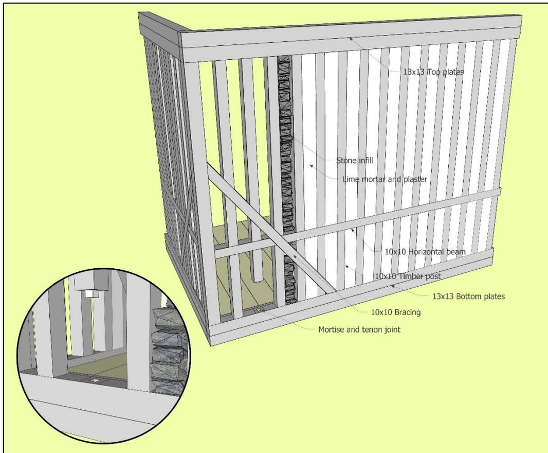
Figure 3.16. Construction detail of the çatma technique
