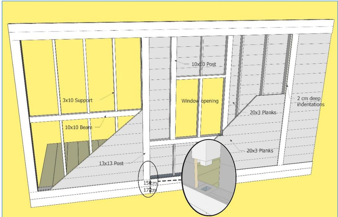
Figure 3.19. Construction detail of the timber infill technique.
