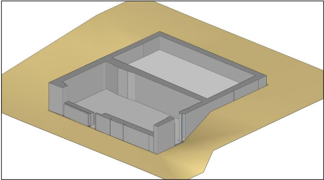
Figure 4.12. Masonry walls of the ground floor and foundation of Şenköy 3
