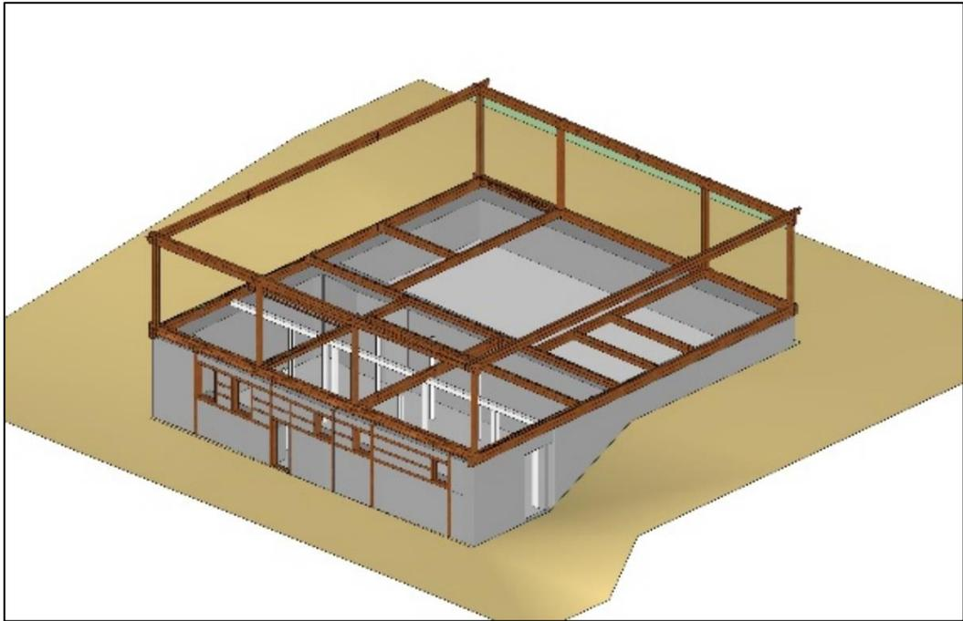
Figure 4.18. Post and beam system of the first floor
