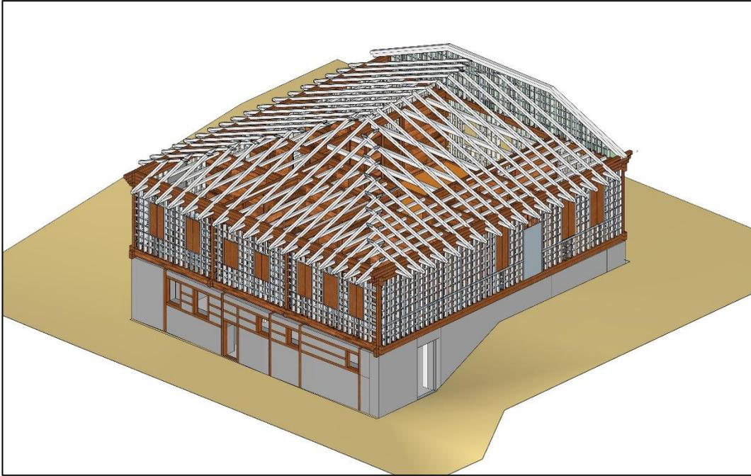
Figure 4.28. Construction of the roof structure
