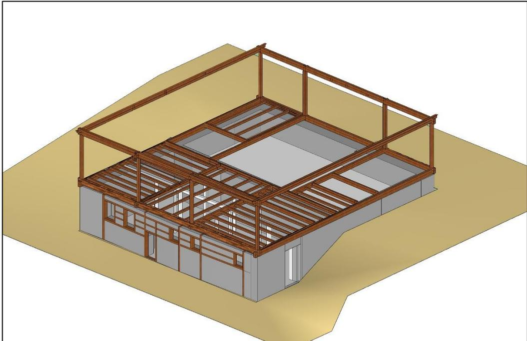
Figure 4.19. Placement of the floor joists
