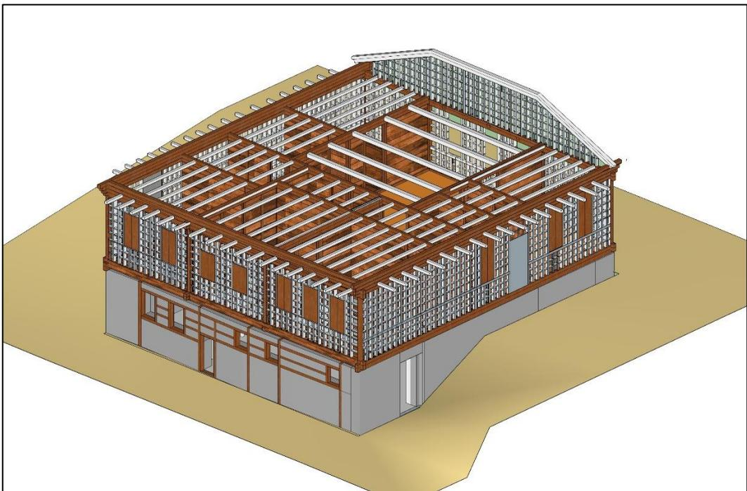
Figure 4.25. Placement of top plates of walls and ceiling joists, and construction of gable wall
