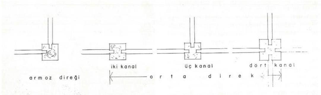
Figure 3.15. Grooving systems at timber posts (Çalma boğaz) (Özgüner, 1970)
