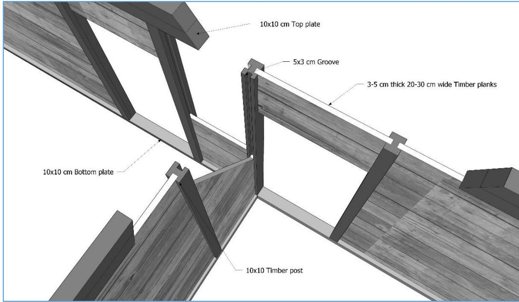
Figure 3.21. Construction detail of the taraba technique.
