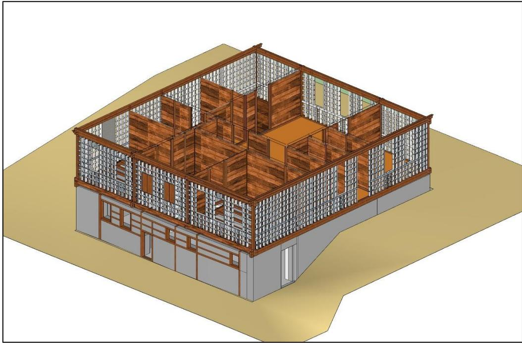
Figure 4.24. Construction of interior partition walls (taraba)
