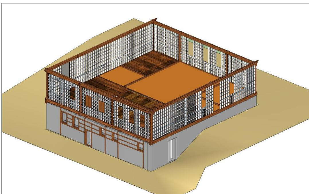
Figure 4.23. Construction of the dolma göz framing and floor coverings
