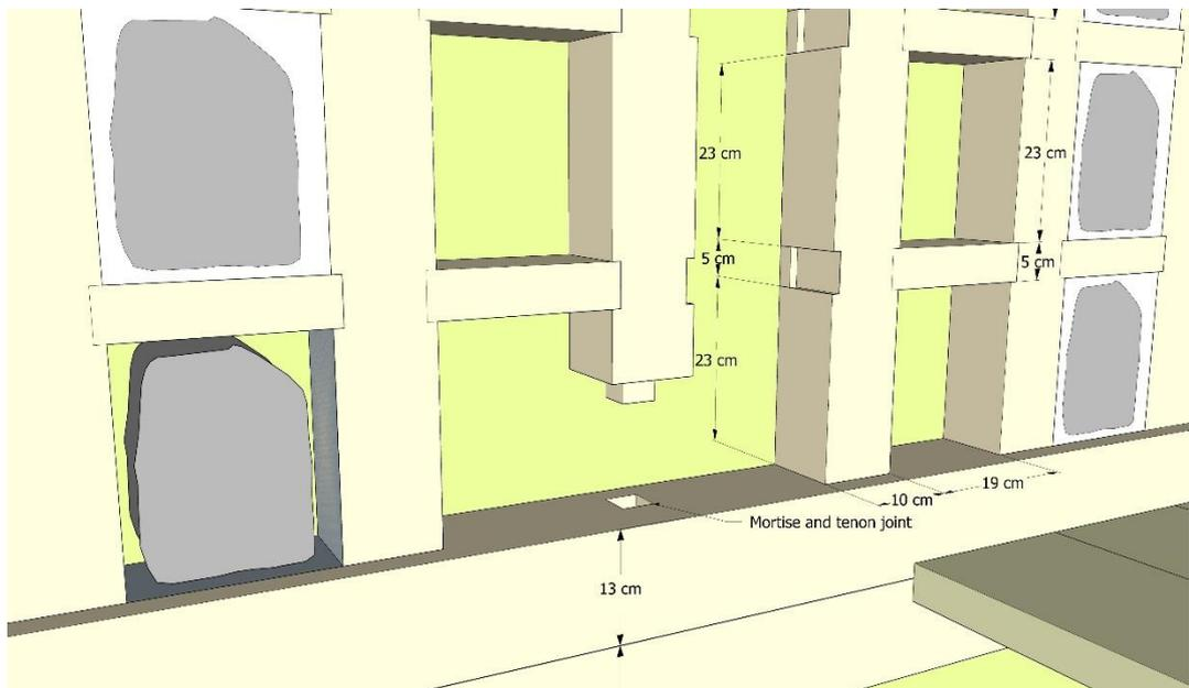
Figure 3.10. Construction detail of the dolma göz technique
