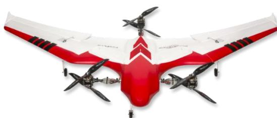
Figure 1.5. All coaxial tilt-rotor: *FireFly6* [42]
