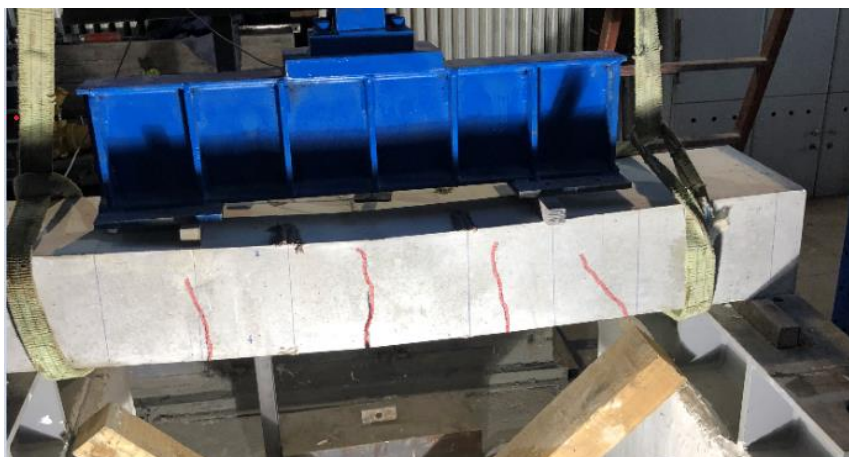
Figure 4-15 Location of cracks for Test beam -2 before failure
