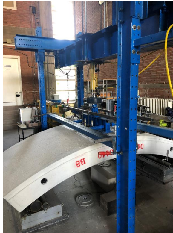
Figure 4-5 Test setup for full scale bending test
