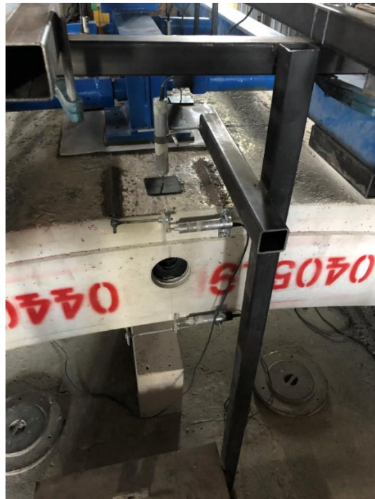
Figure 4-7 Additional LVDT's to measure compressive and tensional strain of the specimen
