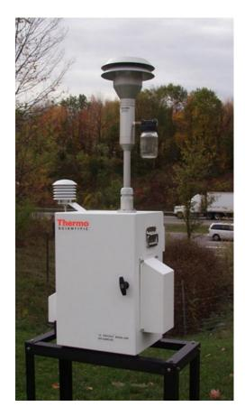
Figure 2.17. Dichotomous Air Sampler (ThermoScientific, 2015)
