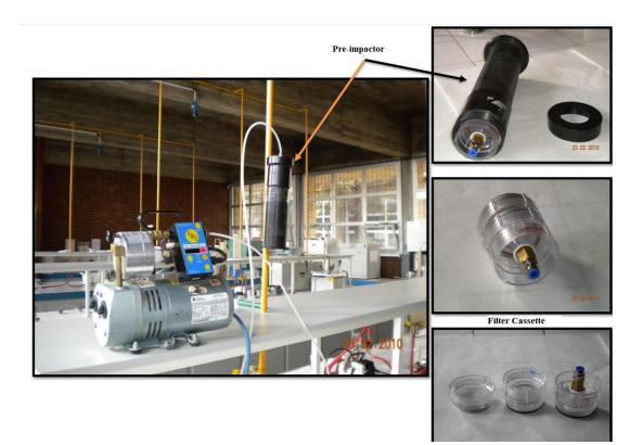
Figure 2.20. Stack Filter Unit (SFU) sampling system
