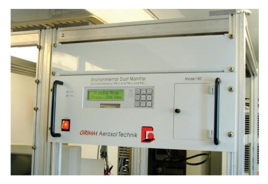
Figure 2.18. Grimm EDM180 Laser Aerosol Spectrometer
