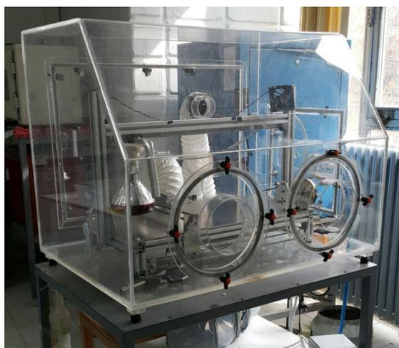
Figure 3.3 Air conditioning glove box
