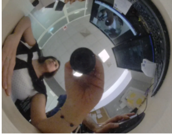
Figure 16: An example for the distortion on omnidirectional images.
