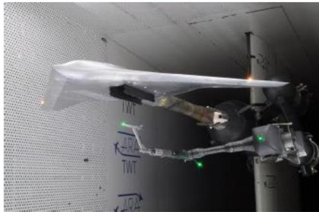
Figure 5.10. Parent and store models installed in the TWT working section on the TSR during the March 2012 tunnel entry [23]
