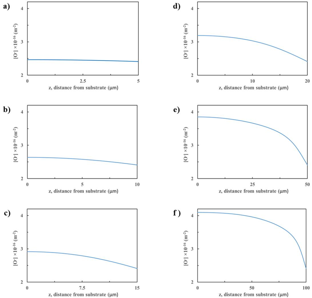
*Figure 4-15. Steady state concentration distribution of ionized oxygen in SnO<sub>2</sub> films have thicknesses of: a) 5  $\mu\text{m}$ ; b) 10  $\mu\text{m}$ ; c) 15  $\mu\text{m}$ ; d) 20  $\mu\text{m}$ ; e) 50  $\mu\text{m}$ ; f) 100  $\mu\text{m}$ . SnO<sub>2</sub> sensing films were exposed to 0.00814 mol/m<sup>3</sup> CO in an excess oxygen environment at 300 °C. ( $x=500\mu\text{m}$ )*
