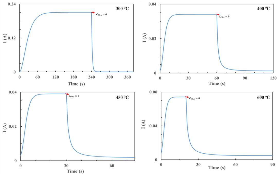
Figure 4-22. The effect of the temperature on the response/recovery dynamics for  $10 \mu\text{m}$  thick  $\text{SnO}_2$  film initially exposed to CO concentration of  $0.00814 \text{ mol/m}^3$  in an excess oxygen ambient.
