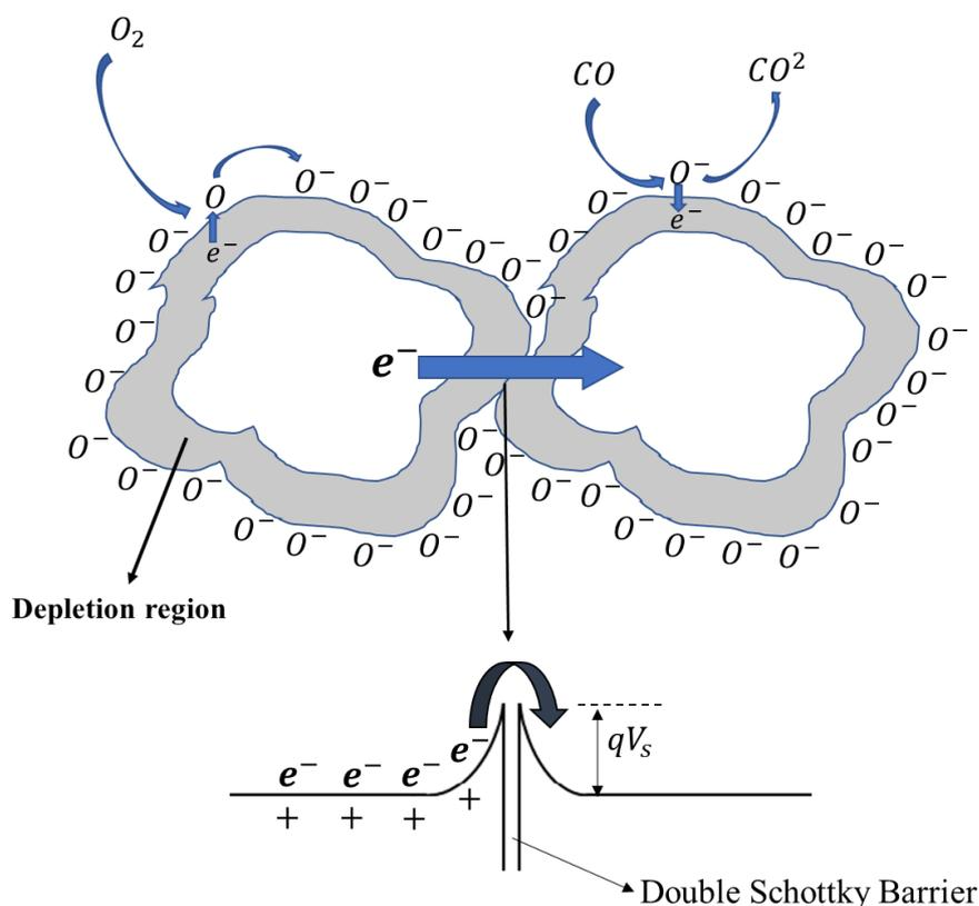
Figure 2-1. Schematic representation of the potential barrier developed at grain boundary of two adjacent grains in a polycrystalline metal oxide semiconductor.
