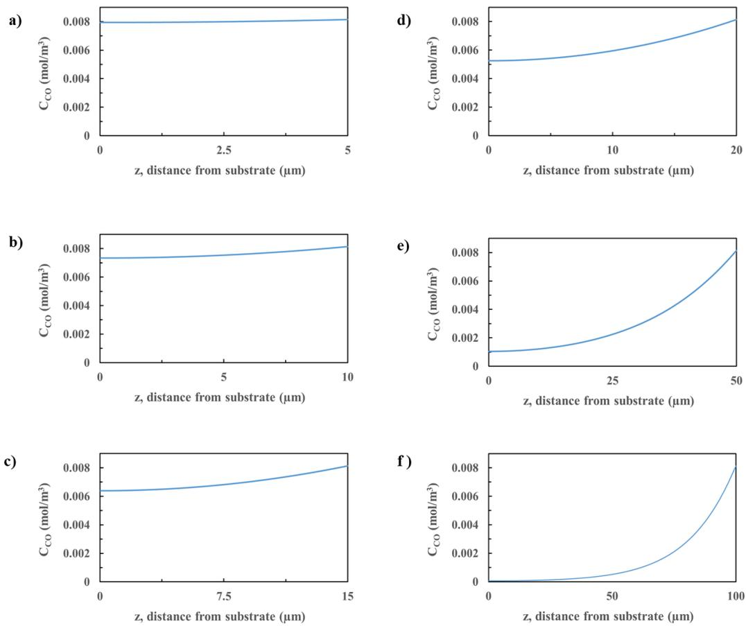
Figure 4-14. Steady state concentration distributions of CO in SnO<sub>2</sub> films have thicknesses of: a) 5 μm; b) 10 μm; c) 15 μm; d) 20 μm; e) 50 μm f) 100 μm. The results were obtained for a step change of 0.00814 mol/m<sup>3</sup> in CO concentration at  $t=0$  and at  $T=300$  °C
