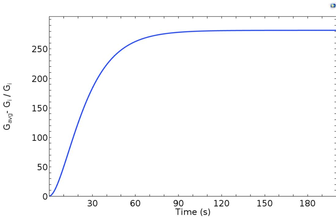
*Figure 4-5. The normalized response of the 15  $\mu\text{m}$  thick  $\text{SnO}_2$  film during exposure of carbon monoxide an excess oxygen ambient at  $T= 300\text{ }^\circ\text{C}$ . Step change in CO concentration of  $0.00814\text{ mol/m}^3$  at  $t=0$ . ( $x=500\text{ }\mu\text{m}$ )*
