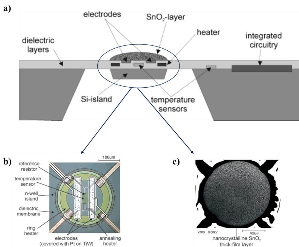
*Figure 1-2. The schematic of SnO<sub>2</sub> based gas sensor fabricated with CMOS technology on a micro hotplate: a) Side view schematics of the gas sensor; b) Top view of the microhotplate with circular heated area on the dielectric membrane; c) SEM image of the SnO<sub>2</sub> thick film.<sup>33</sup>*
