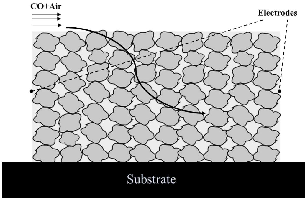
*Figure 3-1. Simple representation of the polycrystalline metal oxide semiconductor gas sensor exposing to carbon monoxide in air ambient.*
