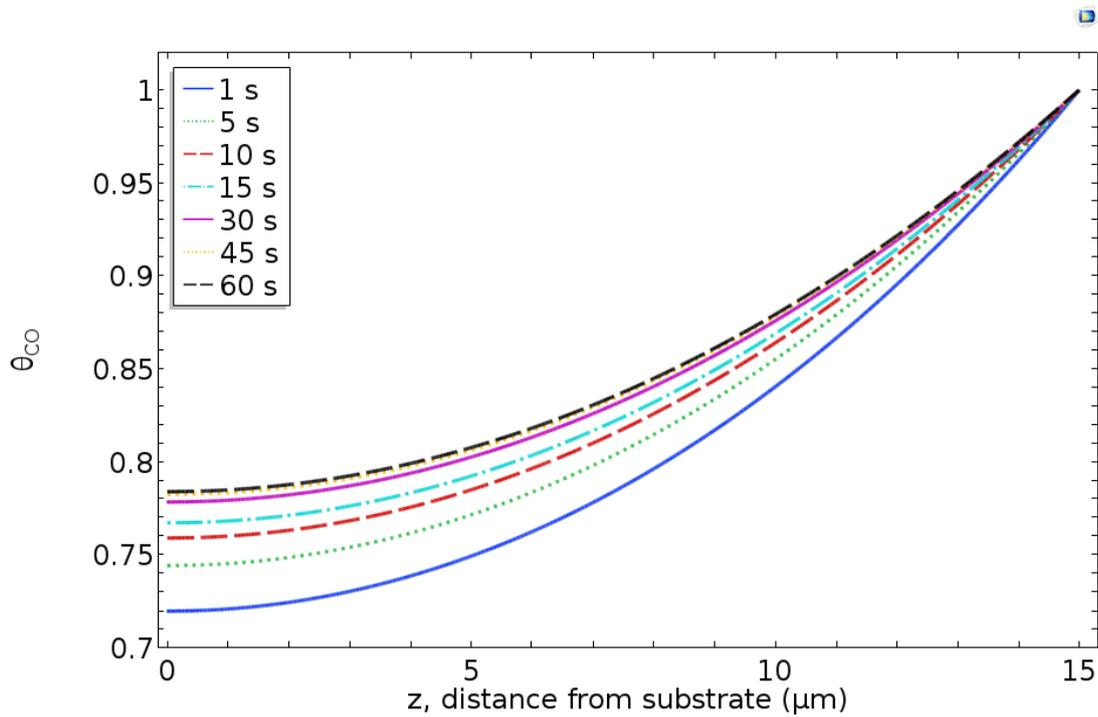
Figure 4-1. Transient analysis of the CO concentration profile development in 15 $\mu\text{m}$  thick film at  $T=300^\circ\text{C}$ . Response to the step change of CO concentration of 0.00814 mol/m<sup>3</sup> in an excess oxygen environment at  $t=0$ .
