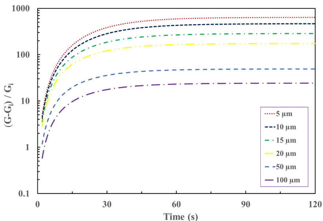
Figure 4-19. Effect of film thickness on the normalized response  $(G - G_i)/G_i$  of  $\text{SnO}_2$  sensing films for a step change of  $0.00814 \text{ mol/m}^3$  in CO concentration in an excess oxygen environment at  $t=0$ . ( $x=500 \mu\text{m}$ )
