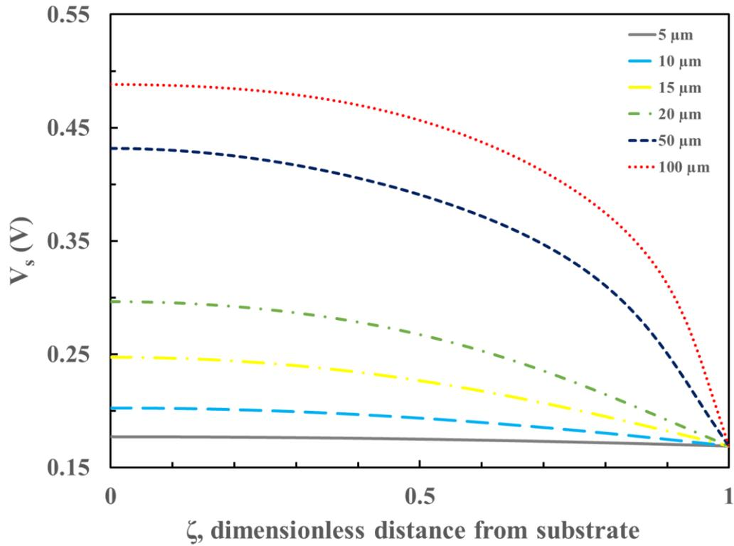
Figure 4-16. The effect of film thickness on the steady state potential energy barrier distribution for the  $\text{SnO}_2$  films at  $300\text{ }^\circ\text{C}$  exposed to  $0.00814\text{ mol/m}^3$  CO in an excess oxygen environment. ( $x=500\mu\text{m}$ )
