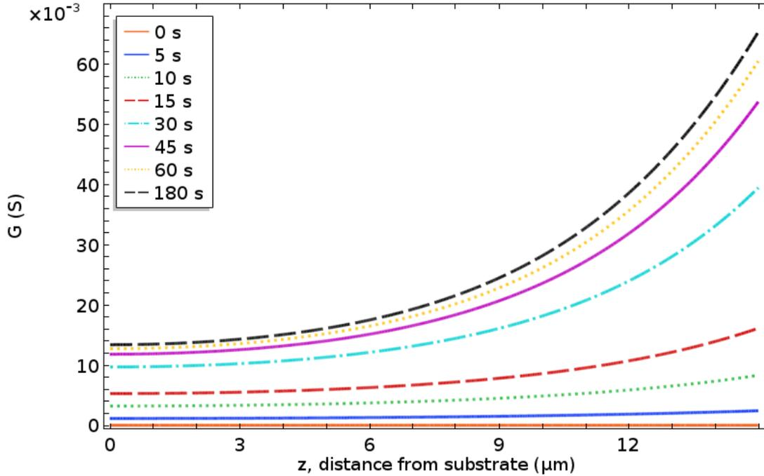
Figure 4-3. The change in the local conductance ( $G$ ) with time and its variation along the  $z$  (thickness) direction in  $15\mu\text{m}$   $\text{SnO}_2$  sensing film at  $T=300\text{ }^\circ\text{C}$ . Response to the step change of  $\text{CO}$  concentration of  $0.00814\text{ mol/m}^3$  at  $t=0$  in an excess oxygen ambient. ( $G_i = 9.31 \times 10^{-5}$ )
