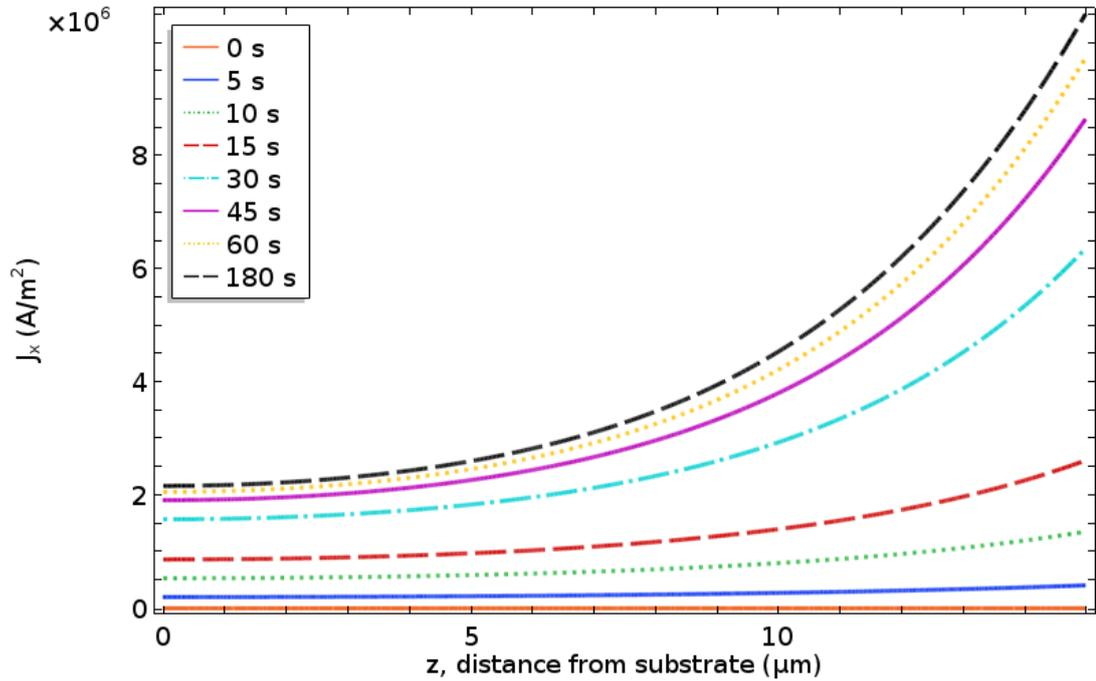
Figure 4-4. The x-component of the current density ( $J_x$ ) profile development in  $15\mu\text{m}$  thick  $\text{SnO}_2$  film at  $T=300^\circ\text{C}$ . Response to the step change of CO concentration of  $0.00814\text{ mol/m}^3$  in an excess oxygen ambient at  $t=0$ . ( $x = 500\mu\text{m}$ )
