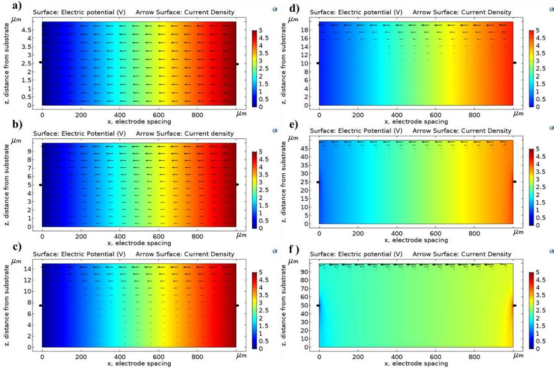
Figure 4-17. Steady state potential energy distributions and arrow representation of the current density for SnO<sub>2</sub> films having thicknesses of: a) 5 μm; b) 10 μm; c) 15 μm; d) 20 μm; e) 50 μm; f) 100 μm. The SnO<sub>2</sub> films were exposed to CO concentration of 0.00814 mol/m<sup>3</sup> in an excess oxygen environment at 300 °C. 5 V DC electric potential was applied with point electrodes from both sides of the sensing film with DC supplier.
