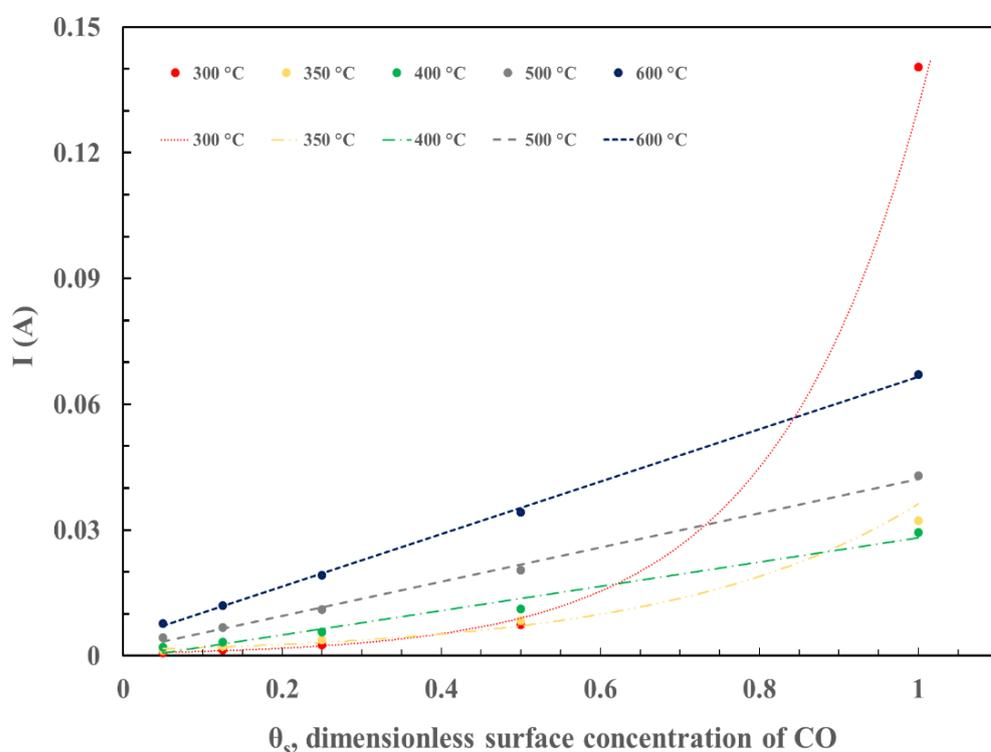
*Figure 4-24. The effect of the ambient concentration of carbon monoxide on the steady state electric current response of 10  $\mu\text{m}$  thick  $\text{SnO}_2$  gas sensor having pores with 1 nm diameter in an excess oxygen environment.*
