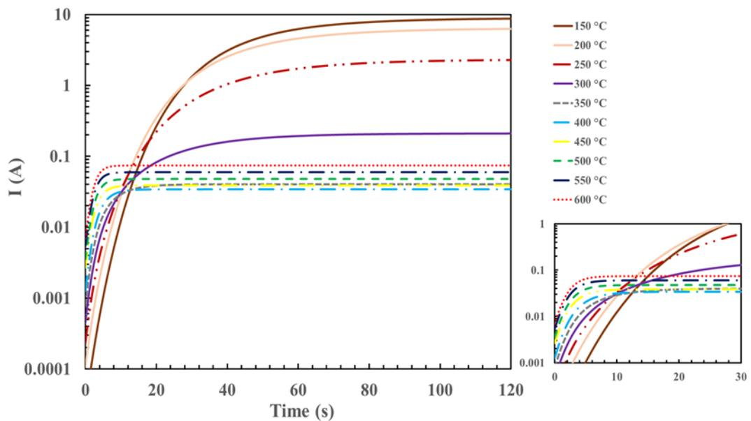
*Figure 4-12. Effect of temperature on the transient response of the 10 μm SnO<sub>2</sub> sensing film to step change in CO concentration of 0.00814 mol/m<sup>3</sup> in terms of electrical current. (x=500 μm)*
