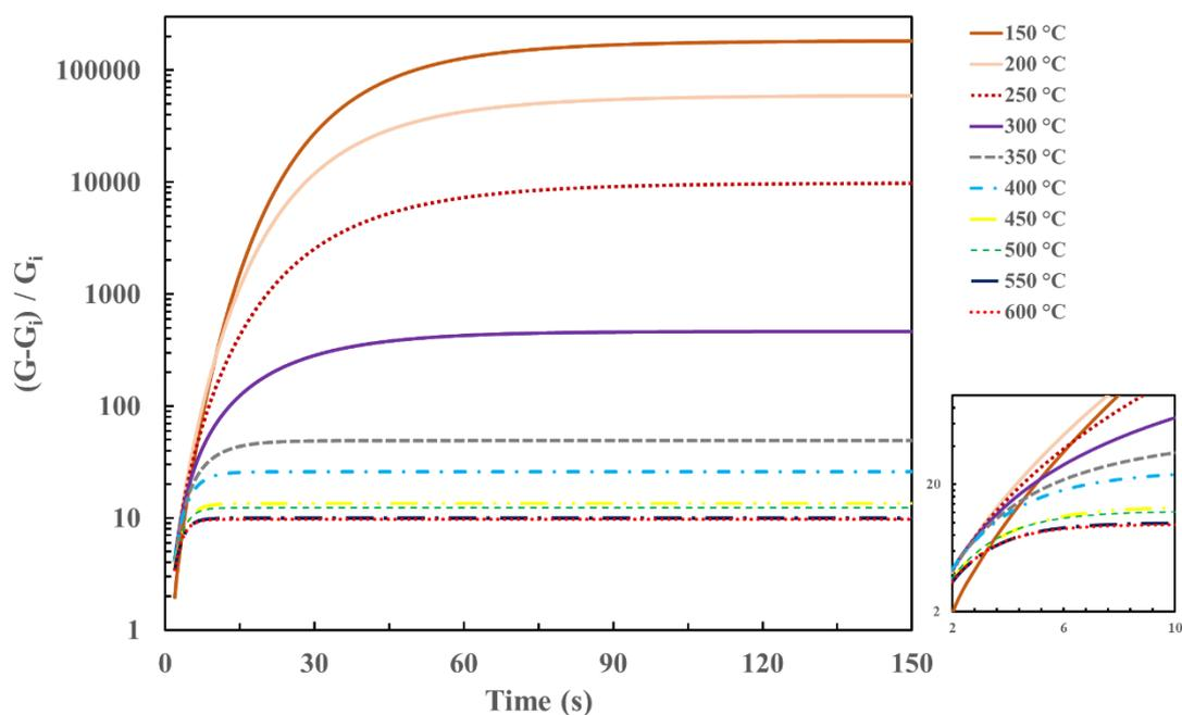
*Figure 4-13. Effect of temperature on the transient normalized response of the 10  $\mu\text{m}$   $\text{SnO}_2$  sensing film to the step change of CO concentration of  $0.00814 \text{ mol/m}^3$  in an excess oxygen ambient at  $t=0$ . ( $r=1 \text{ nm}$ ).*
