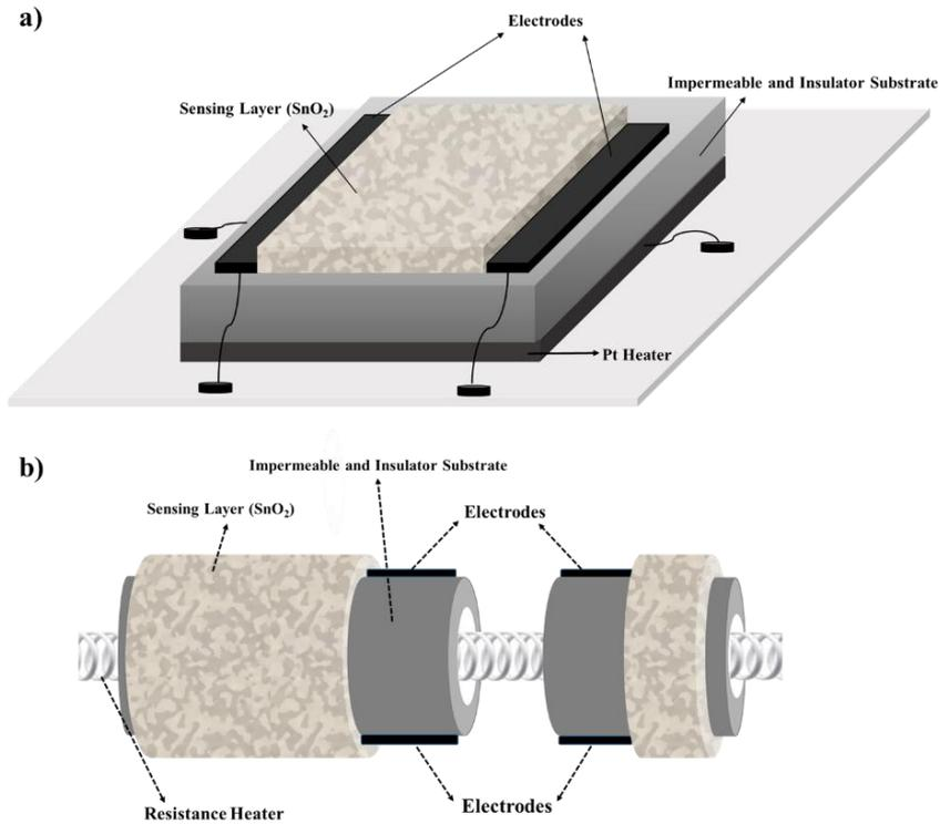
*Figure 1-1. Schematic representation of classical Taguchi-typed gas sensors: a) Planar configuration; b) Cylindrical configuration.*
