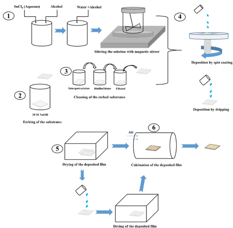
*Figure 2-2. Synthesis of thin/thick film SnO<sub>2</sub> by sol-gel method and deposition on substrates.*
