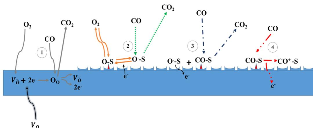
Figure 2-3. Kinetic mechanisms for the CO interaction with SnO<sub>2</sub>: 1) Oxygen vacancy mechanism; 2) Eley-Rideal mechanism; 3) Langmuir-Hinshelwood mechanism; 4) Ionization of CO in the absence of oxygen or low oxygen pressure ambient.
