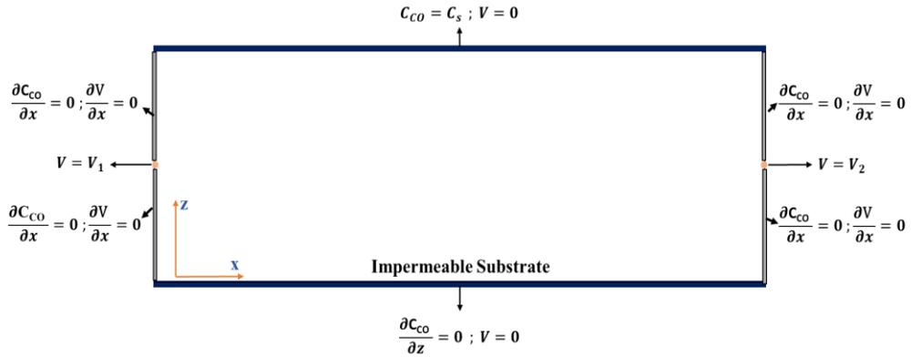
*Figure 3-2. The representation of the rectangular geometry used in the model with the boundary conditions.*
