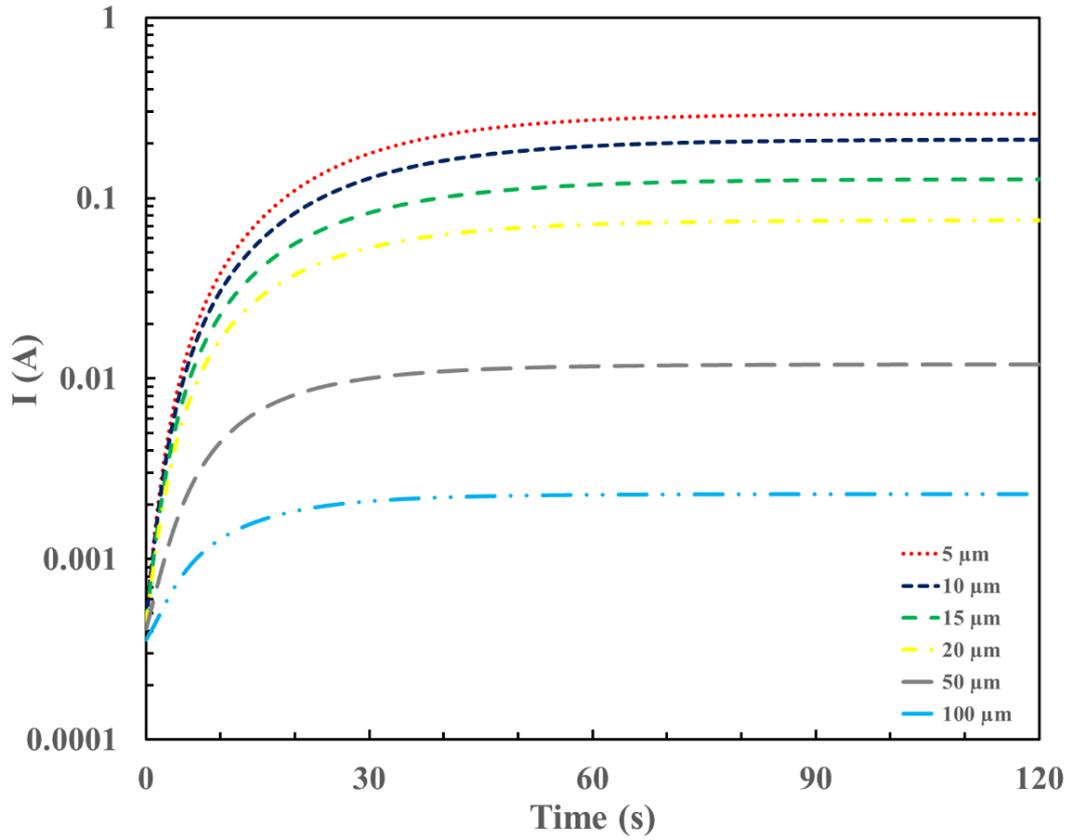
Figure 4-18. The effect of film thickness on the dynamic current response to the step change in CO concentration of  $0.00814 \text{ mol/m}^3$  in an excess oxygen ambient at  $300^\circ\text{C}$ . 5 V DC electric potential applied through point electrodes at both sides of the  $\text{SnO}_2$  sensing films. ( $x = 500 \mu\text{m}$ ).
