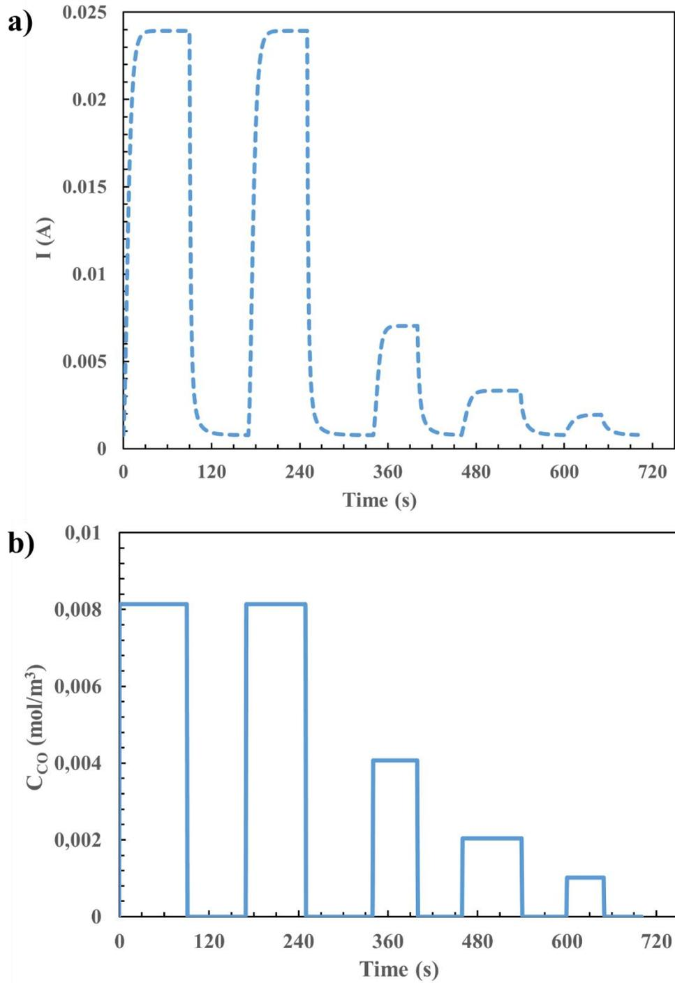
Figure 4-21. Response/recovery analysis of 10µm thick SnO<sub>2</sub> films having 1 nm pore diameter to step changes of carbon monoxide concentration in an excess oxygen ambient at 350 °C.
