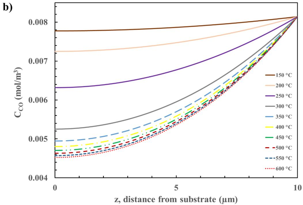
Figure 4-8. The steady state CO concentration distributions in the 10  $\mu\text{m}$   $\text{SnO}_2$  film at temperatures between 150-600 °C for pore diameters :a)4nm; b)1nm.
