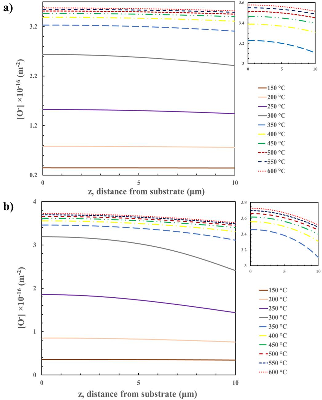
Figure 4-9. The steady state ionized oxygen concentration distributions in the  $10 \mu\text{m}$   $\text{SnO}_2$  film at different temperatures for pore diameters: a) 4 nm; b) 1 nm.
