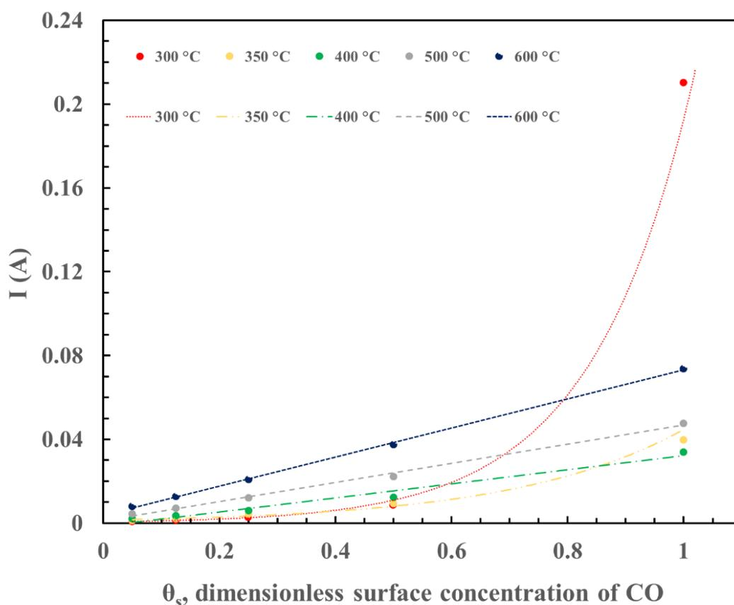
Figure 4-23. The effect of the ambient concentration of carbon monoxide on the steady state electric current response of 10  $\mu\text{m}$  thick  $\text{SnO}_2$  gas sensor having pores with 4 nm diameter in an excess oxygen environment.
