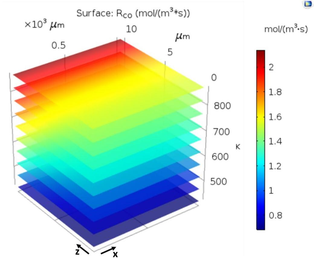
Figure 4-11. Two dimensional representation of the steady state consumption rates of CO at operating temperatures between 423-873K. Results were obtained for a step change of CO concentration of  $0.00814 \text{ mol/m}^3$  in an excess oxygen ambient at  $t=0$ .
