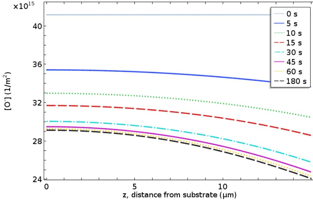
Figure 4-2. Transient analysis of the ionized oxygen density  $[O]$  in  $15 \mu\text{m}$  thick  $\text{SnO}_2$  film at  $T = 300^\circ\text{C}$ . Response to the step change of  $\text{CO}$  concentration of  $0.00814 \text{ mol/m}^3$  at  $t=0$ .
