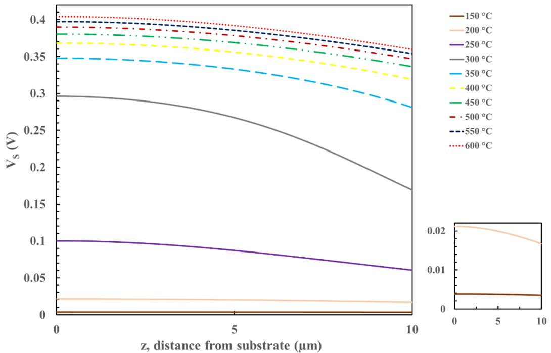
*Figure 4-10. Temperature effect on the steady state potential barrier profiles for 10 μm thick SnO<sub>2</sub> film which has pore diameter of 1nm.*
