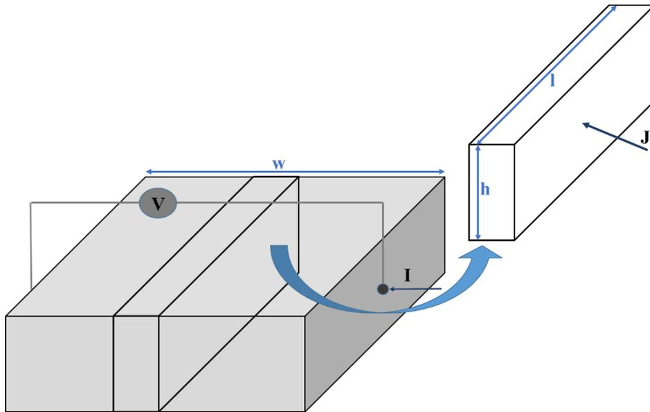
*Figure 3-4. The schematic representation of the cross-sectional area perpendicular to the current direction on a cut plane from the three dimensional representation of the gas sensor.*
