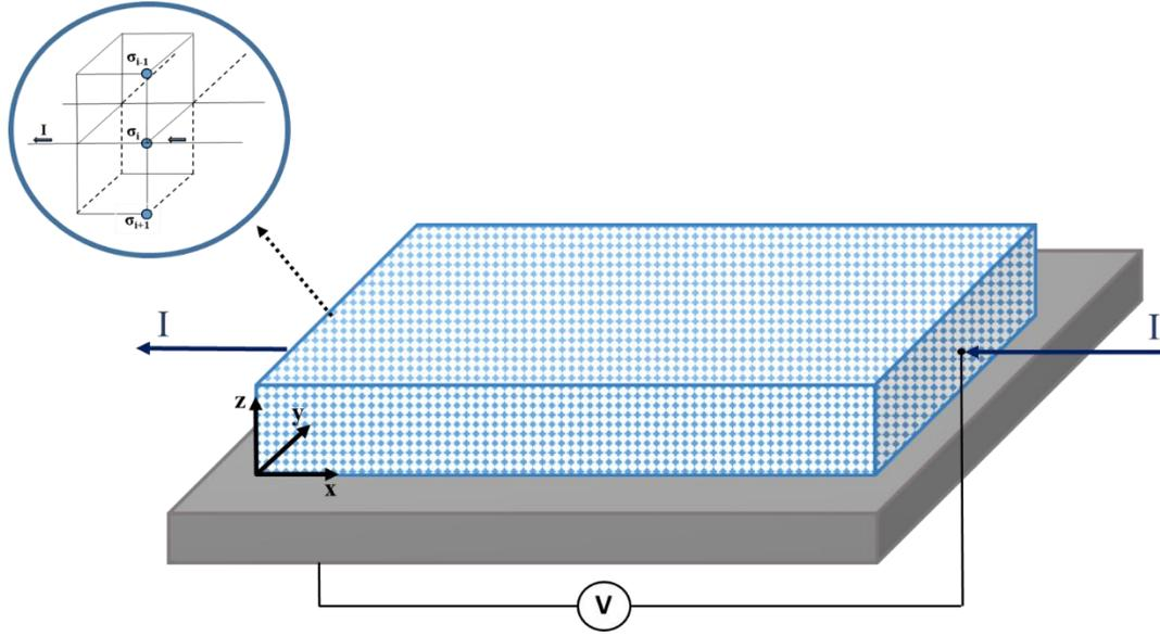
Figure 3-3. Three dimensional representation of the gas sensor device.
