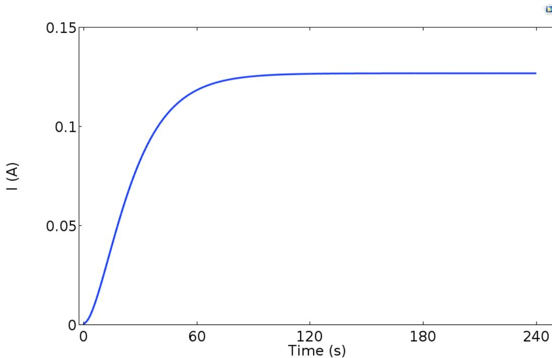
*Figure 4-6. Electric current signal response of the 15  $\mu\text{m}$  thick  $\text{SnO}_2$  sensing film to carbon monoxide in excess oxygen ambient at  $T= 300\text{ }^\circ\text{C}$ . Response to the step change of CO concentration of  $0.00814\text{ mol/m}^3$  at  $t=0$ .*
