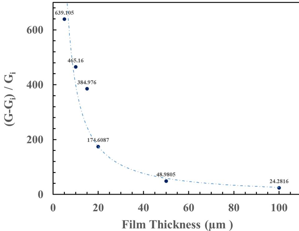
Figure 4-20. Steady state normalized responses of the SnO<sub>2</sub> films having different thicknesses to exposing CO continuously in an excess oxygen ambient.
