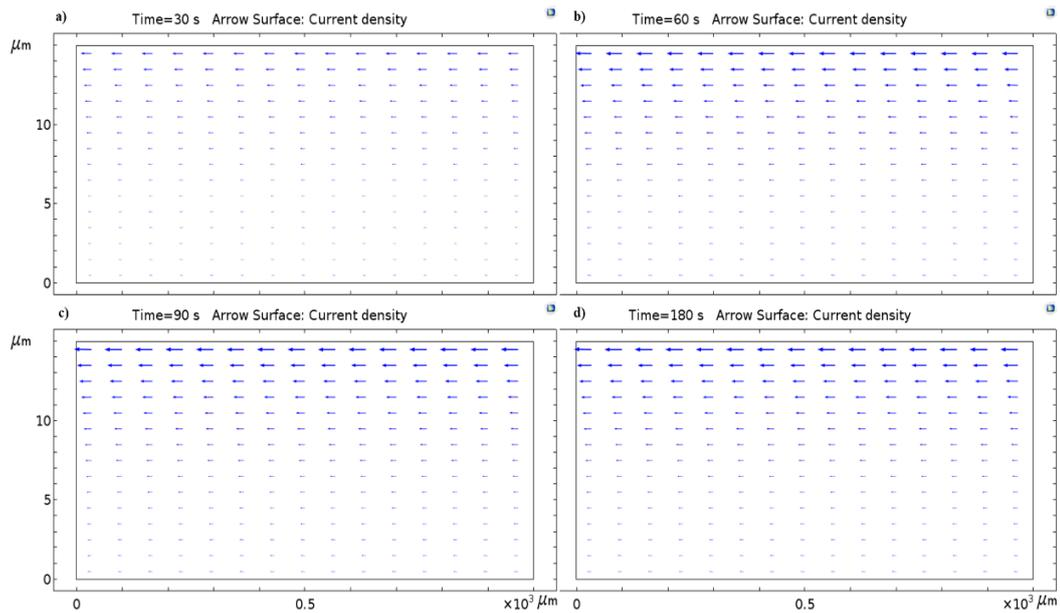
*Figure 4-7. The arrow representation of the current density for 15  $\mu\text{m}$  thick  $\text{SnO}_2$  film response to the step change of CO concentration of  $0.00814 \text{ mol/m}^3$  in an excess oxygen ambient at times: a)  $t=30 \text{ s}$ ; b)  $60 \text{ s}$ ; c)  $90 \text{ s}$ ; d)  $120 \text{ s}$ . Note that the scales for the arrows are same. ( $T=300 \text{ }^\circ\text{C}$ )*
