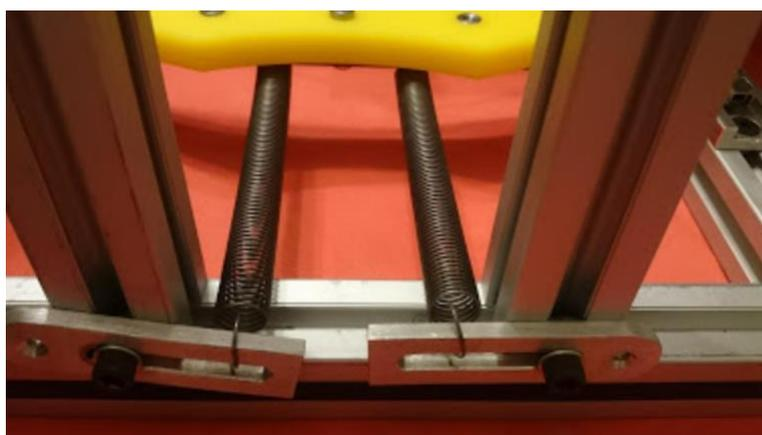
Figure 5.17. MFG spring endpoints on the ground link side
