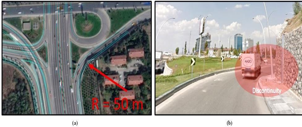
Figure 6.28. Plan View of the South-East Leg on Inonu Blvd. Interchange (a) and Discontinuity on the Ramp (b)
