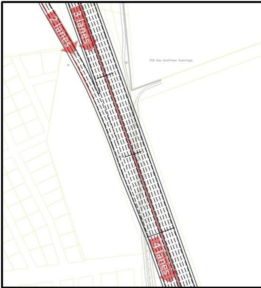
Figure 6.52. Lane Balance Situation at the Entrance Terminal of South-West Quadrant Ramp of METU Interchange and 1071 Malazgirt Boulevard
