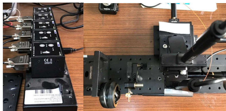
Figure 4.4. T-Cube DC Servo Controllers (left) and Z825B Motorized Actuators (right)
