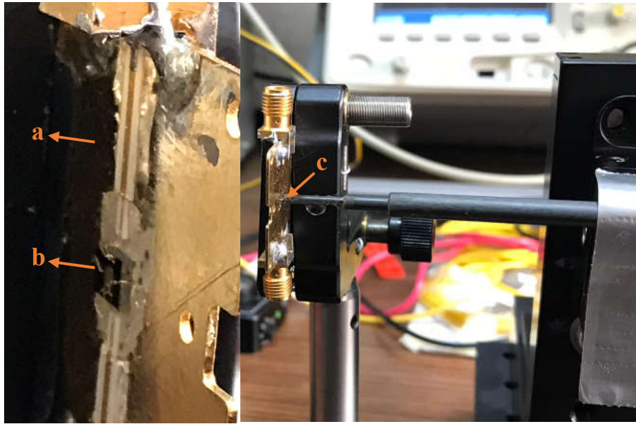
Figure 4.11. The MEMS microphone coupled to the chip carrier(left) and the cleaved fiber tip mounted on the XYZ stage(right)
