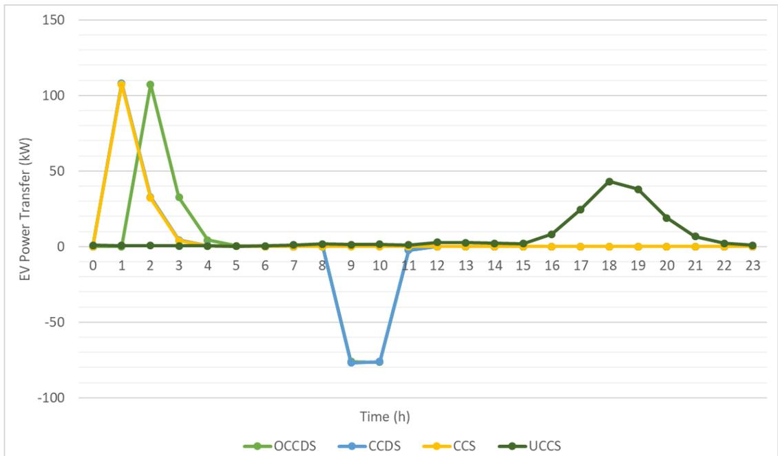
Figure 45. The Power Transfer Between the Microgrid and EVs for Case II in February
