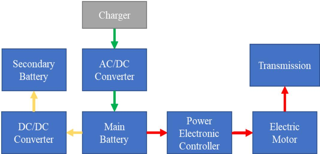
Figure 1. Working Principle Diagram of BEVs
