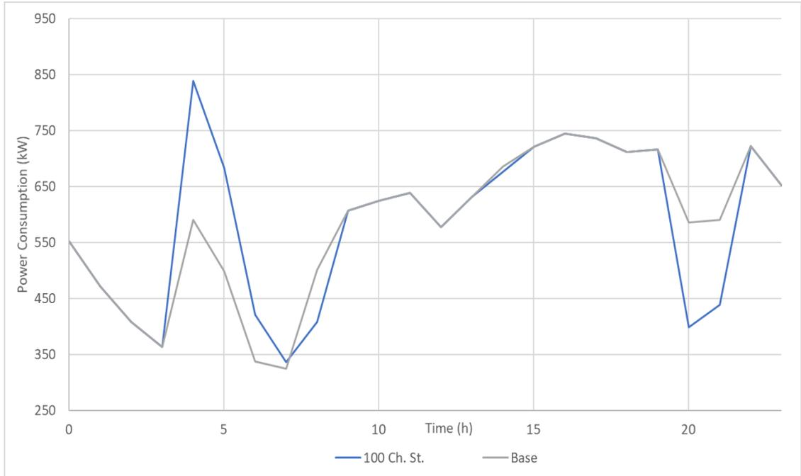
Figure 42. The Power Curve of the Microgrid with Different Number of Charging Stations for Case II
