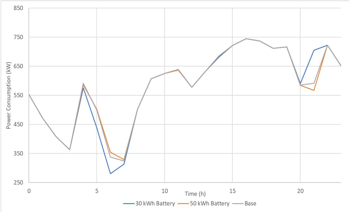
Figure 36. The Power Curve of the Microgrid with Different Battery Capacity for Case II
