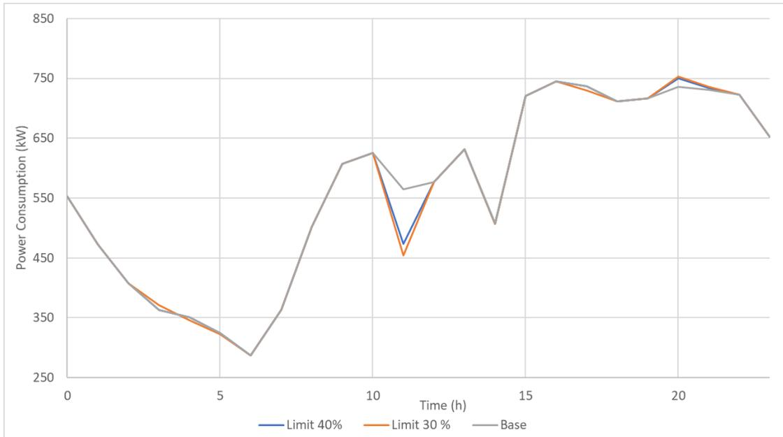
Figure 23. The Power Curve of the Microgrid with Different MSoCL for Case I
