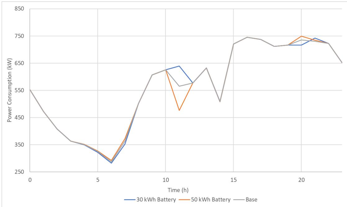
Figure 22. The Power Curve of the Microgrid with Different Battery Capacity for Case I
