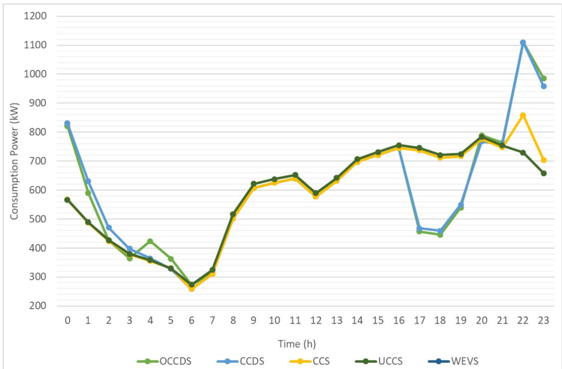
Figure 51. The Daily Power Curve of the Microgrid for Case III with TOUT
