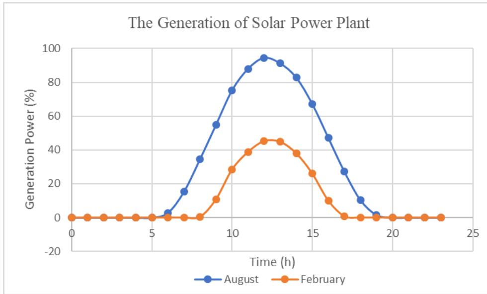
Figure 8 . The Electricity Generation of the Solar Power Plant
