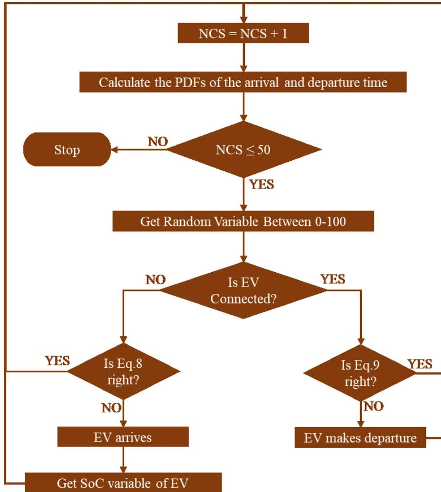
Figure 17. The Flow Chart of Generation of Probabilistic Variables About EVs
