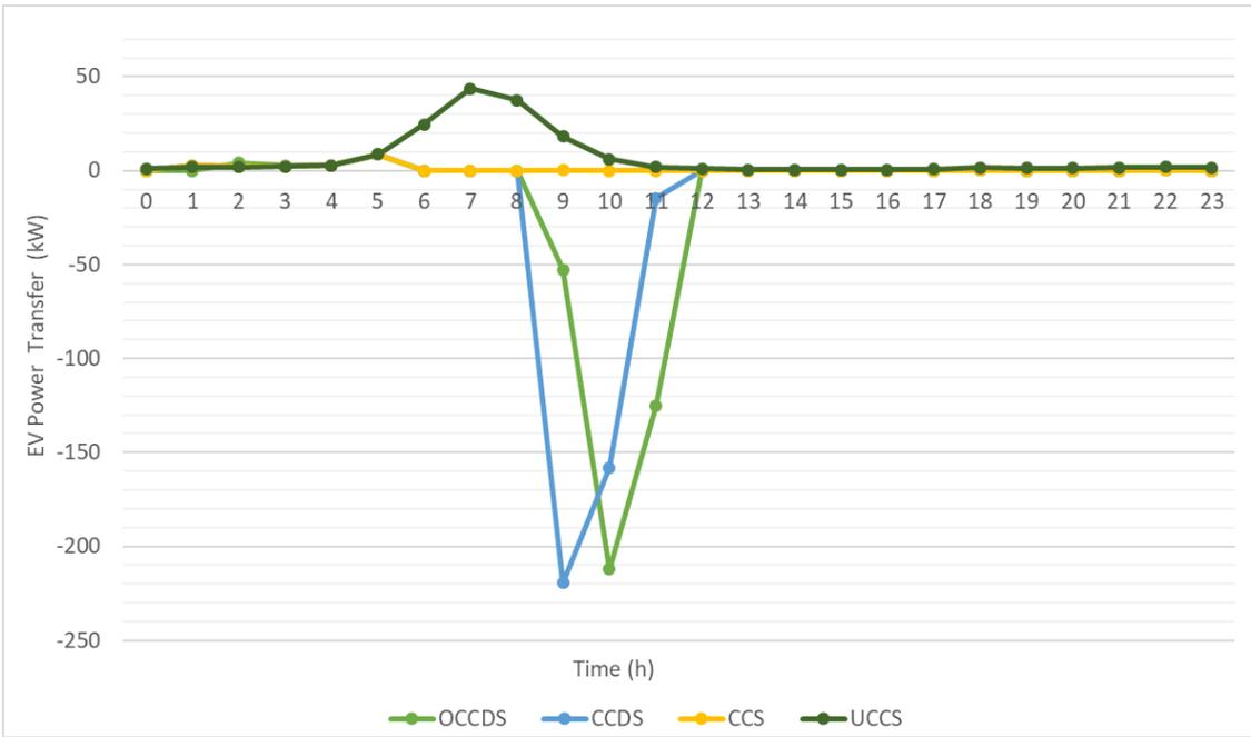
Figure 31. The Power Transfer Between the Microgrid and EVs for Case I in February
