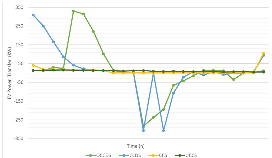
Figure 47. The Daily Power Transfer Between the Microgrid and EVs for Case III
