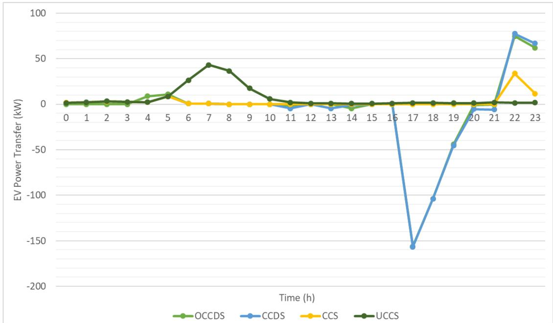
Figure 29. The Power Transfer Between the Microgrid and EVs for Case I with TOUT
