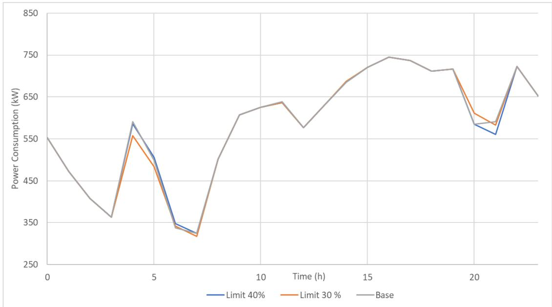
Figure 37. The Power Curve of the Microgrid with Different MSoCL for Case II
