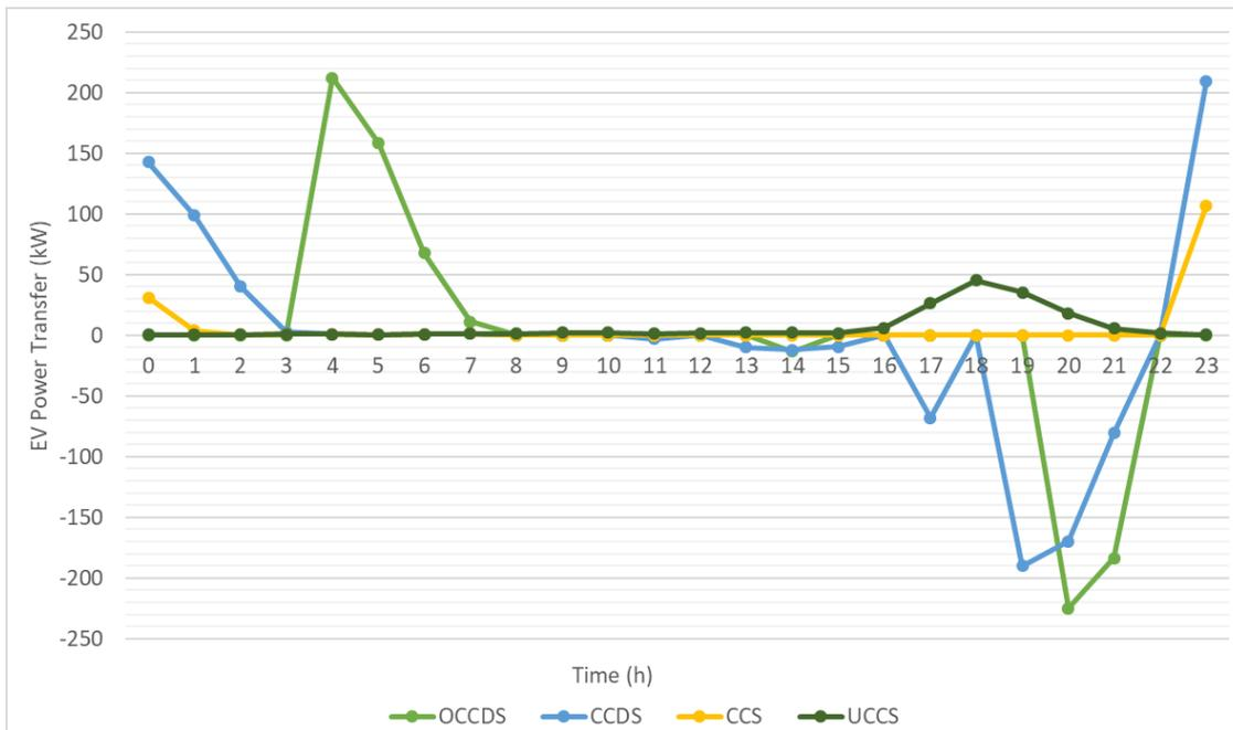
Figure 34. The Power Transfer Between the Microgrid and EVs for Case II
