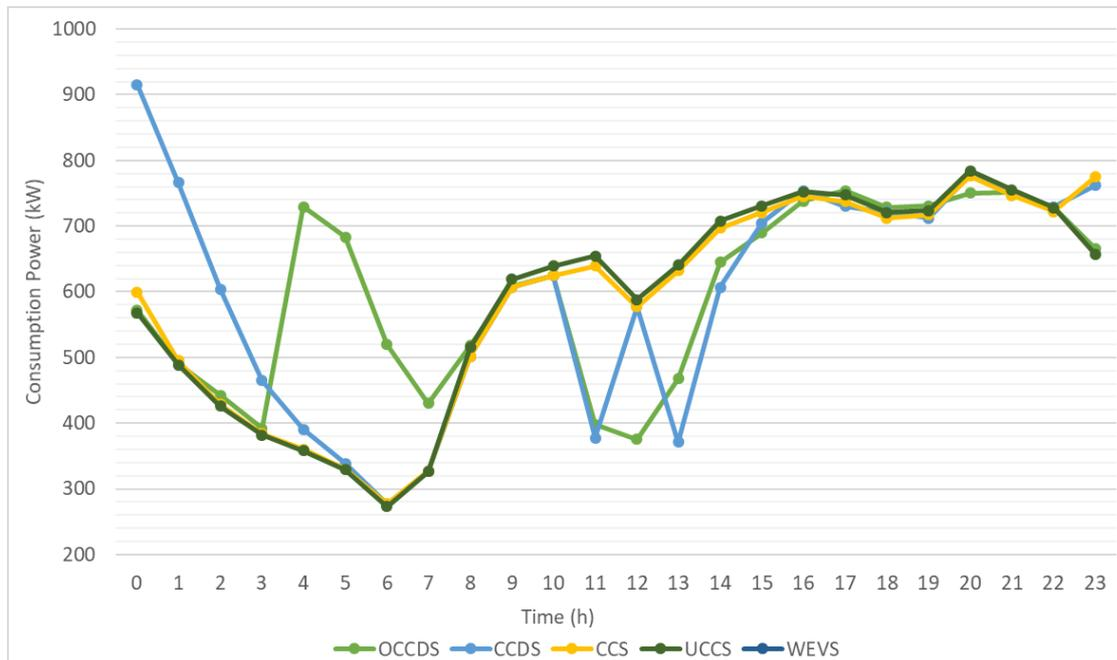
Figure 48. The Daily Power Curve of the Microgrid for Case III
