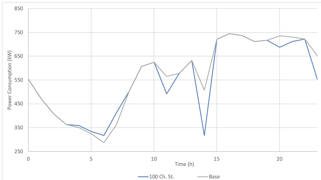
Figure 28. The Power Curve of the Microgrid with Different Number Charging Stations for Case I
