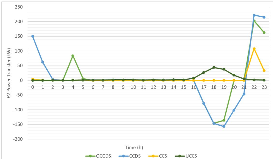
Figure 43. The Power Transfer Between the Microgrid and EVs for Case II with TOUT
