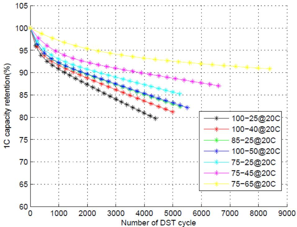
Figure 2. The Degradation of Li-ion Battery Respect to Charging Behavior [5]
