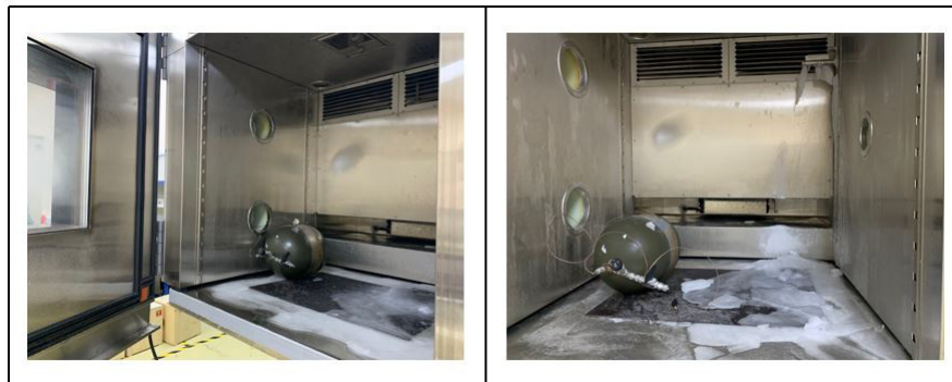
Figure 4.10: Propellant tank inside the conditioning cabin at the end of cooling process
