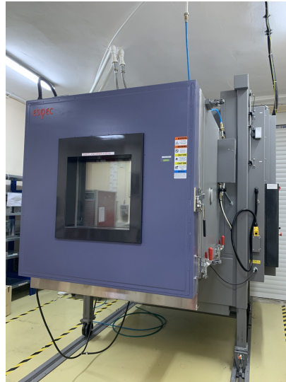
Figure 4.9: Conditioning cabin used for low temperature operational conditions experiments
