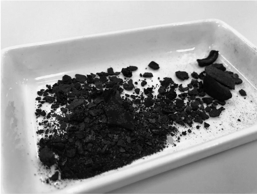
*Figure 3.3 Fuel gas soot (FG) sample gathered from the burner tips*
