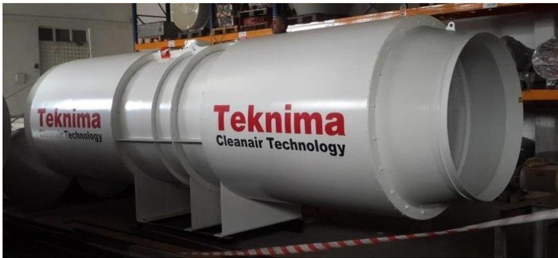
*Figure 5.6. Assembled Axial Flow Fan*
