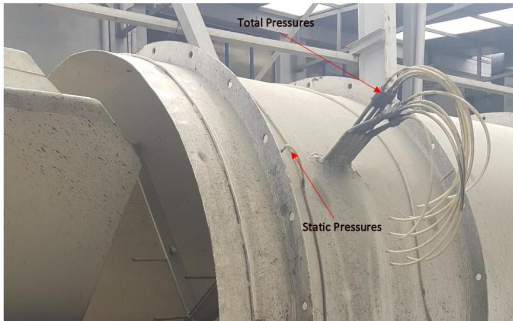
*Figure 5.10.* Pitot Tube Section of the Test Tube
