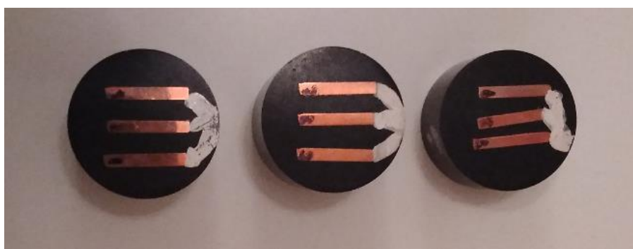
Figure 3.5. Prepared coupons for EDS line analysis
