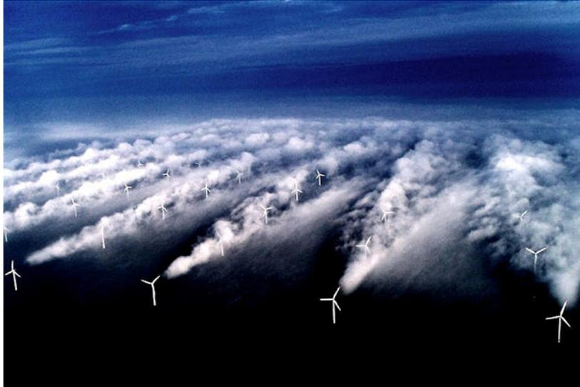
Figure 1.1: Wake interactions in Horns Rev Offshore Wind Farm, Denmark.
