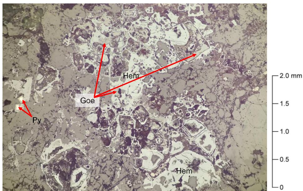
Figure 3.19 Pyrite (Py) grains completely replaced by hematite (Hem) and goethite (Goe; reflected plane-polarized light).
