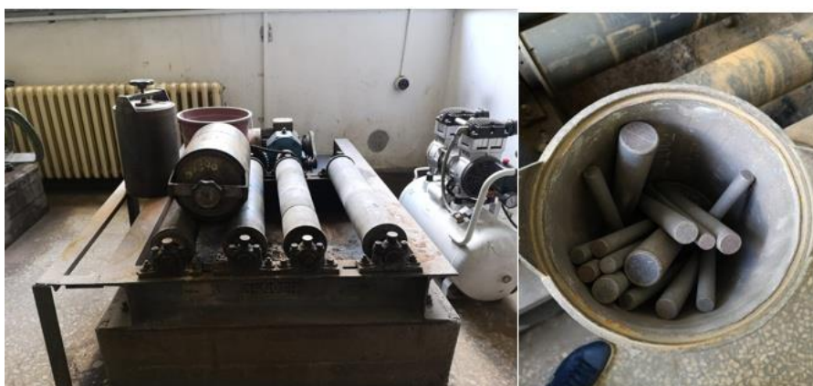
Figure 3.28 a) Representation of Rod Mill b) Representation of Grinding Media
