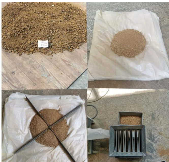
Figure 3.26 Representative Sample Preparation Procedure: a) Run of Mine Ore b) Crushed Ore Sample c) representative sampling by using cone and quartering method d) representative sampling by using Jones Riffle.
