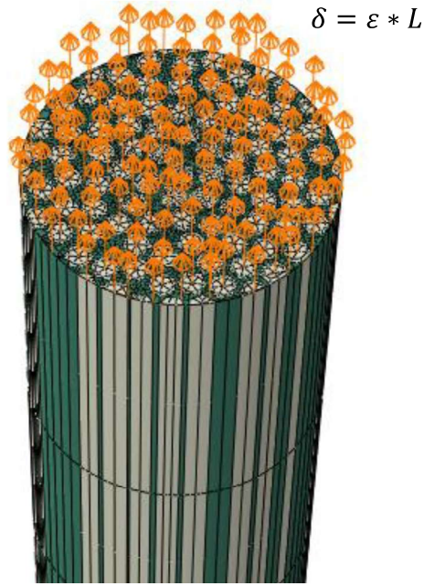
Figure 3.18. Top plane boundary conditions.
