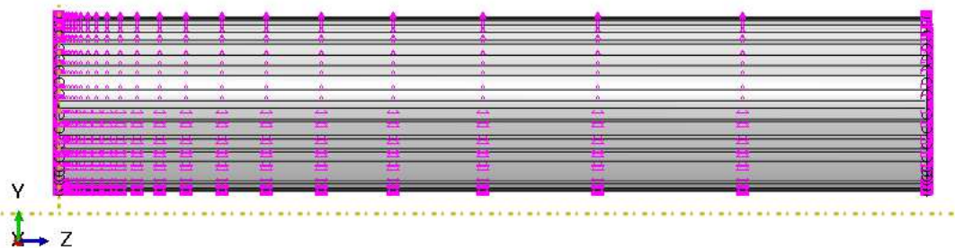
Figure 3.11. Seeding along fiber direction by using bias method.
