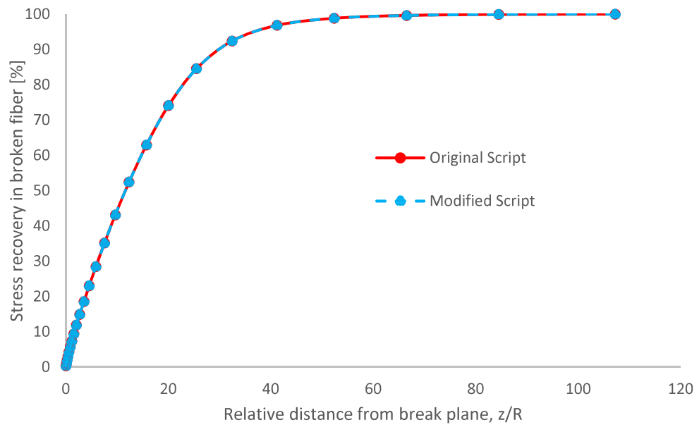
Figure 3.21. Stress recovery profiles of broken fibers for models of both original and modified scripts.
