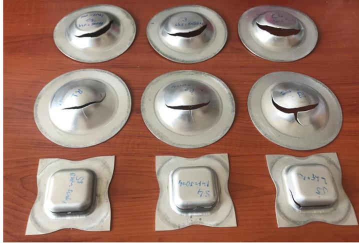
Figure 4.26. Deep drawing process specimens after completion of processes
