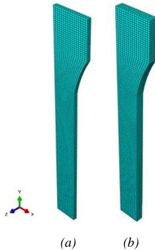
Figure 5.12. Mesh domain covering  $\frac{1}{4}$  of the specimen (a) Al2024T3 (b) S235JR
