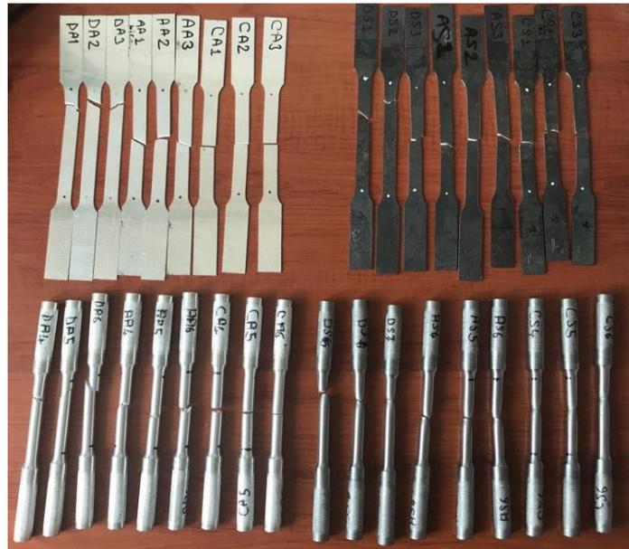
Figure 4.7. Flat and cylindrical specimens after the completion of the tests
