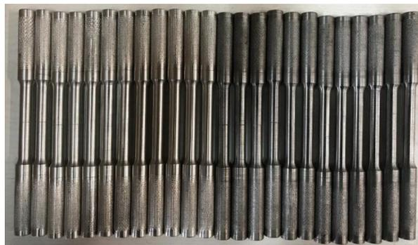
*Figure 4.5.* All the round specimens prepared for the test including the spares (12 on the left hand-side are Al and 12 on the righthand- side are steel)
