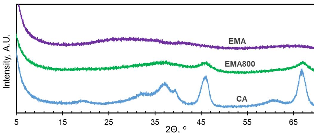
Figure 5.6. XRD patterns of alumina supports
