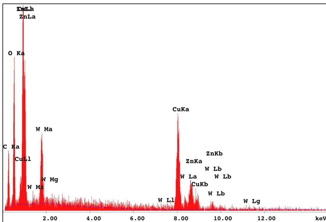
Figure 5.46. EDX spectrum of the TPA@Cu-Zn@CMK-3 catalyst
