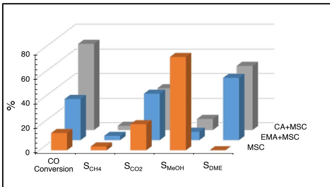
Figure 5.51. Effect of single-step DME synthesis on product selectivities over different catalysts (P: 50 bar, T: 275°C, H<sub>2</sub>/CO= 1/1, GHSV: 5000 ml/h.gcat)
