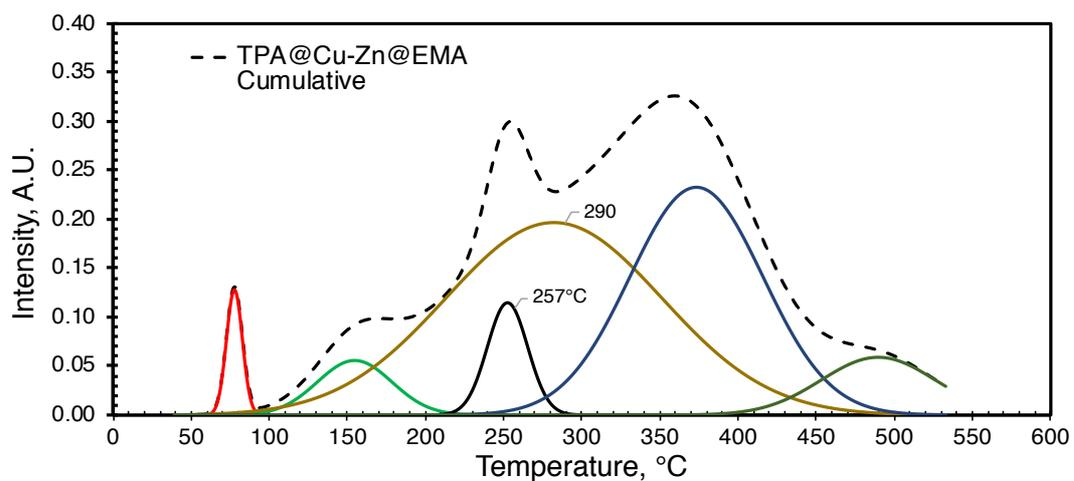
Figure 5.40. Deconvoluted TPD curve of TPA@Cu-Zn@EMA catalyst (dashed lines represents cumulative curves, solid lines represents deconvoluted peaks)
