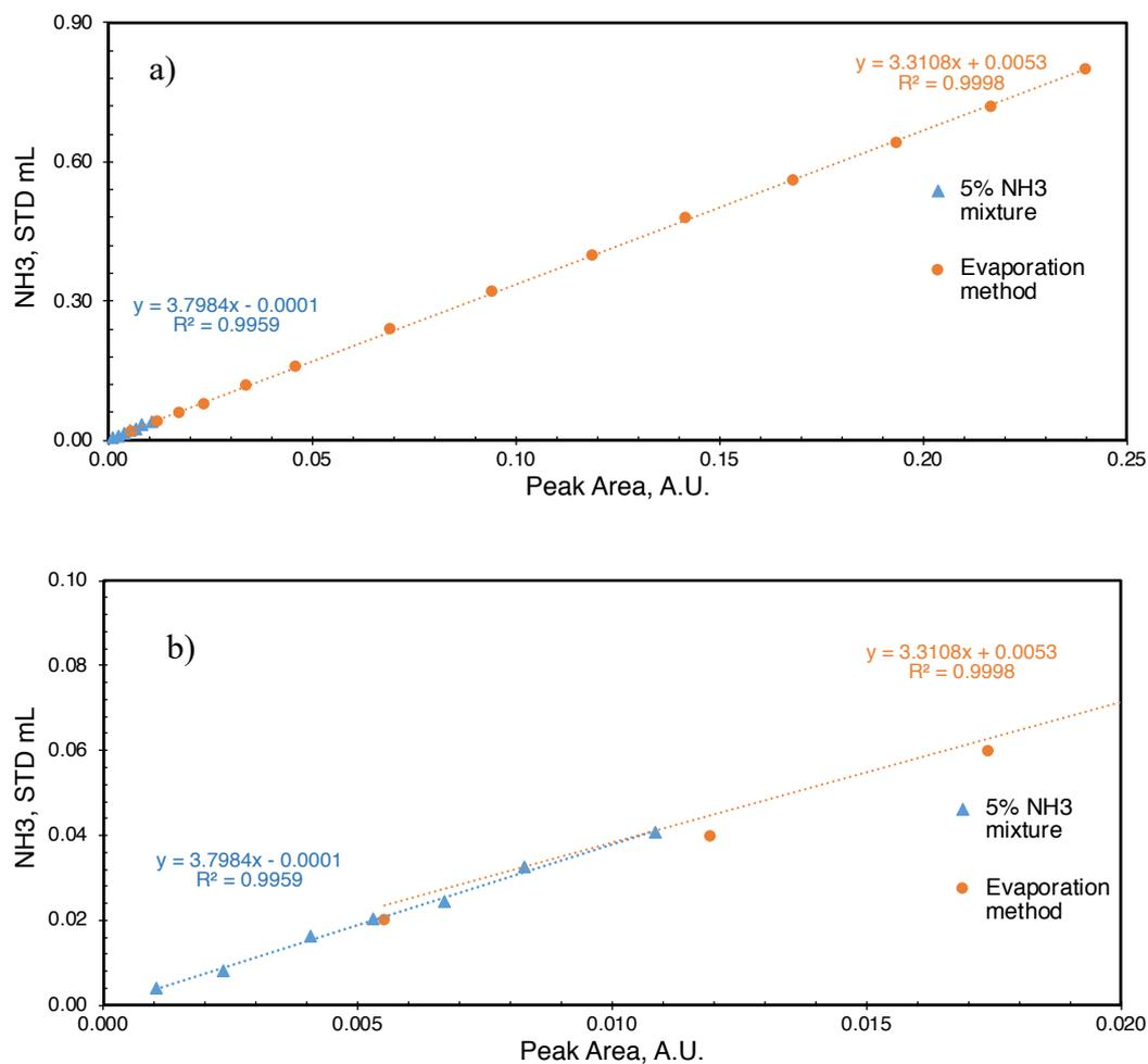
Figure B.1. a) NH<sub>3</sub>-TPD calibration curve b) magnified version of calibration curve
