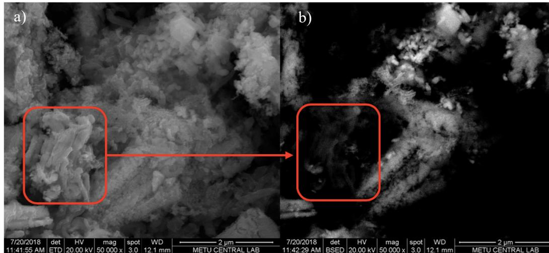
Figure 5.45. SEM (a) and backscattered electron (b) images of TPA@Cu-Zn@CMK-3 catalyst at 50,000 magnification
