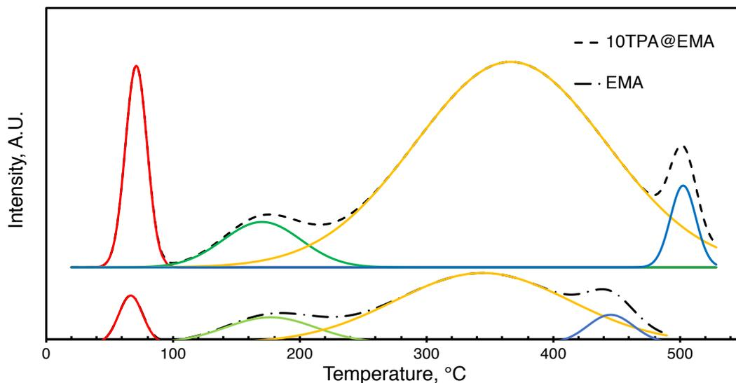
Figure 5.23. Deconvoluted TPD profiles of EMA support and 10TPA@EMA catalyst (dashed lines: original TPD curves, solid lines: deconvoluted peaks)
