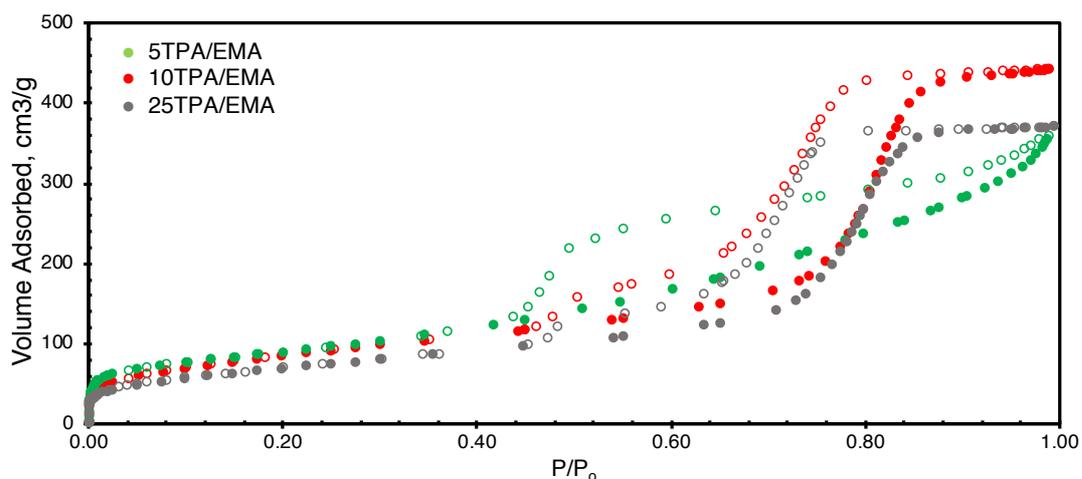
Figure 5.20. Nitrogen adsorption/desorption isotherms of TPA loaded EMA catalysts using one-pot method (filled symbols: adsorption and empty symbols: desorption branches).
