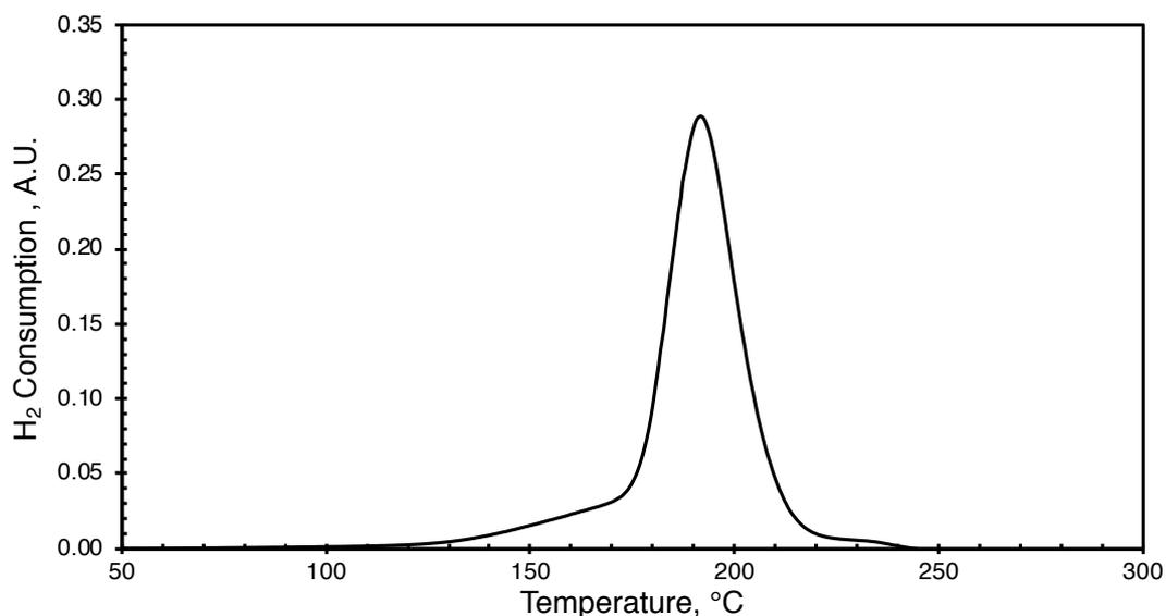
Figure 5.4. H<sub>2</sub>-TPR analysis of commercial methanol synthesis catalyst
