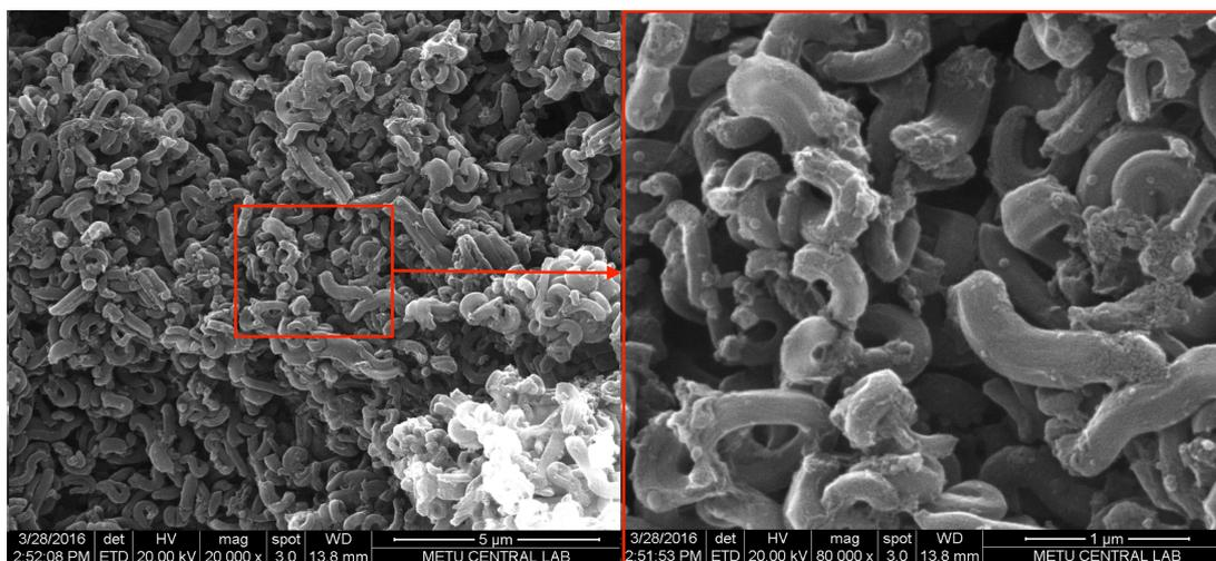
Figure 5.33. SEM images of CMK-3 catalyst at different magnifications: (a) 20,000 and (b) 80,000
