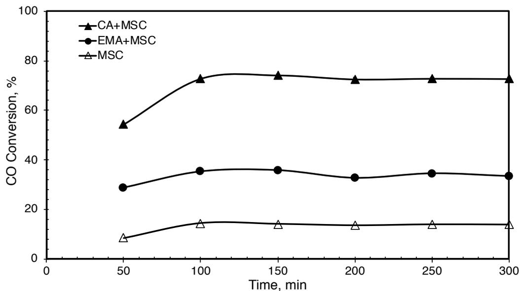
Figure 5.50. Effect of single-step DME synthesis on CO conversion over different catalysts (P: 50 bar, T: 275°C, H<sub>2</sub>/CO= 1/1, GHSV: 5000 ml/h.gcat).
