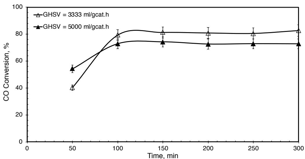
Figure 5.58. Effect of GHSV on CO conversion (P: 50 bar, T: 275°C, H<sub>2</sub>/CO= 1/1, Catalyst: MSC + CA (1/1 by wt.))
