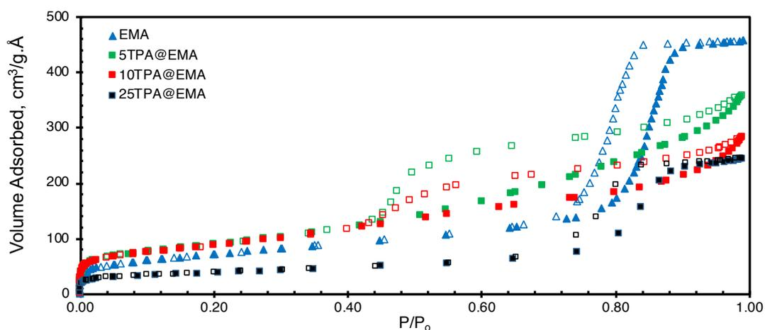
Figure 5.18. Nitrogen adsorption/desorption isotherms of EMA support and TPA impregnated EMA catalysts (filled symbols: adsorption and empty symbols: desorption branches).
