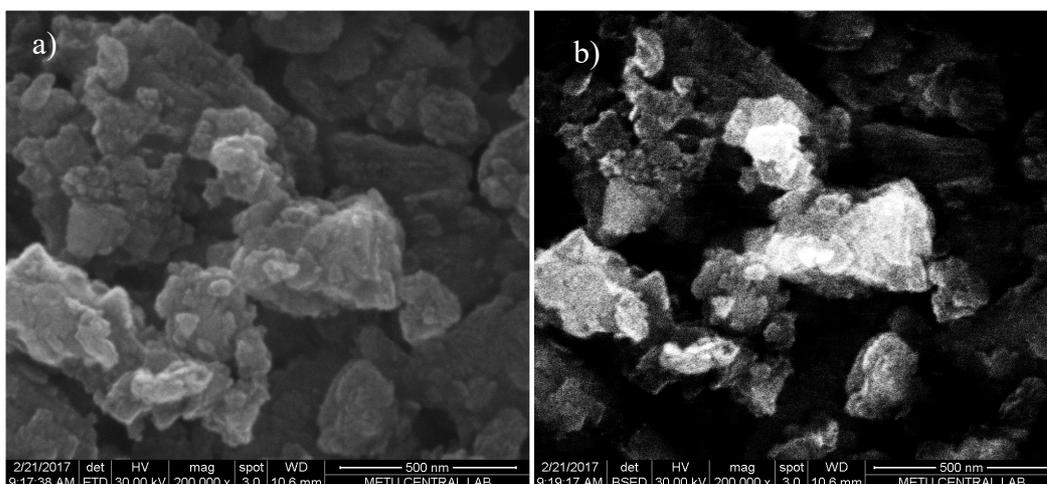
*Figure 5.27.* SEM (a) and backscattered electron (b) images of the 10TPA@EMA catalyst at 200,000 magnification
