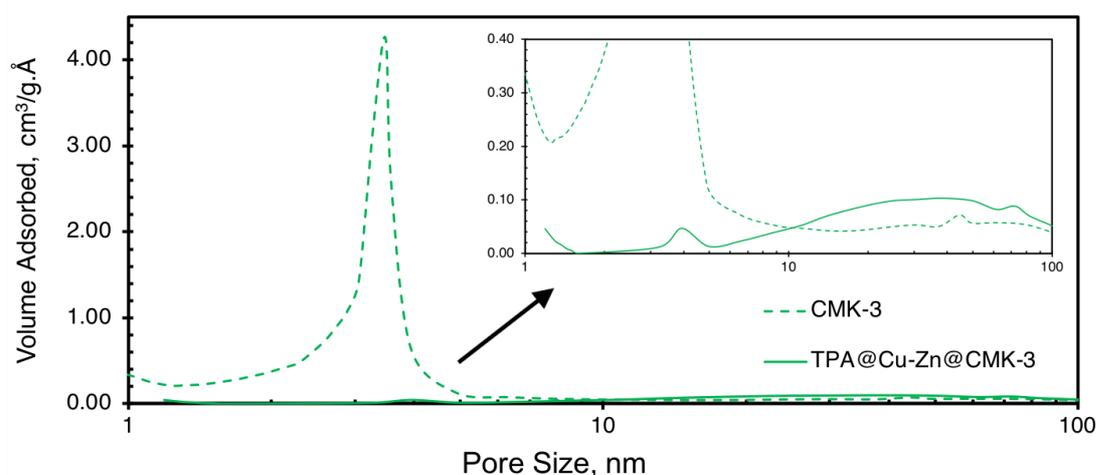
Figure 5.38. BJH desorption pore size distributions of CMK-3 support and TPA@Cu-Zn@CMK-3 bifunctional DME catalyst
