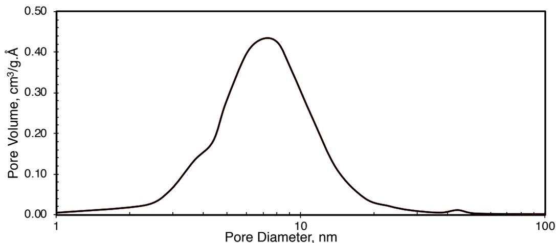
Figure 5.3. BJH desorption pore size distribution of MSC
