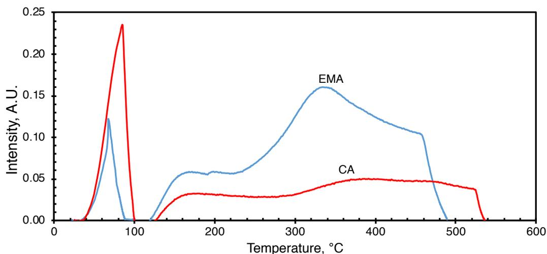
Figure 5.10. NH<sub>3</sub>-TPD curves of mesoporous alumina supports
