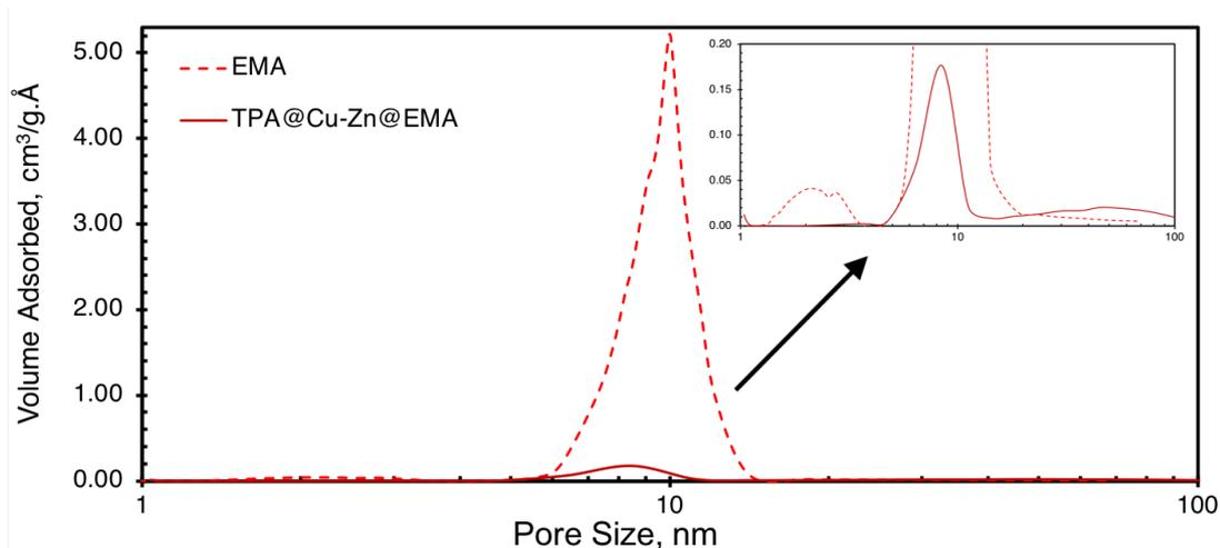
Figure 5.37. BJH desorption pore size distributions of EMA support and TPA@Cu-Zn@EMA bifunctional DME catalyst
