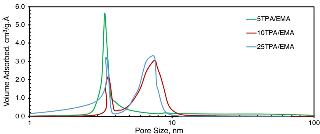
Figure 5.21. BJH desorption pore size distribution TPA loaded EMA catalysts using the one-pot method.
