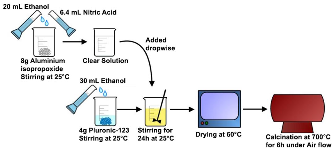
Figure 4.1. Synthesis of mesoporous alumina using EISA method.
