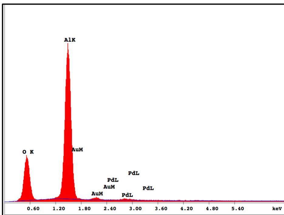
Figure 5.14. EDX spectrum of commercial alumina material
