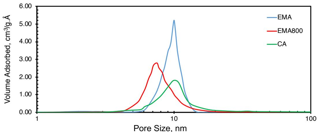
Figure 5.8. BJH desorption pore size distribution of mesoporous alumina materials
