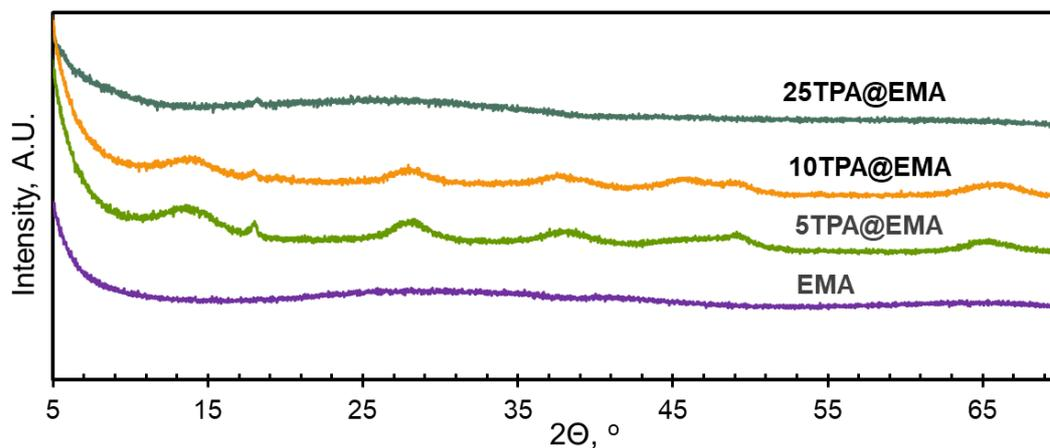
Figure 5.16. XRD patterns of TPA loaded alumina catalysts using the impregnation method
