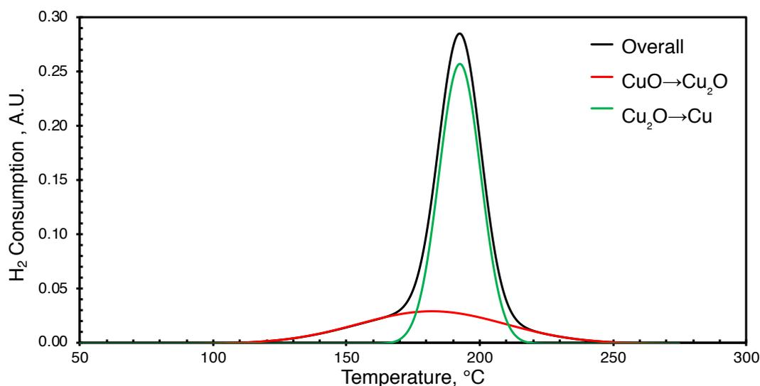
Figure 5.5. Peak deconvolution for TPR profile of MSC
