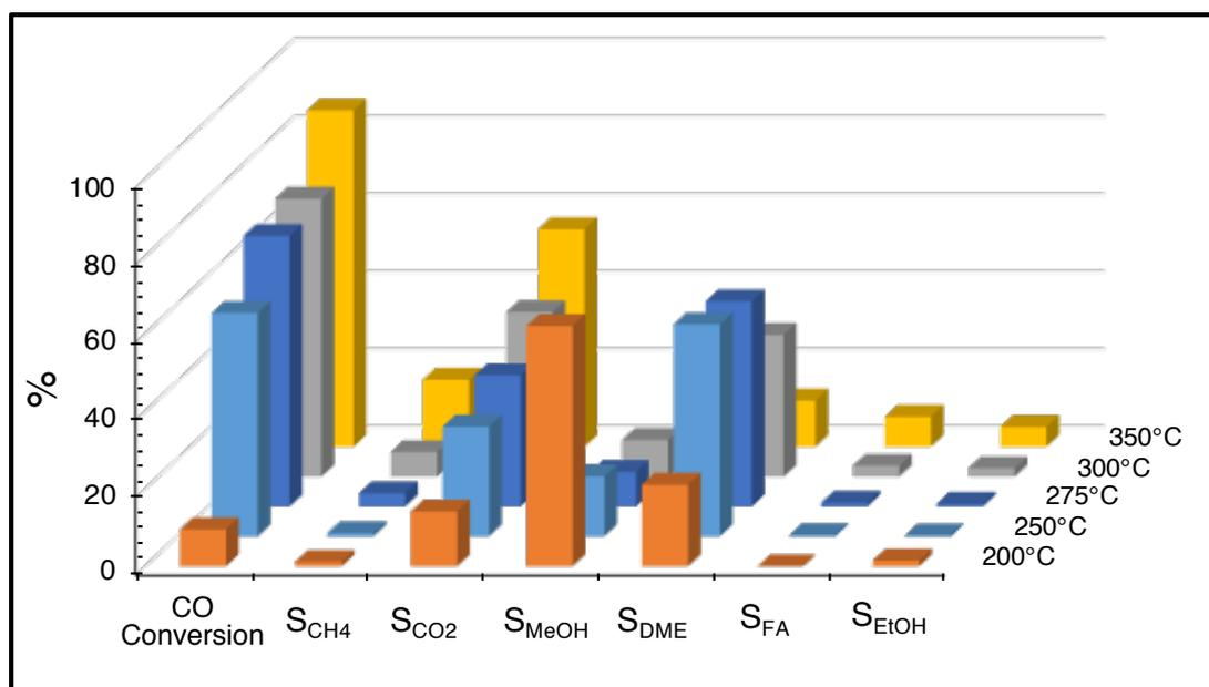
Figure 5.53. Effect of reaction temperature on CO conversion and product selectivities (P: 50 bar, H<sub>2</sub>/CO= 1/1, GHSV: 5000 ml/h.gcat, Catalyst: MSC+CA (1/1 by wt.))
