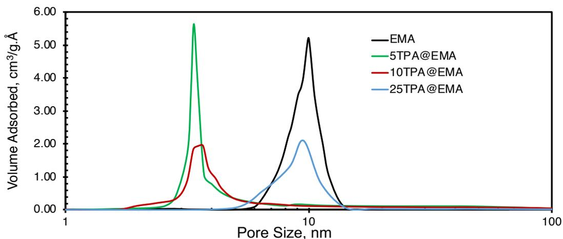
Figure 5.19. BJH desorption pore size distribution of EMA support and TPA loaded EMA catalysts
