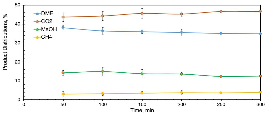
Figure 5.48. Product distribution of three runs with respect to time for DME repeatability tests (P: 50 bar, T: 275°C, H<sub>2</sub>/CO= 1/1, GHSV: 5000 ml/h.gcat, Catalyst: MSC + CA (1/1 by wt.))
