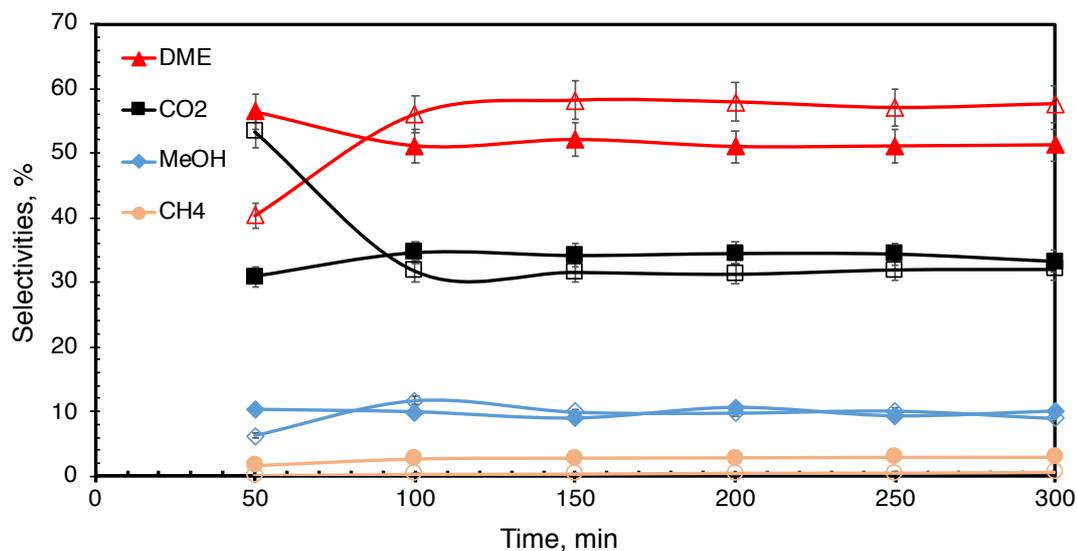
Figure 5.57. Effect of catalyst reduction on product selectivities on single step DME synthesis (P: 50 bar, T: 275°C, H<sub>2</sub>/CO= 1/1, GHSV: 5000 ml/h.gcat, Catalyst: MSC + CA (1/1 by wt)) (Filled symbols: reduced MSC and empty symbols: non-reduced MSC)
