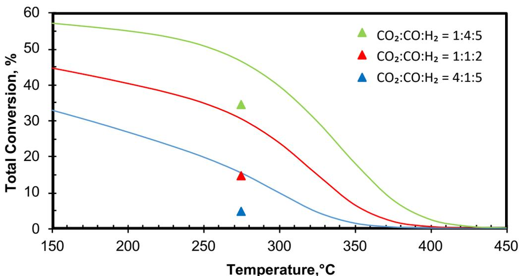
Figure 5.62. Effect of CO<sub>2</sub> content in syngas on total conversion and total equilibrium conversion (P: 50 bar, T: 275°C, GHSV: 5000 ml/h.gcat, Catalyst: MSC+CA (1/1 by wt.)) (Triangle symbols: experimental CO Conversion values)
