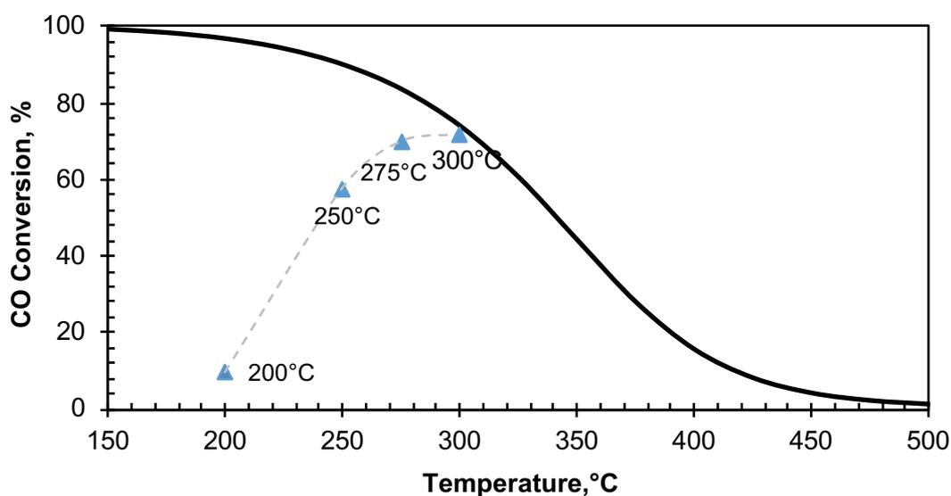
Figure 5.54. Effect of temperature on CO conversion and CO equilibrium conversion (P: 50 bar,  $\text{H}_2/\text{CO} = 1/1$ , GHSV: 5000 ml/h.gcat, Catalyst: MSC+CA (1/1 by wt.)) (Triangle symbols: experimental CO conversion values)
