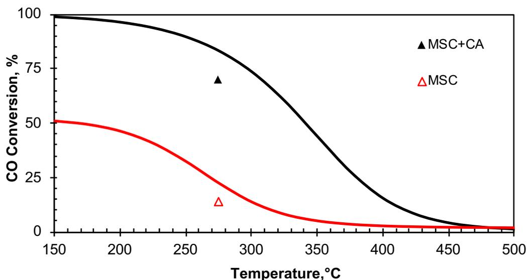
Figure 5.52. Comparison of CO conversion values obtained using the MSC and MSC+CA catalysts with the equilibrium conversion values (P: 50 bar, T: 275°C, H<sub>2</sub>/CO= 1/1, GHSV: 5000 ml/h.gcat, red: methanol synthesis equilibrium and black: DME synthesis equilibrium conversion curve)
