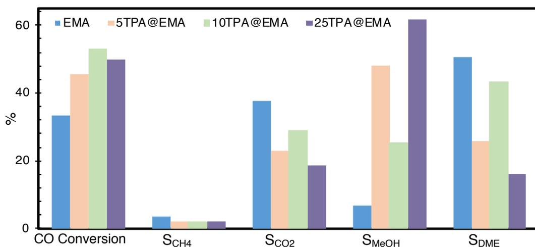
Figure 5.65. Effect of TPA amount impregnated to EMA support on CO conversion and product selectivities (P: 50 bar, T: 275°C, H<sub>2</sub>/CO= 1/1, GHSV: 5000 ml/h.gcat, Catalyst: each was physically mixed with MSC)
