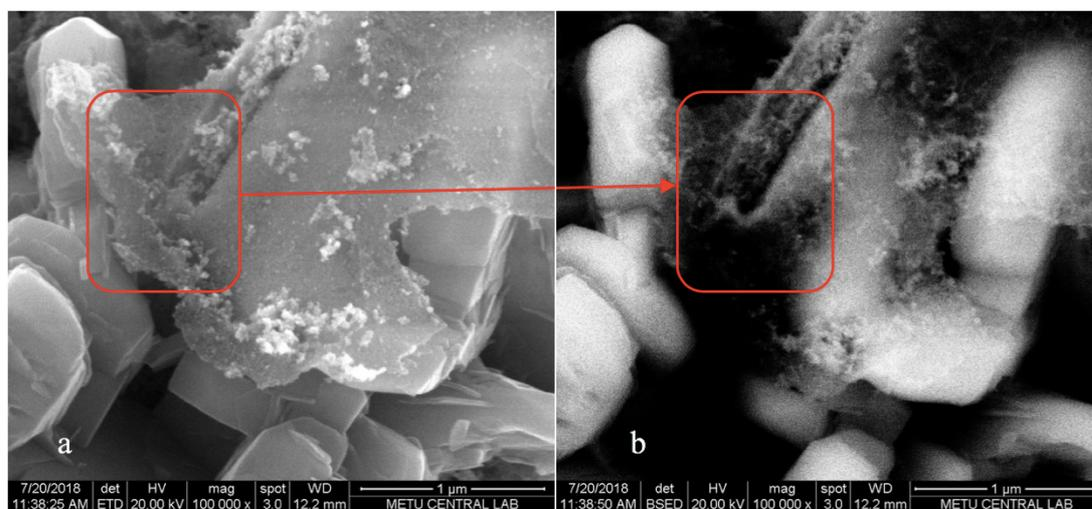
Figure 5.42. SEM (a) and backscattered electron (b) images of TPA@Cu-Zn@EMA catalyst at 100,000 magnification
