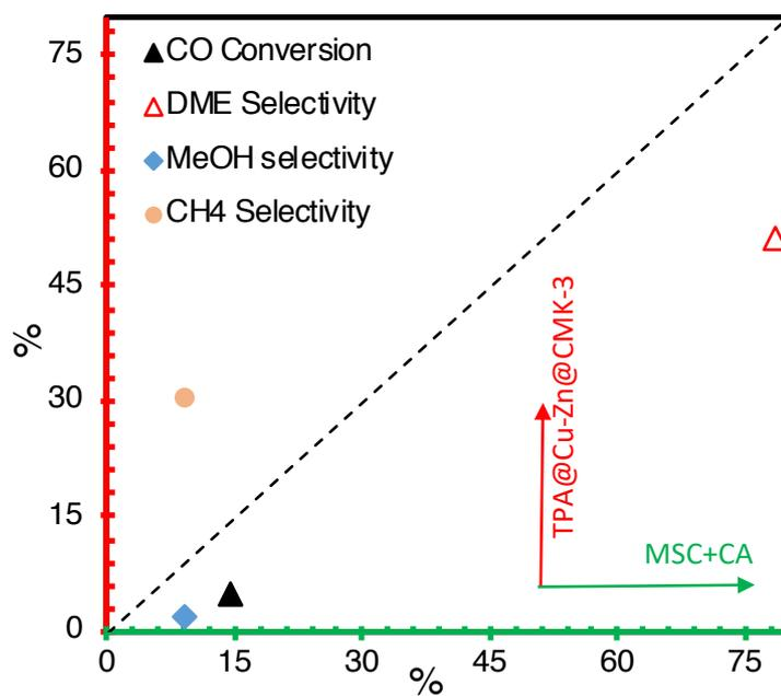
Figure 5.72. Comparison of bifunctional and physically mixed catalysts (P: 50 bar, T: 275°C, CO<sub>2</sub>/CO/H<sub>2</sub> = 1/1/2, GHSV: 5000 ml/h.gcat)
