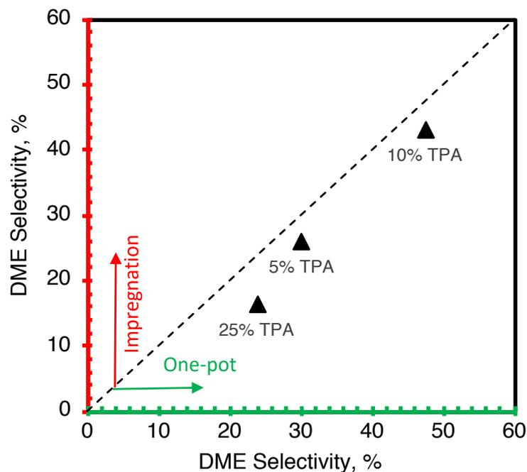
Figure 5.68. Effect of TPA loading method into support on DME selectivity (P: 50 bar, T: 275°C, H<sub>2</sub>/CO= 1/1, GHSV: 5000 ml/h.gcat, Catalyst: each was physically mixed with MSC)
