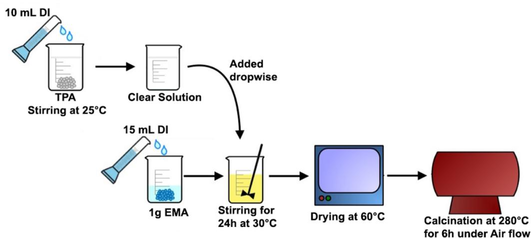
Figure 4.2. TPA loading on EMA support using impregnation method.
