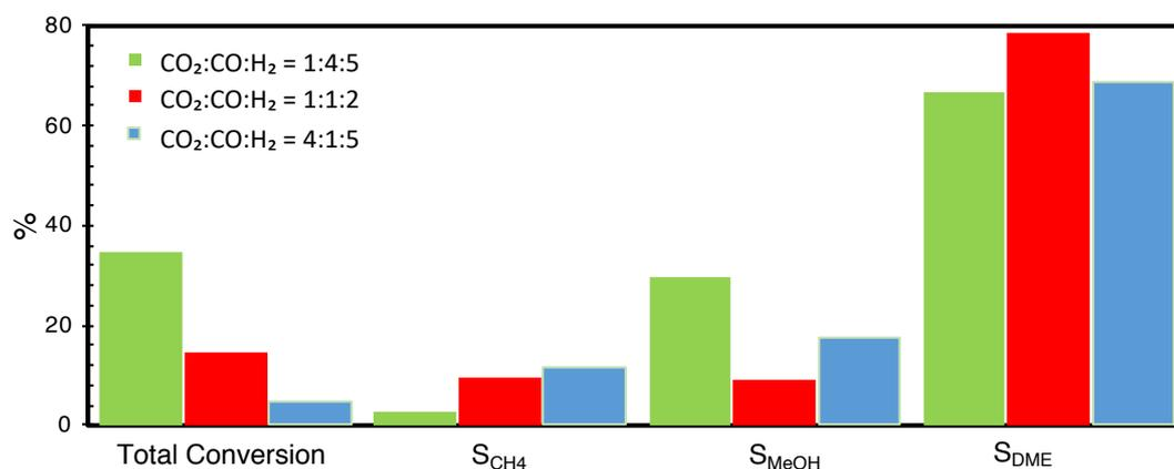
Figure 5.61. Effect of CO<sub>2</sub> content on total conversion and product selectivities (P: 50 bar, T: 275°C, GHSV: 5000 ml/h.geat, Catalyst: MSC + CA (1/1 by wt.))
