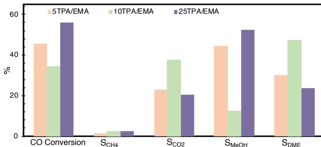
Figure 5.66. Effect of TPA amount loaded with one-pot method into EMA support on CO conversion and product selectivities (P: 50 bar, T: 275°C, H<sub>2</sub>/CO= 1/1, GHSV: 5000 ml/h.gcat, Catalyst: each was physically mixed with MSC)
