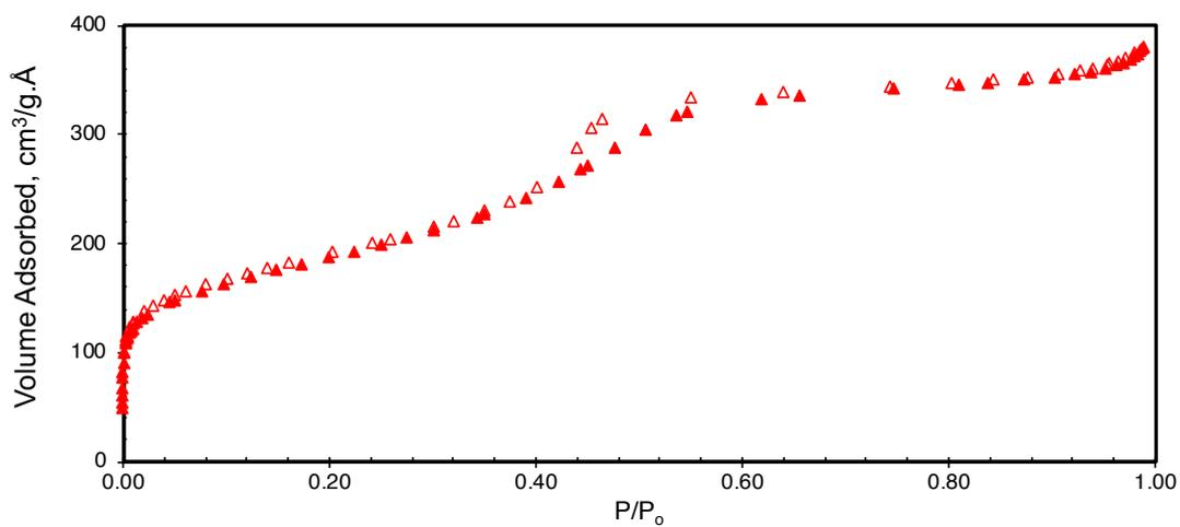
Figure 5.31. Nitrogen physisorption isotherm of CMK-3 support (filled symbols: adsorption and empty symbols: desorption branches).
