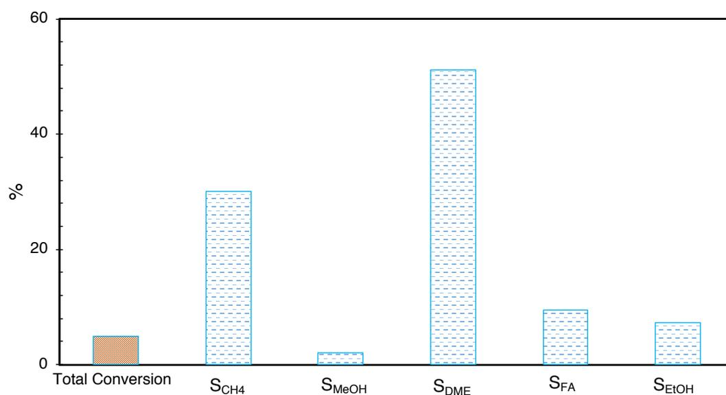
Figure 5.71. Total conversion and product selectivities of bifunctional TPA@Cu-Zn@CMK-3 catalyst (P: 50 bar, T: 275°C, CO<sub>2</sub>/CO/H<sub>2</sub> = 1/1/2, GHSV: 5000 ml/h.gcat)
