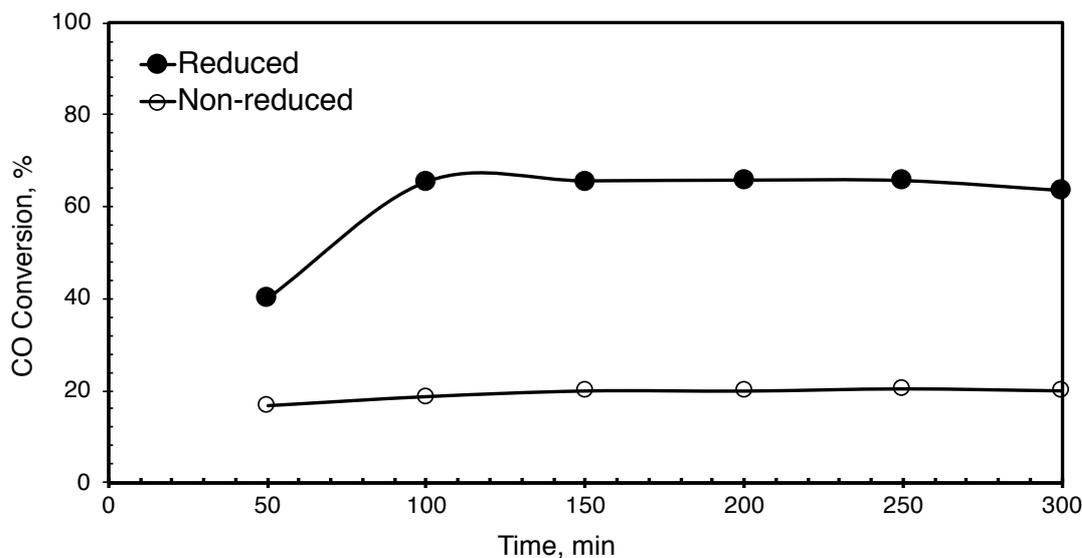
Figure 5.56. Effect of catalyst reduction on CO conversion (P: 50 bar, T: 275°C, H<sub>2</sub>/CO= 1/1, GHSV: 5000 ml/h.gcat, Catalyst: MSC + CA (1/1 by wt.)) (Filled symbols: reduced MSC, empty symbols: non-reduced MSC)
