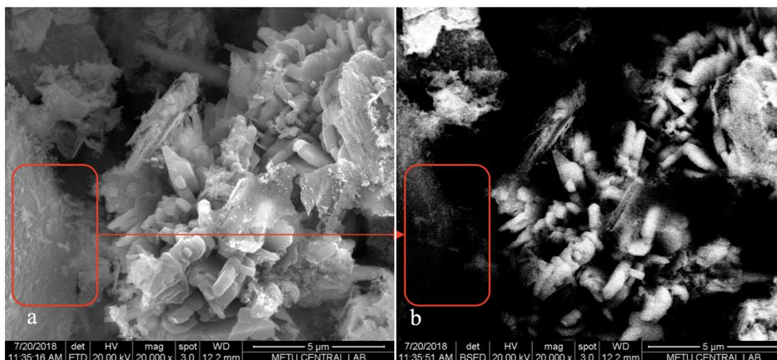
Figure 5.41. SEM (a) image and backscattered (b) images of TPA@Cu-Zn@EMA catalyst at 20,000 magnification
