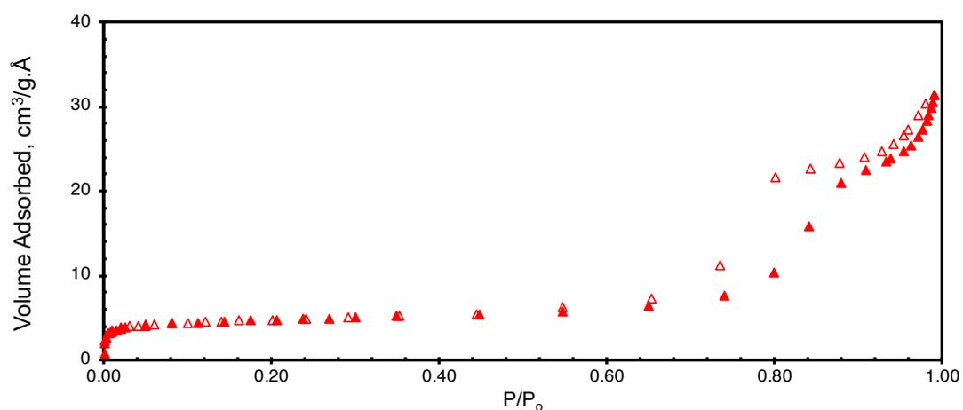
Figure 5.35. Nitrogen physisorption isotherm of TPA@Cu-Zn@EMA bifunctional DME catalyst (filled symbols: adsorption and empty symbols: desorption branches)
