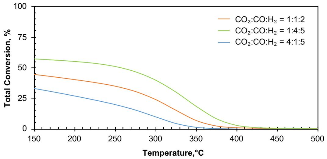
Figure 3.5. Effect of CO<sub>2</sub> composition in syngas on total conversion
