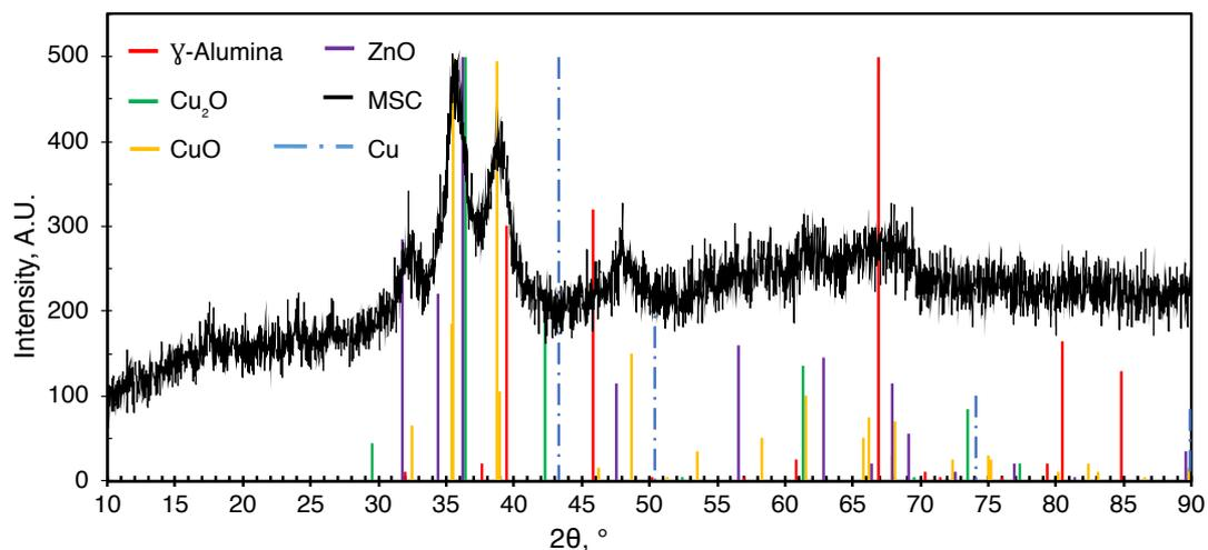
Figure 5.1. XRD pattern of commercial methanol synthesis catalyst (MSC) with XRD data of  $\text{Cu}_2\text{O}$ ,  $\text{CuO}$ ,  $\text{ZnO}$  and  $\gamma$ -alumina materials
