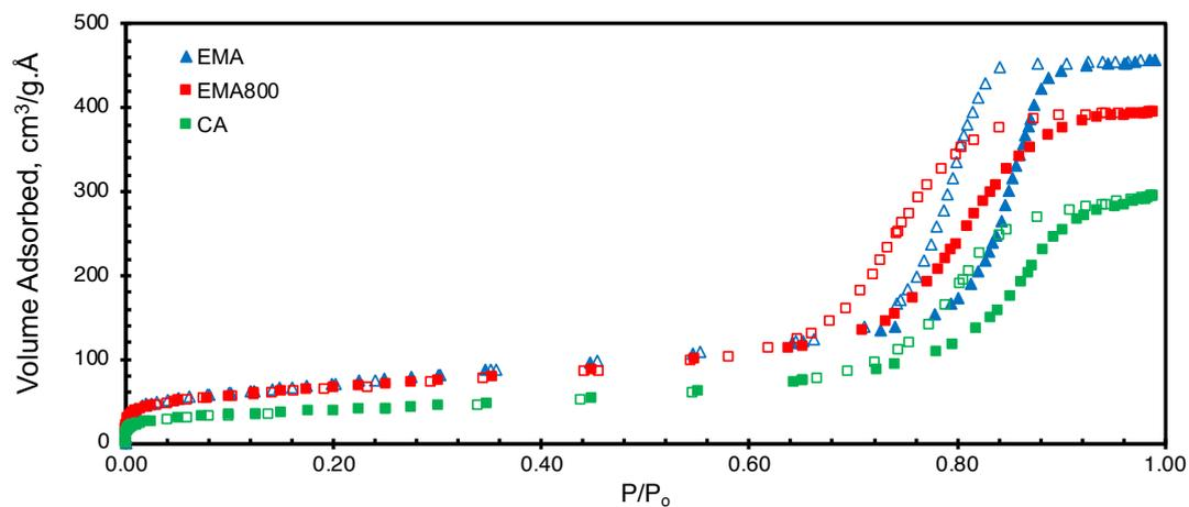
Figure 5.7. Nitrogen physisorption isotherms of alumina support (filled symbols: adsorption and empty symbols: desorption branches)
