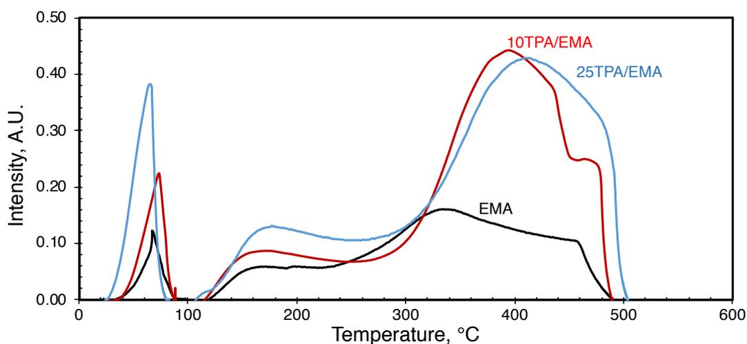
Figure 5.24. NH<sub>3</sub>-TPD curves of EMA support and TPA loaded EMA catalysts using one-pot method
