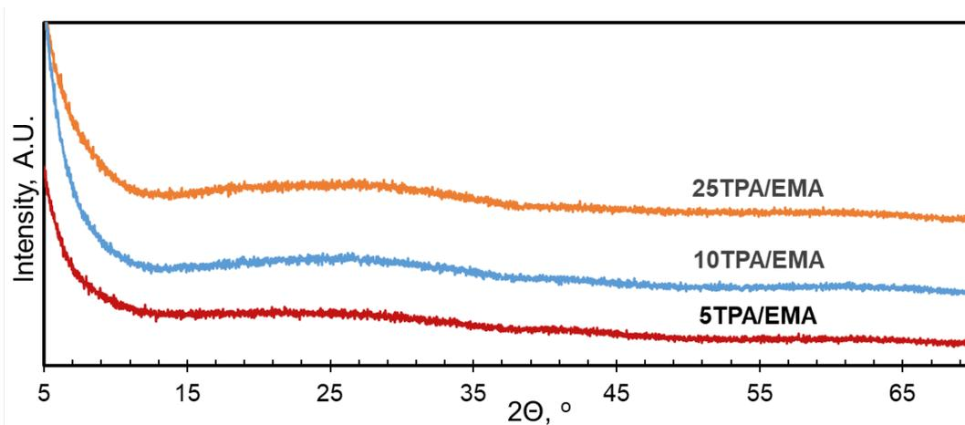
Figure 5.17. XRD patterns of TPA loaded alumina catalysts using the one-pot method
