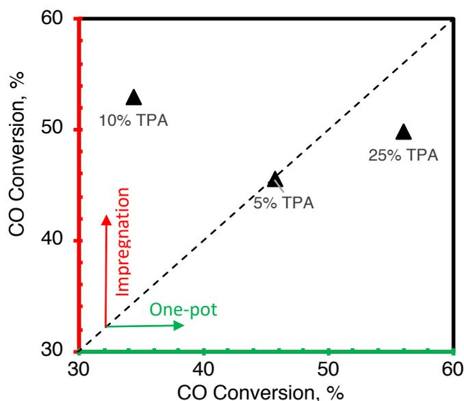
Figure 5.67. Effect of TPA loading method into support on CO conversion (P: 50 bar, T: 275°C, H<sub>2</sub>/CO= 1/1, GHSV: 5000 ml/h.gcat, Catalyst: each was physically mixed with MSC)
