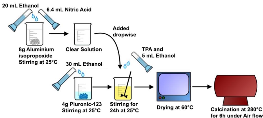
Figure 4.3. TPA loading on EMA using one-pot method.
