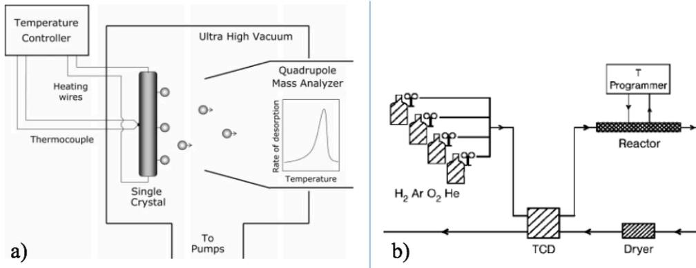
Figure 4.4. TPD set-up a) UHV chamber coupled with MS b) flow set-up coupled with TCD (adapted from (Niemantsverdriet, 2007))
