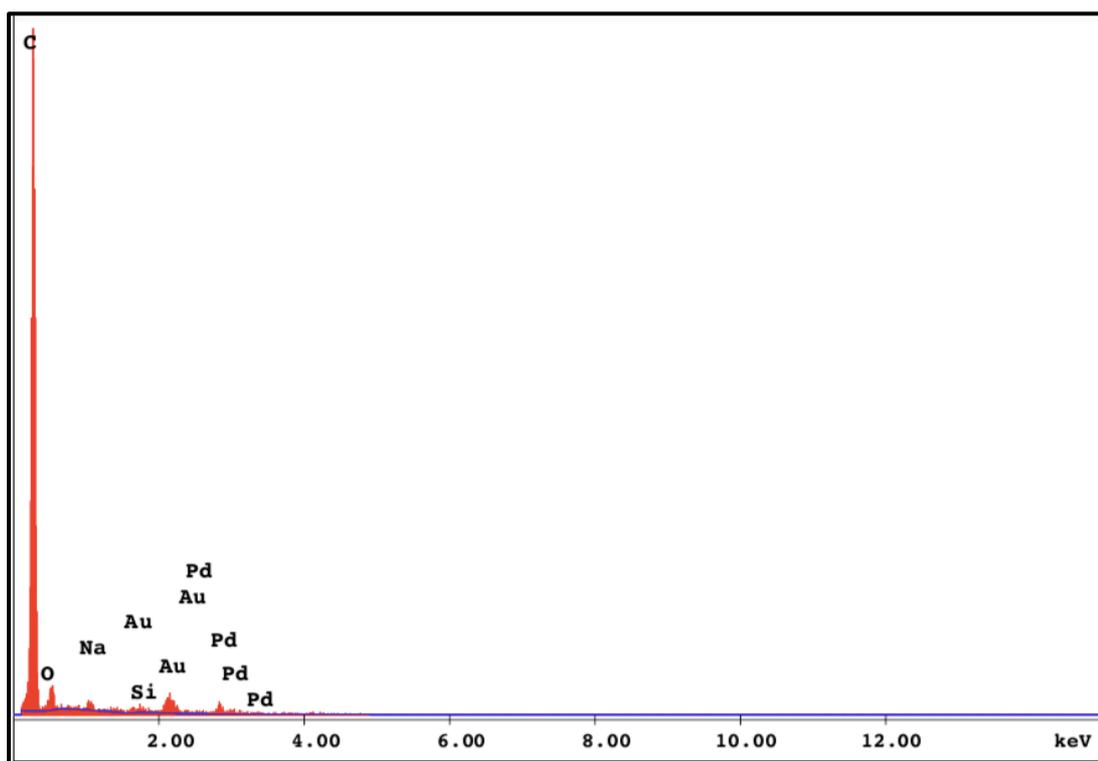
Figure 5.34. EDX spectrum of CMK-3 support
