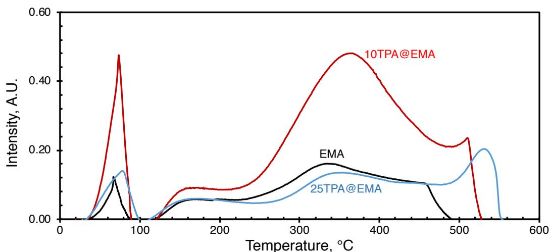
Figure 5.22.  $\text{NH}_3$ -TPD curves of EMA support and TPA impregnated EMA catalysts
