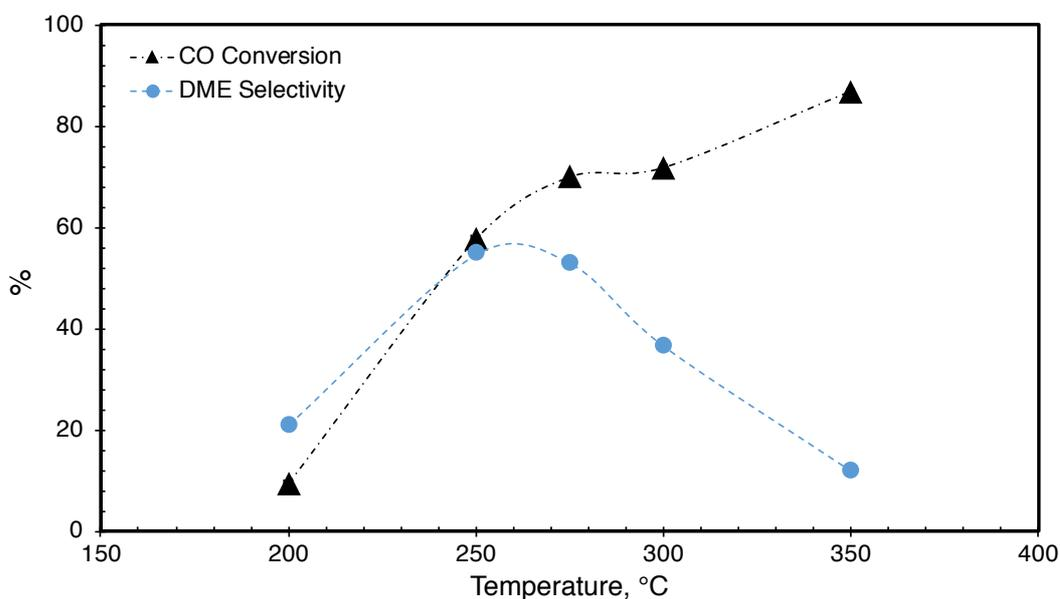
Figure 5.55. Temperature effect on CO conversion and DME selectivity (P: 50 bar, H<sub>2</sub>/CO= 1/1, GHSV: 5000 ml/h.gcat, Catalyst: MSC + CA (1/1 by wt.))
