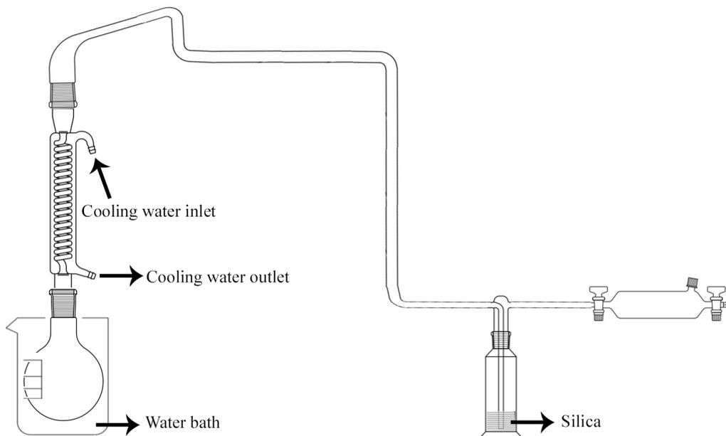
Figure 4.5. Ammonia purification set-up used in ammonia calibration
