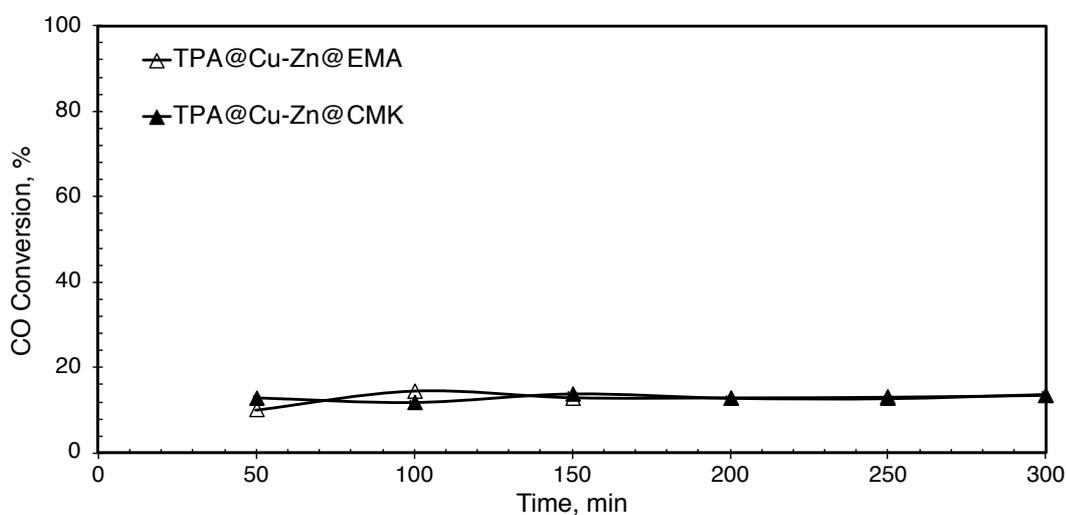
Figure 5.69. CO conversion in the presence of bifunctional DME synthesis catalysts (P: 50 bar, T: 275°C, H<sub>2</sub>/CO= 1/1, GHSV: 5000 ml/h.gcat)
