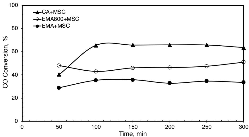
Figure 5.63. Effect of type of alumina on CO conversion (P: 50 bar, T: 275°C, H<sub>2</sub>/CO= 1/1, GHSV: 5000 ml/h.gcat, Catalyst: alumina support + MSC (1/1 by wt.))
