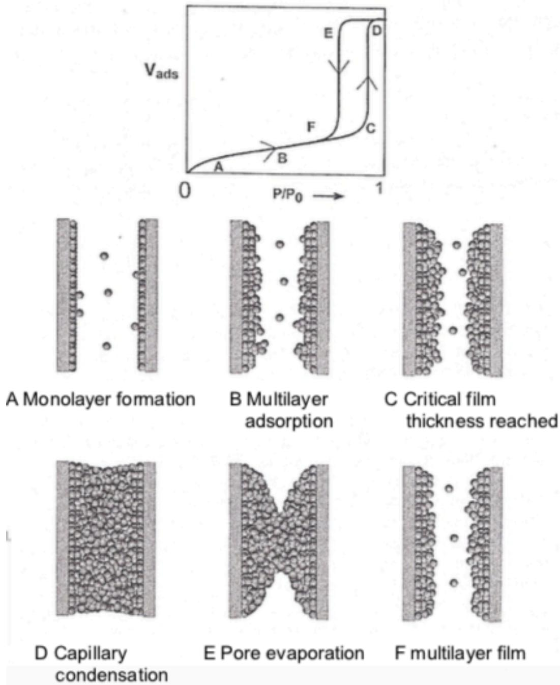
Figure 2.1. Capillary condensation mechanism (Trunschke, 2013)
