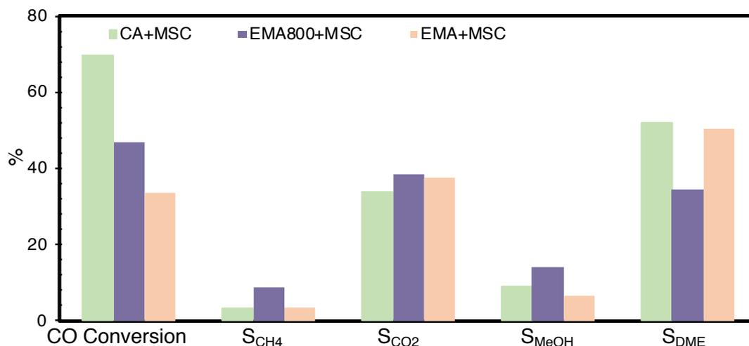
Figure 5.64. Effect of different mesoporous alumina catalysts on average CO conversion and product selectivities (P: 50 bar, T: 275°C, H<sub>2</sub>/CO= 1/1, GHSV: 5000 ml/h.gcat, Catalyst: alumina support + MSC (1/1 by wt.))
