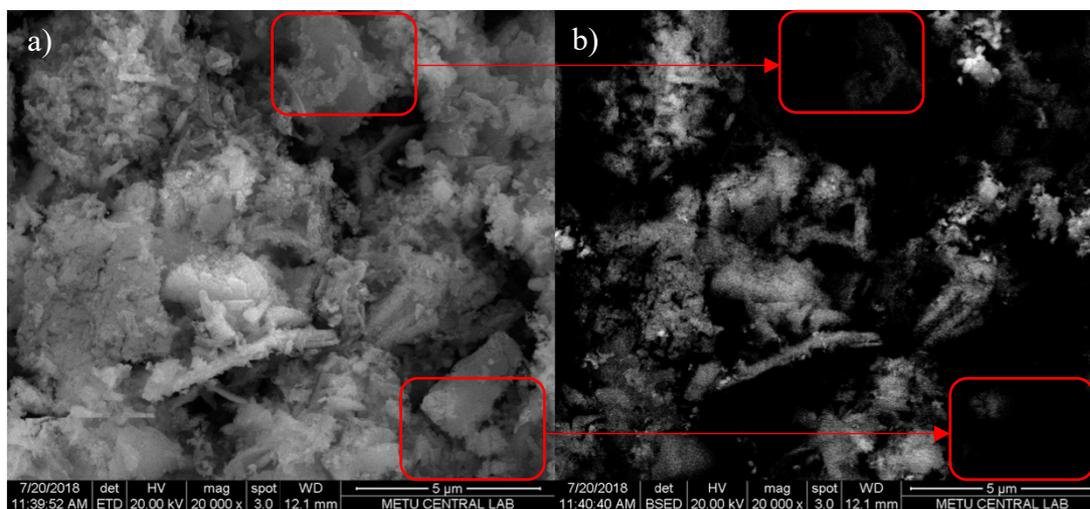
Figure 5.44. SEM (a) and backscattered electron (b) images of TPA@Cu-Zn@CMK-3 catalyst at 20,000 magnification
