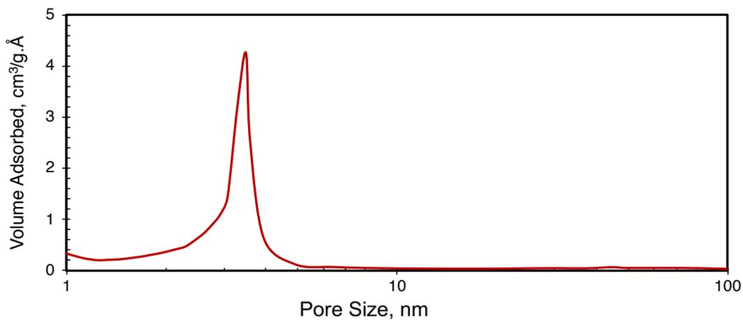
Figure 5.32. BJH desorption pore size distribution of CMK-3 support
