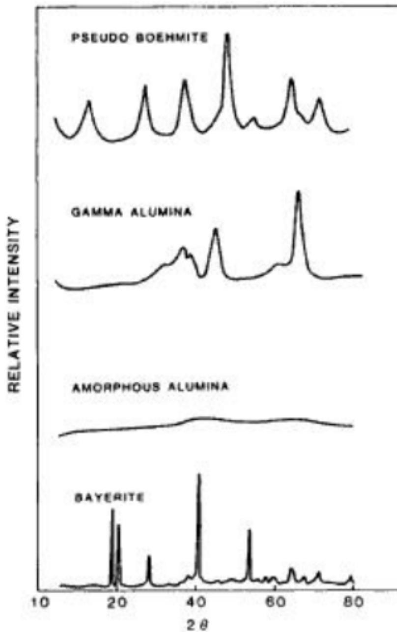
Figure 2.3. XRD patterns of different types of alumina structures (Richardson, 1989)
