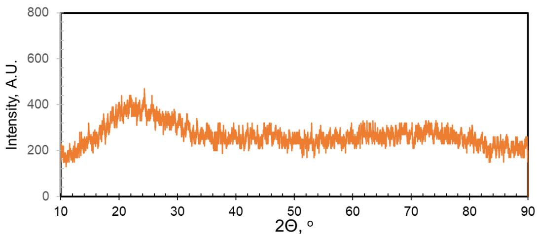
*Figure 5.30.* XRD pattern of CMK-3 support.
