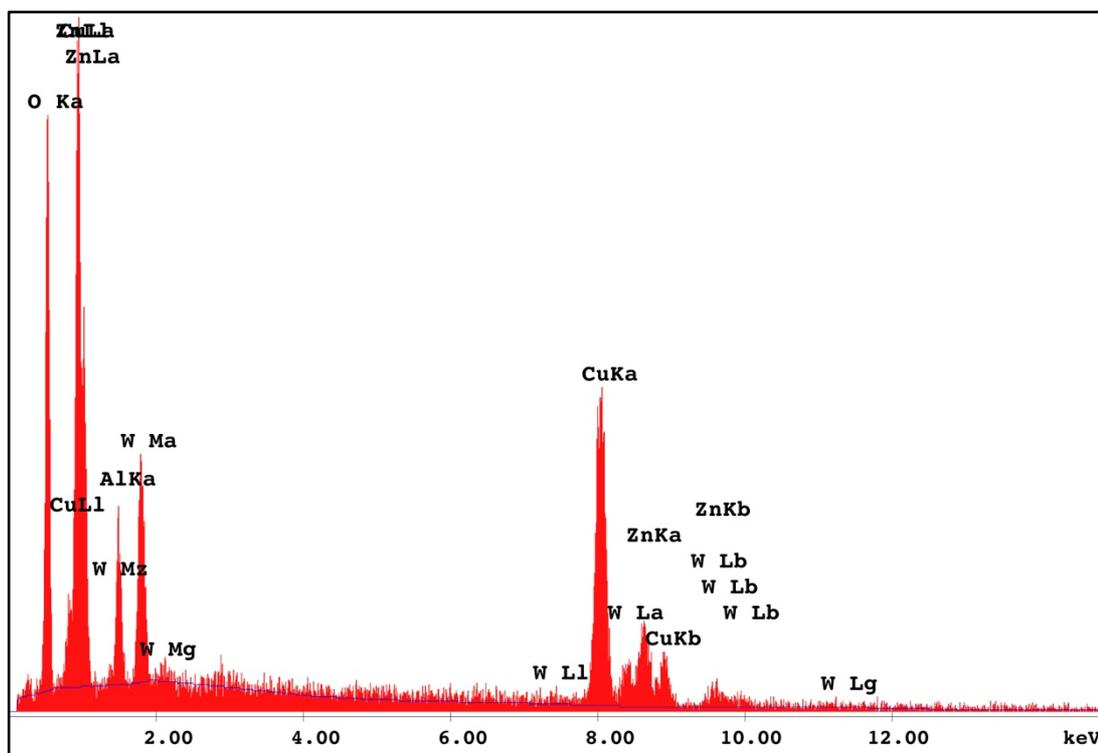
Figure 5.43. EDX spectrum of the TPA@Cu-Zn@EMA catalyst
