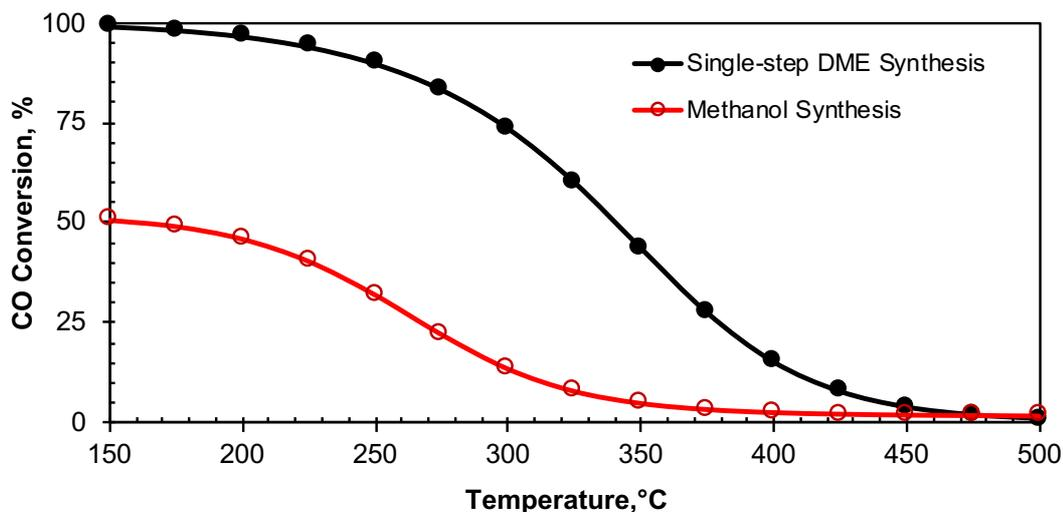
Figure 3.1. Comparison of CO equilibrium conversion for methanol and the direct DME syntheses (P: 50 bar, H<sub>2</sub>/CO= 1/1,) (Filled symbols: the single-step DME synthesis and empty red symbols: methanol synthesis)
