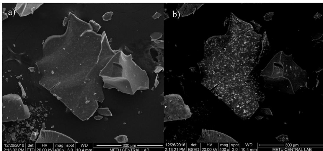
*Figure 5.29.* SEM (a) and backscattered electron (b) images of the 25TPA/EMA catalyst at 400 magnification
