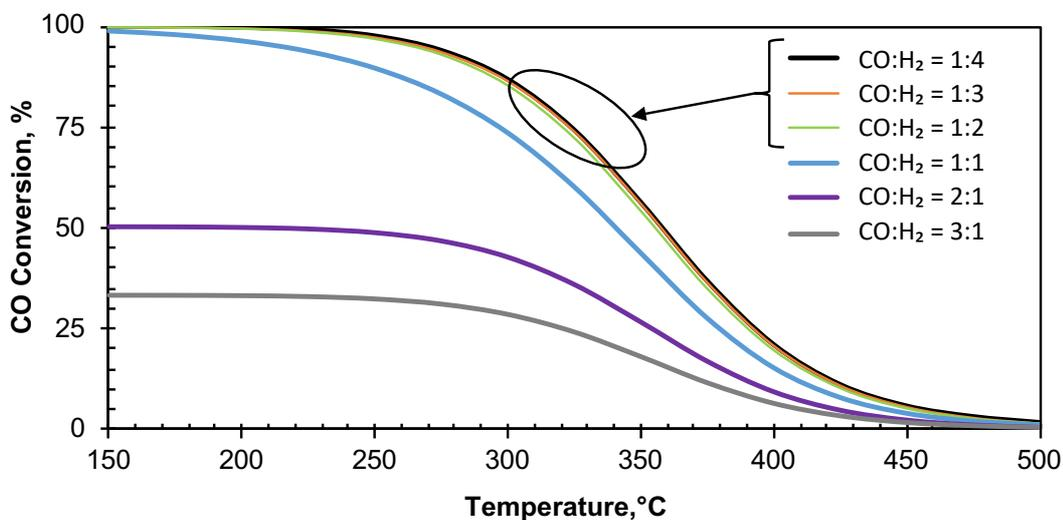
Figure 3.3. Effect of molar CO:H<sub>2</sub> feed ratio on CO equilibrium conversion at 50 bar
