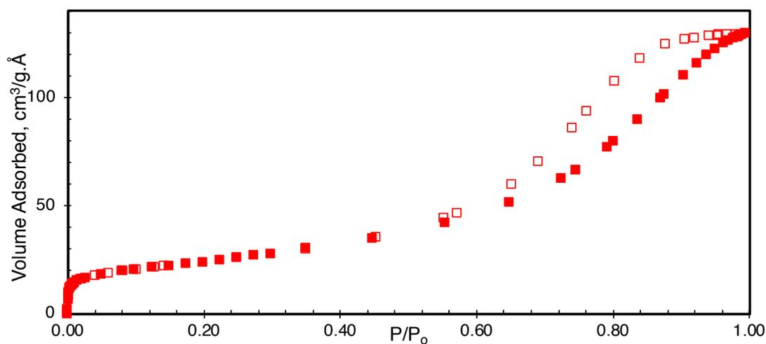
Figure 5.2. Nitrogen physisorption isotherm of MSC (filled symbols: adsorption and empty symbols: desorption branches)
