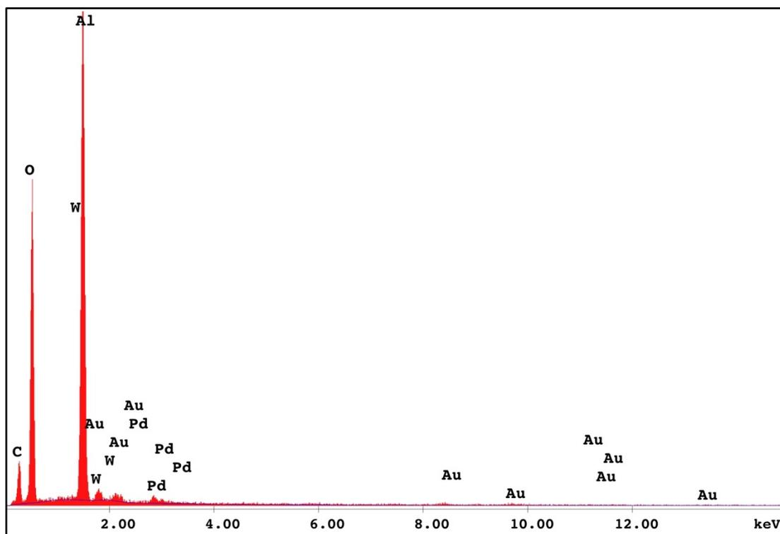
Figure 5.26. EDX spectrum of 5TPA@EMA
