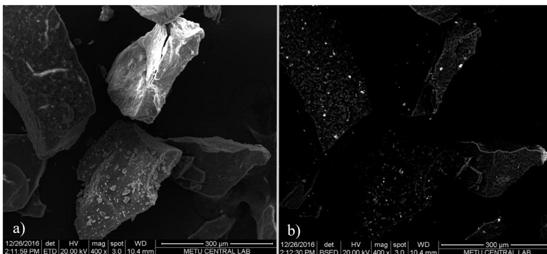
*Figure 5.28.* SEM (a) and backscattered electron (b) images of the 10TPA/EMA catalyst at 400 magnification
