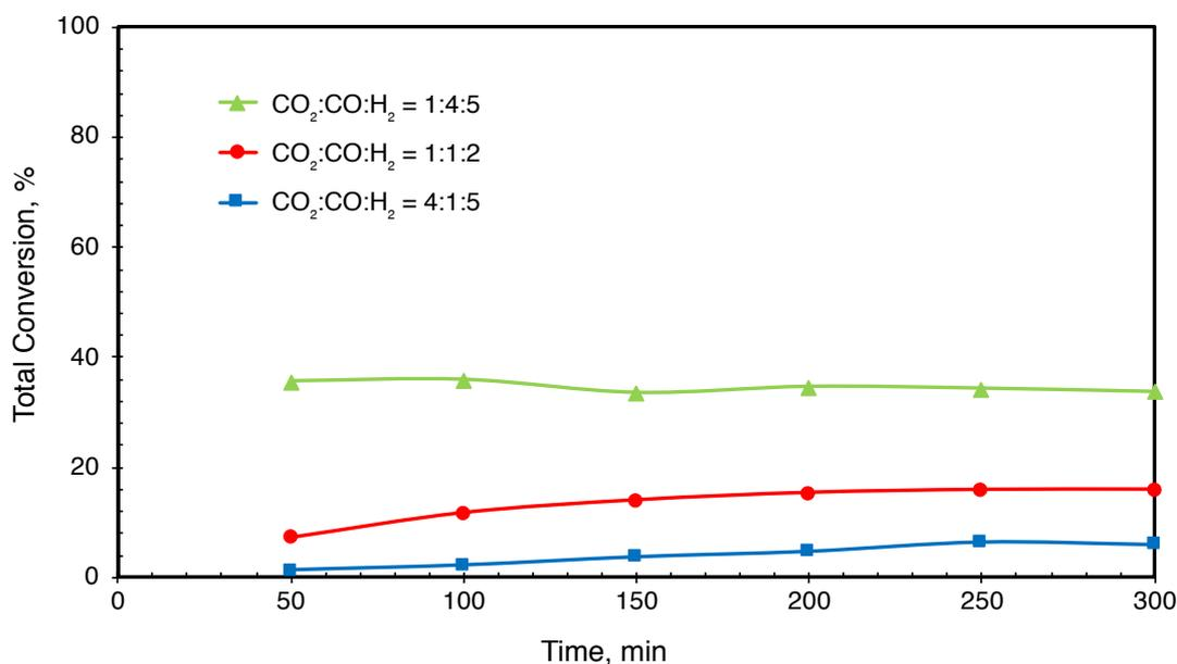
Figure 5.60. Effect of syngas composition on total conversion (P: 50 bar, T: 275°C, CO<sub>2</sub>/CO/H<sub>2</sub> = 1/4/5, GHSV: 5000 ml/h.gcat, Catalyst: MSC + CA (1/1 by wt.))
