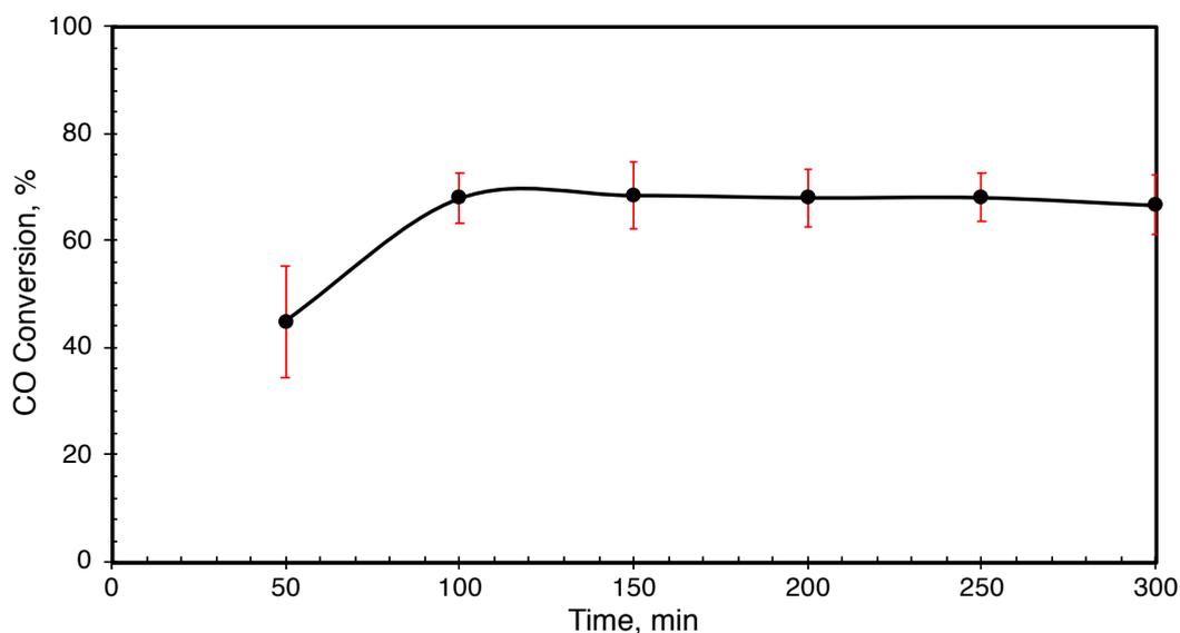
Figure 5.47. Average CO conversion of three runs with respect to time for DME repeatability tests (P: 50 bar, T: 275°C, H<sub>2</sub>/CO= 1/1, GHSV: 5000 ml/h.gcat, Catalyst: MSC + CA (1/1 by wt.))
