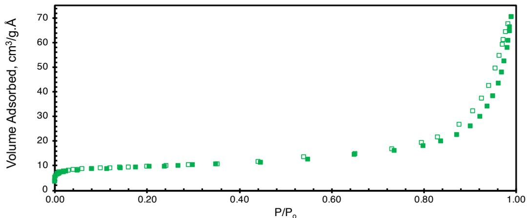
Figure 5.36. Nitrogen physisorption isotherm of TPA@Cu-Zn@CMK-3 bifunctional DME catalyst (filled symbols: adsorption and empty symbols: desorption branches)
