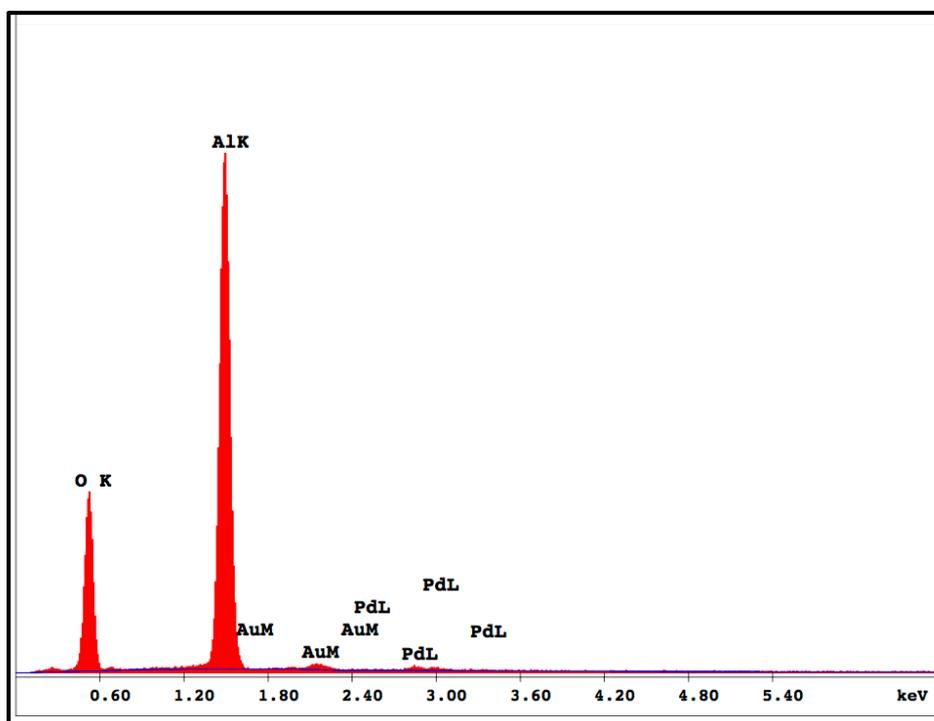
Figure 5.12. EDX spectrum of EMA support
