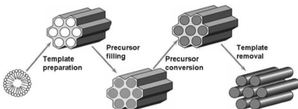
Figure 2.4. Schematic illustration of the nanocasting technology (de Jong, 2009)
