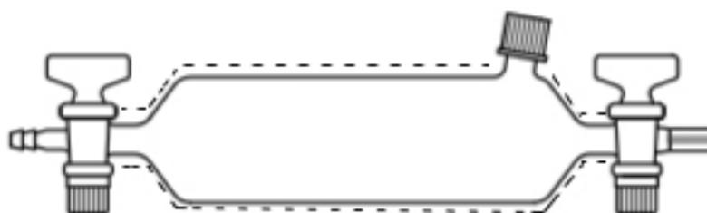
Figure 4.7. Gas sampling bottle (dashed lines indicates the heat zones)
