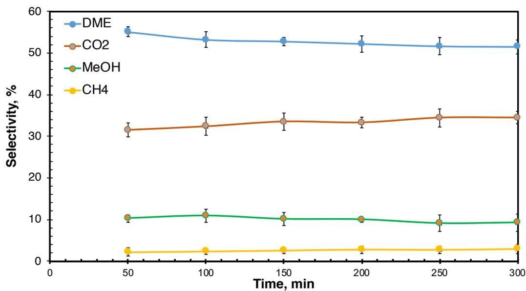
Figure 5.49. Product selectivities of three runs with respect to time for DME repeatability tests (P: 50 bar, T: 275°C, H<sub>2</sub>/CO= 1/1, GHSV: 5000 ml/h.gcat, Catalyst: MSC + CA (1/1 by wt.))
