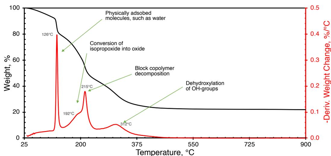
Figure 5.9. TGA curve of uncalcined mesoporous alumina
