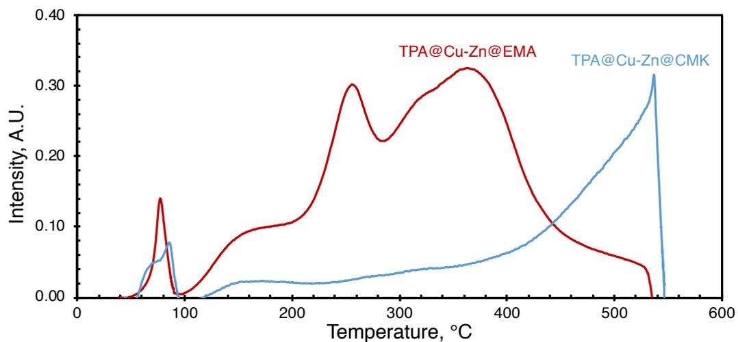
Figure 5.39. NH<sub>3</sub>-TPD curves of bifunctional DME catalysts
