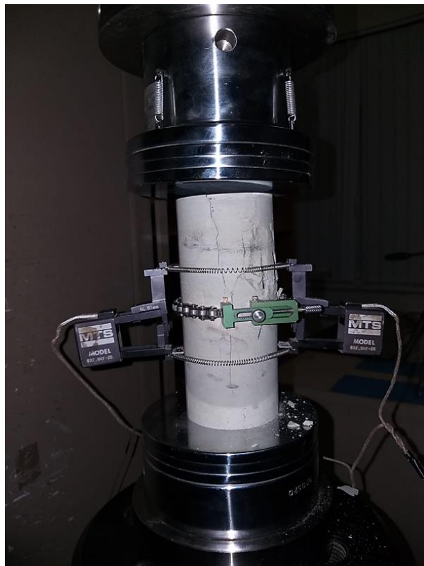
Figure 4-4: Static deformability test sample with axial and lateral extensometers after loading
