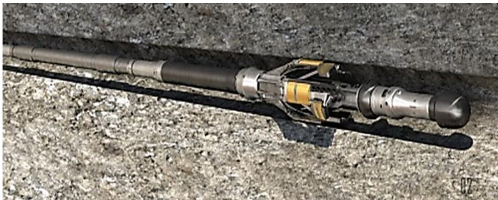
Figure 3-1: FMI tool with four pads in a borehole (Schlumberger, 2018)
