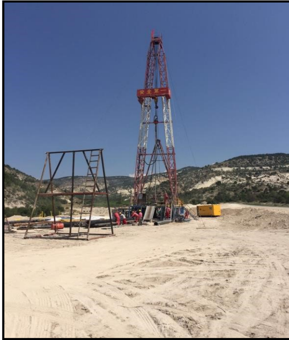
Figure 15. While drilling a vertical well with rotary-table rig
