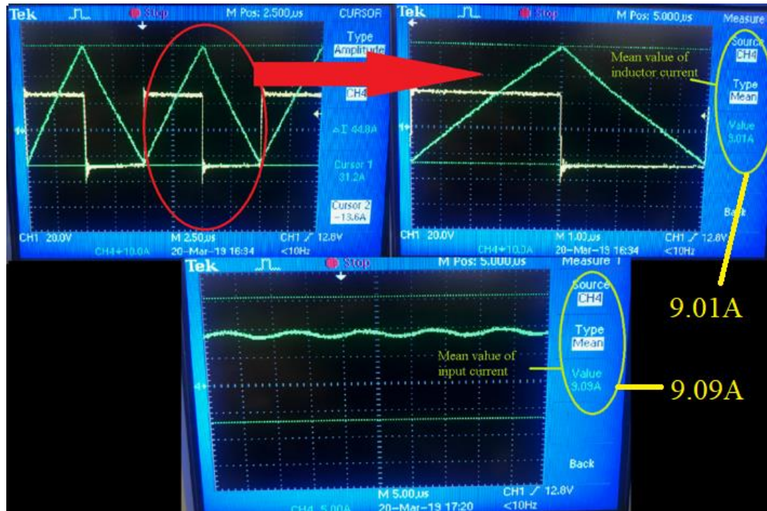
Figure 4.25. Inductor voltage (up-yellow), current (up-green) and input current (bottom) waveforms while V_2=28V , V_1=56V and P=250W for conventional operation (Test)
