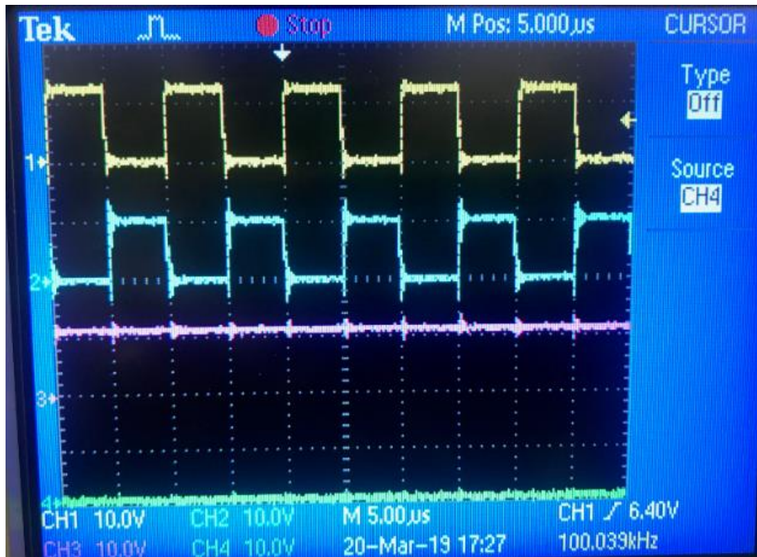
Figure 4.22. Gating signal waveforms (Gate SW1 : yellow, Gate SW2 : blue, Gate SW3 : pink, Gate SW4 : green) for switching devices while V_2=28\text{V} , V_1=56\text{V} and P=250\text{W} for conventional operation (Test)
