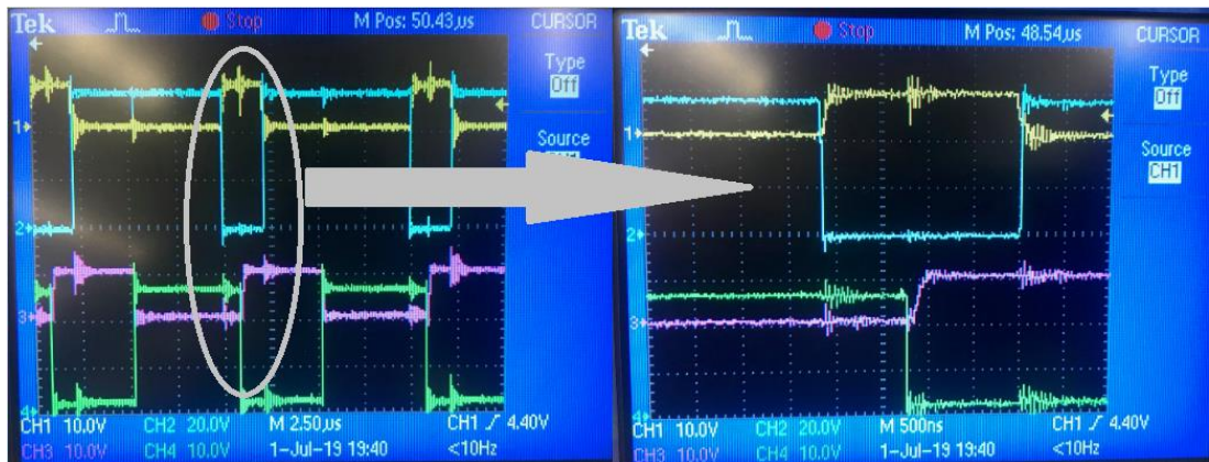
Figure 4.7. Switching device S1 gate (yellow) and V_{ds} (blue) voltage, switching device S3 gate (purple) and V_{ds} (green) voltage waveforms while V_1=56V , V_2=28V and P=250W for phase shifted operation (Test)
