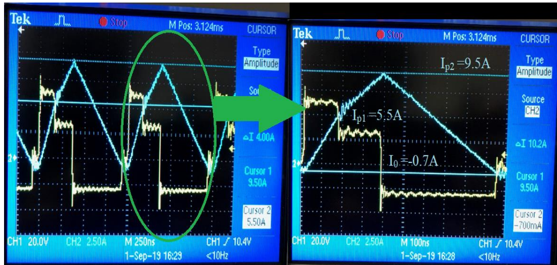
Figure 5.4. Inductor voltage (yellow) and current (blue) waveforms while V_1=56V , V_2=28V and P=112W for phase shifted operation with GaN
