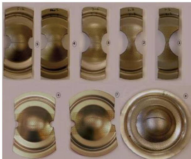
Figure 3.2 Example of blank specimens for Nakazima test [8]
