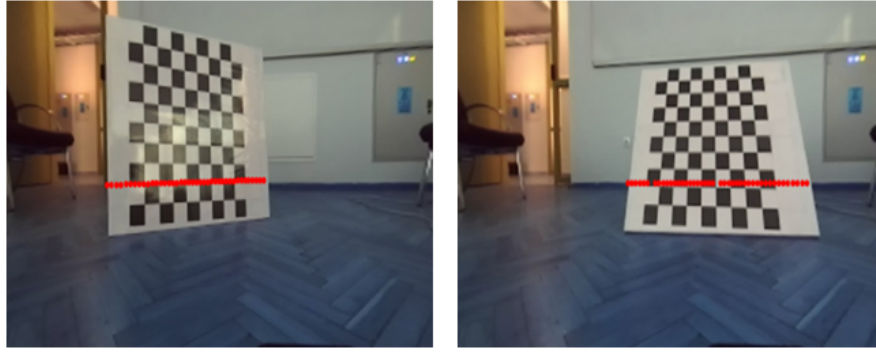
Figure 4.6: Laser scans hitting the chekerboard
