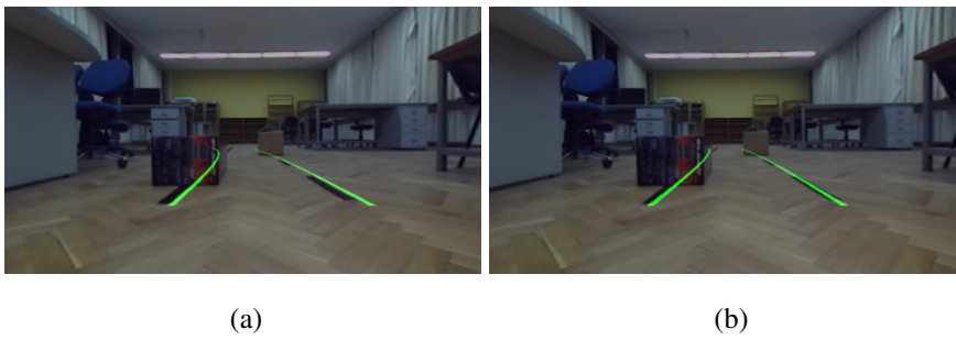
Figure 4.27: Lane detection illustrations without and with 2D LIDAR, respectively
