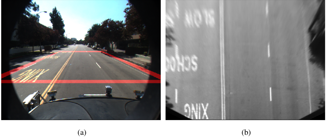
Figure 3.3: The fixed ROI (a) and grayscale BEV image (b)
