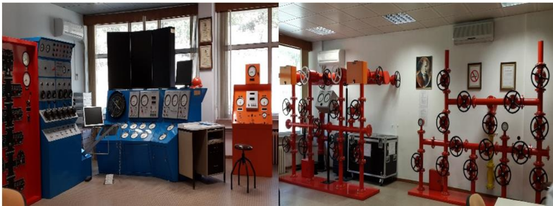
Figure 4.1. Well Control Simulator, DrillSIM 5000Enter the Figure Caption here
