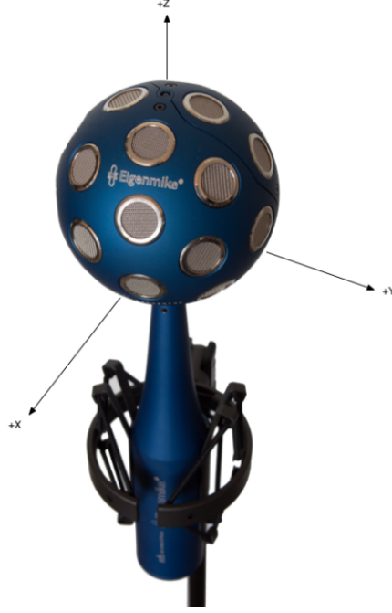
Figure 2.4: em32 Eigenmike spherical microphone array
