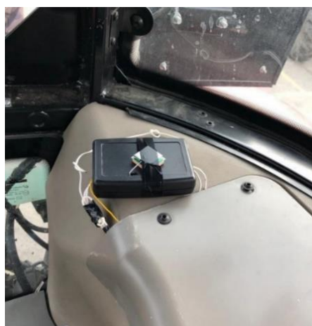
Figure 4.7. Data acquisition and storage unit
