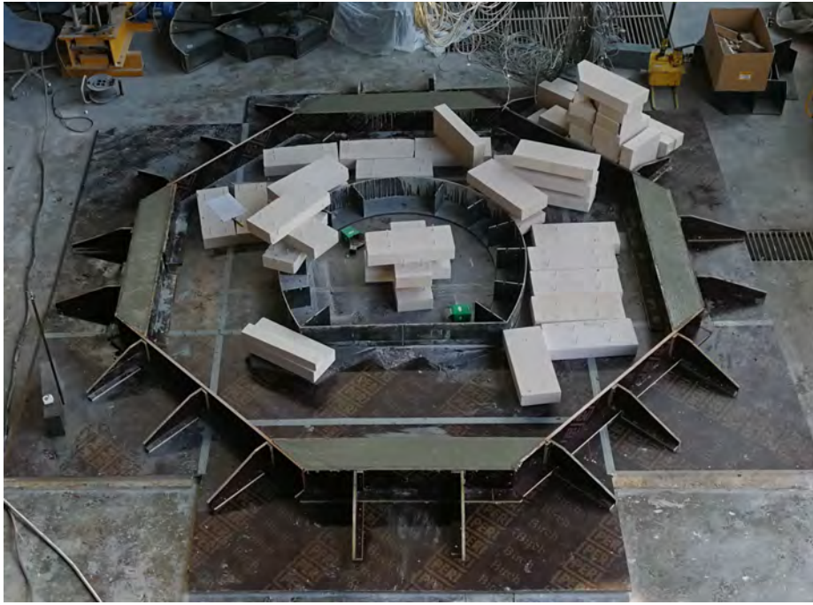
Figure 3.7: Photograph of laboratory model after casting of Buffer RC Beam and before application of rock substitute
