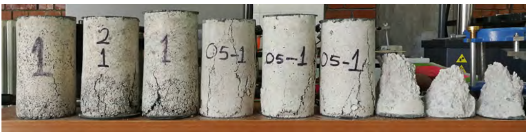
Figure A.3: Rubberized concrete samples after compression test: %100, %50 and control groups from left to right
