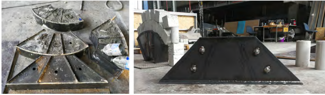
Figure 3.2: Concrete filling process and roller supports of pressure transmitting sections
