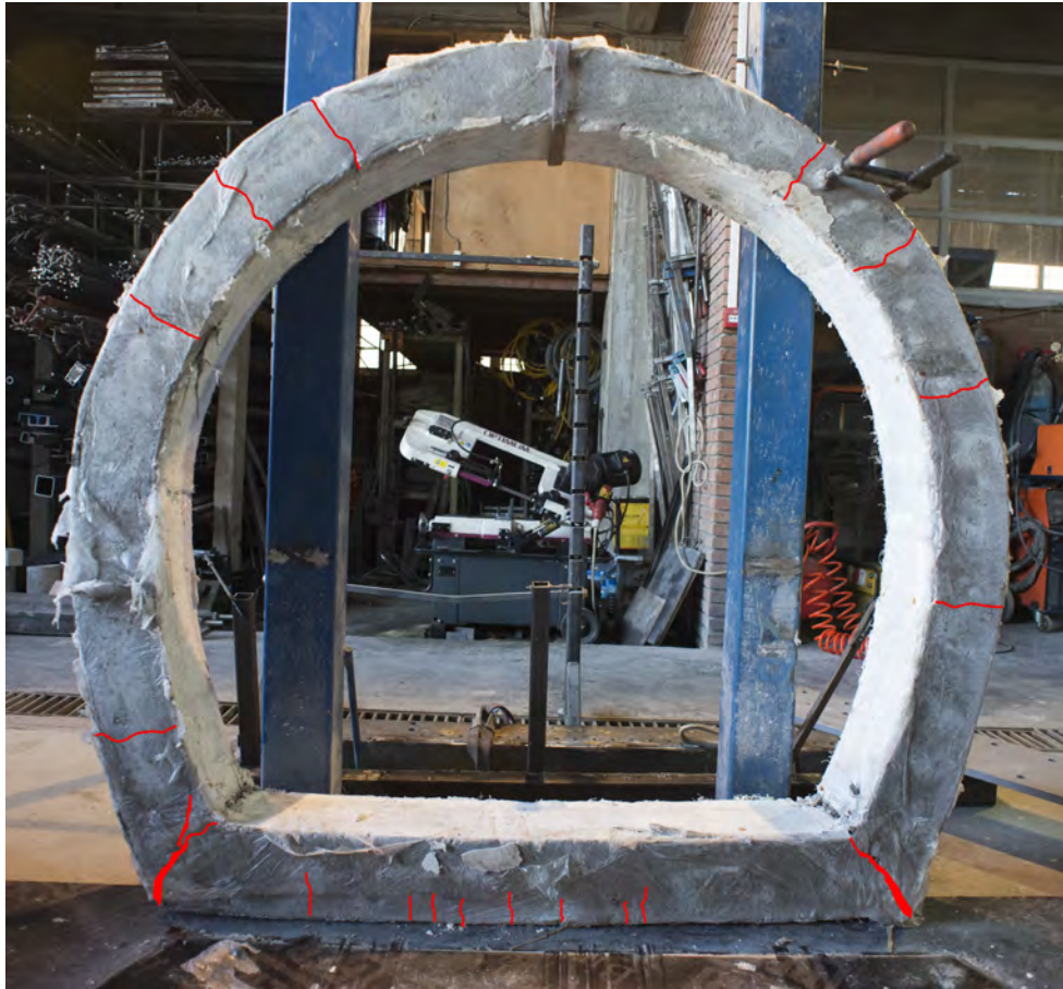
Figure 4.13: Crack map after NCF experiment
