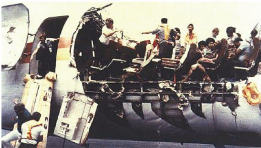
Figure 1.1. The Aloha Airways Boeing 737 which lost part of its top skin over Hawaii in 1988 showing convergent tears in the fuselage skin below floor level [1].
