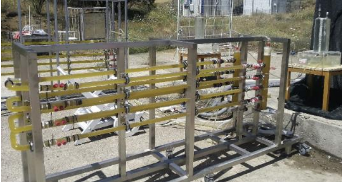
Figure 0.8. A stacked U-tube photobioreactor with internal cooling by manifolds in outdoor conditions.
