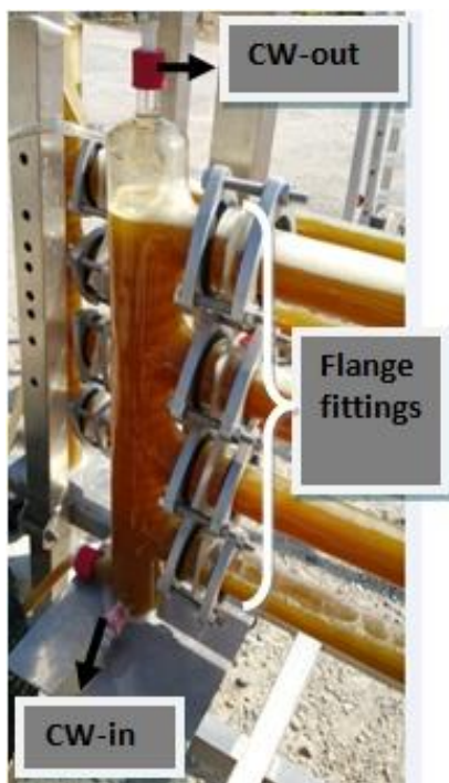
Figure 0.12. A photograph of (a) stacked U-tube photobioreactor (b) inlet manifold performed with R. capsulatus hup- on molasses. CW-in and CW-out are coolant water inlet and outlet, respectively. The experiment started on August 7 th , 2016.
