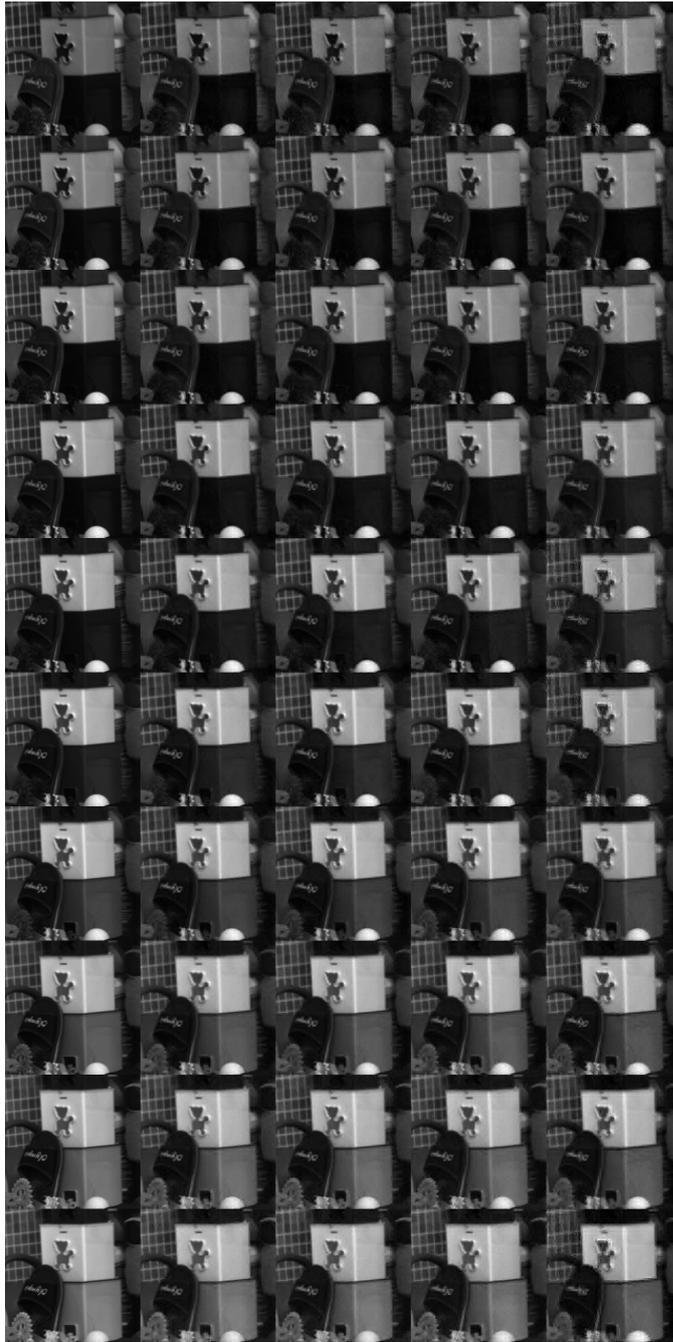
Figure 4.8: Reconstructed spectral images (at 10 wavelengths in the range 530 – 620 nm with 10 nm spacing) from compressive measurements using 2D Daub + 1D DCT prior when input SNR is 30 dB. Left to right: true images, reconstructions with 50%, 60%, 70%, and 80% CR.
