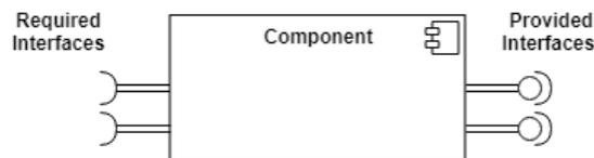
Figure 2.3: Component Interfaces.
