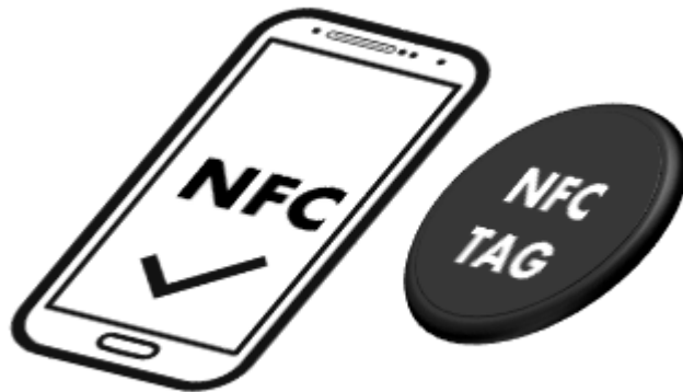
Figure 2.7. An NFC Phone in Reader Mode reads NFC Tag
