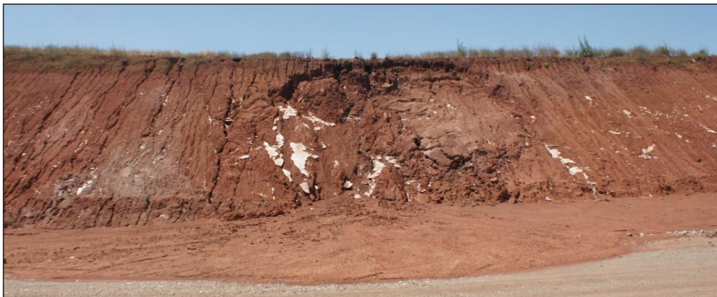
Figure 6.1. Fine evaporite vessels at KM: 121+120 cut slope
