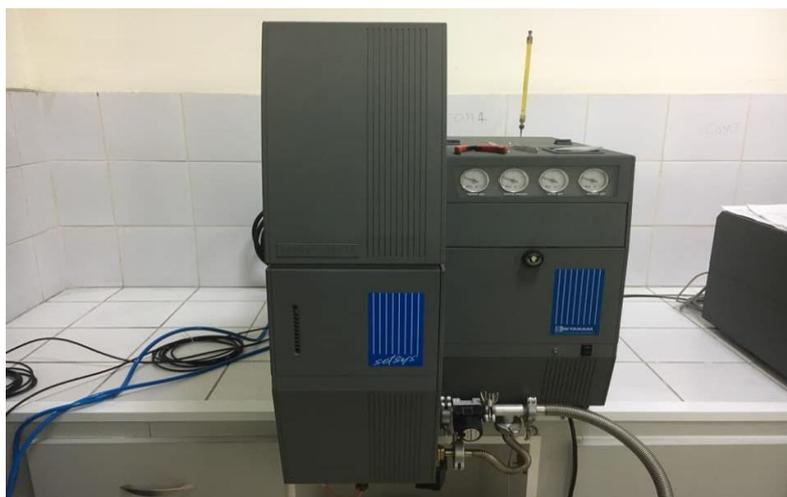
Figure 3.5 Differential Scanning Calorimeter (DSC) Setaram Setsys 16/18
