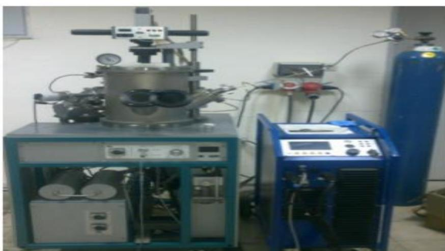
Figure 3.2 Arc melting unit used for the production of samples
