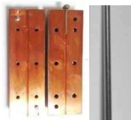
Figure 3.3 Copper mold and cylindrical  $\text{Ni}_{60}\text{B}_{40}$  bulk rod.
