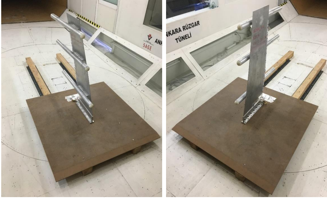
Figure 5-10 Wind Tunnel Test Setup of Configuration-1
