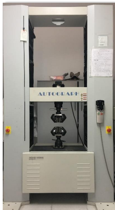
Figure 12. Shimadzu Autograph AG-IS 100kN universal tensile test instrument.
