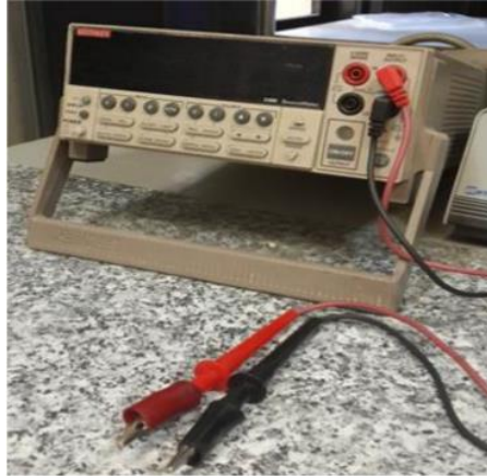
Figure 17. Two-point probe electrical resistivity determiner, Keithley 2400.
