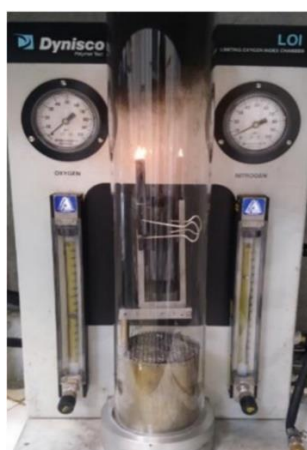
Figure 15. Dynisco polymer LOI test instrument.
