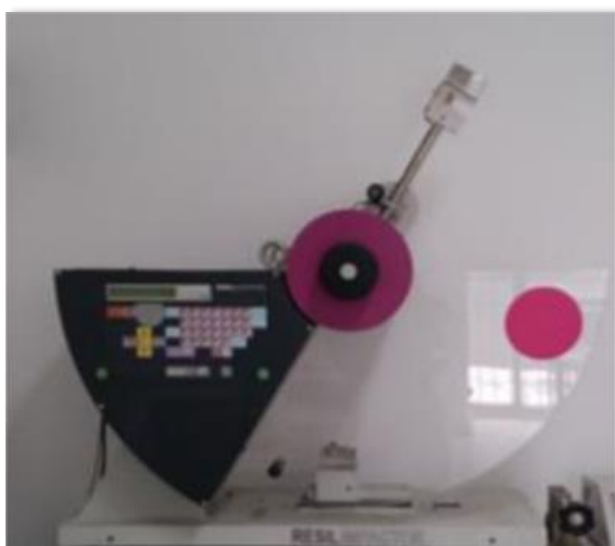
Figure 13. Ceast Resil Impactor 6967 impact test instrument.
