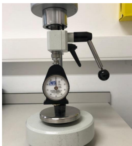
Figure 14. Shore D hardness test instrument.
