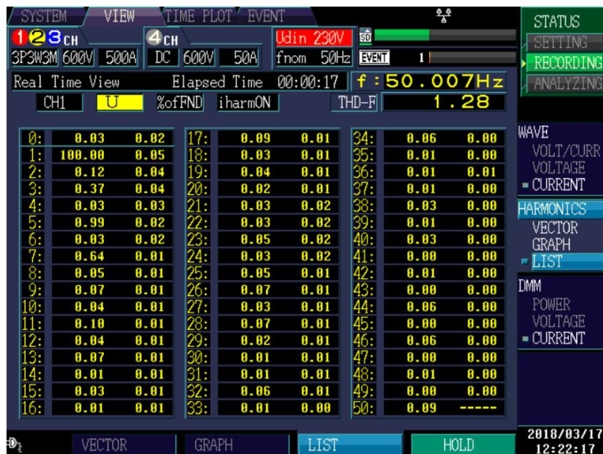
Figure 6. 9. THD value of line to line voltage,  $V_{AB}$  and percentage of each harmonic according to fundamental value
