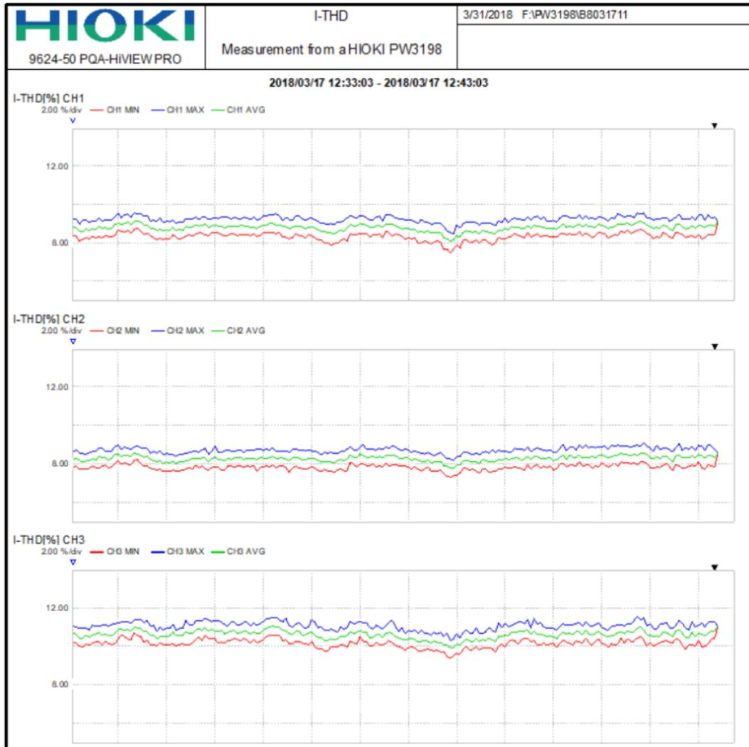
Figure 6. 28. THD values of line currents,  $i_A$ ,  $i_B$ ,  $i_C$  for 10 minutes of record
