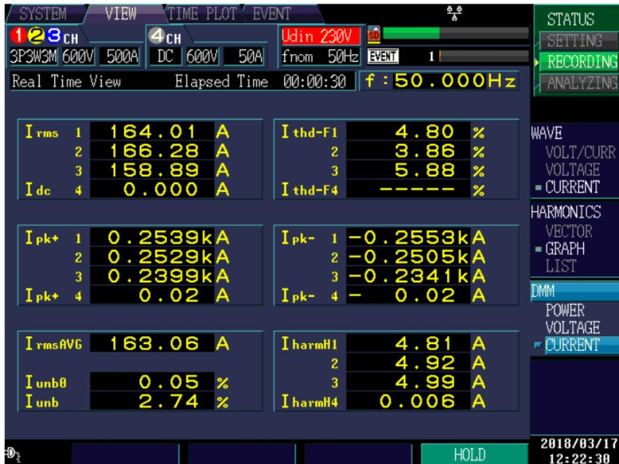
Figure 6. 13. THD values of line currents,  $i_A$ ,  $i_B$ ,  $i_C$
