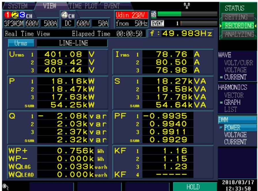
Figure 6. 22. RMS values of line to line voltages, RMS values of line currents, total active power of rectifier, total reactive power of rectifier, total apparent power of rectifier and power factor
