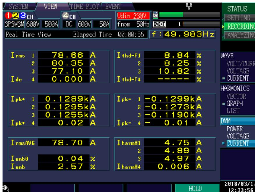
Figure 6. 24. THD values of line currents,  $i_A$ ,  $i_B$ ,  $i_C$
