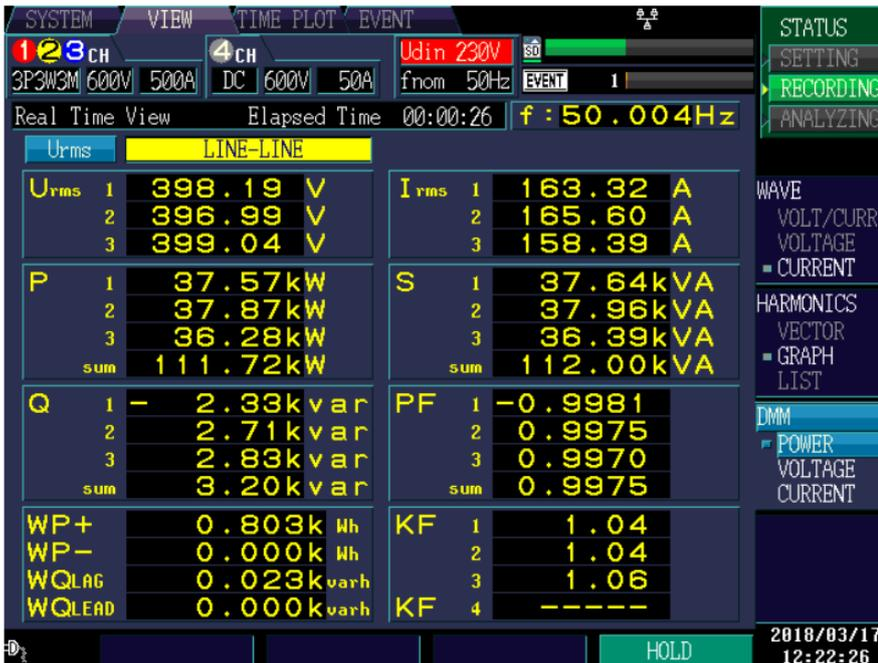
Figure 6. 11. RMS values of line to line voltages, RMS values of line currents, total active power of rectifier, total reactive power of rectifier, total apparent power of rectifier and power factor
