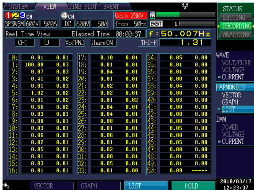
Figure 6. 20. THD value of line to line voltage,  $V_{AB}$  and percentage of each harmonic according to fundamental value
