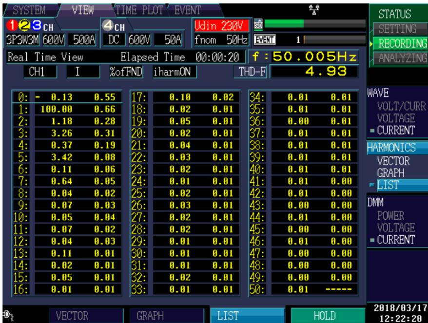
Figure 6. 10. THD value of line current,  $i_A$  and percentage of each harmonic according to fundamental value
