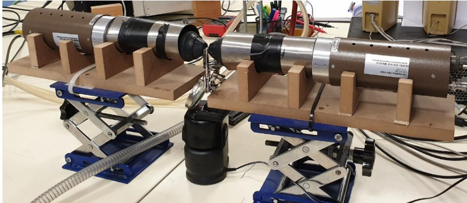
Figure 3.8: The positron annihilation lifetime spectroscopy apparatus. Defects inside the materials were examined with this spectroscopy [92].
