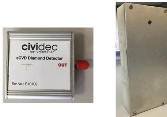
Figure 4.8: Unshielded (left) and shielded (right) diamond detector. The shielding of the detector is Al: 0.25 cm - Pb: 0.40 cm - PE: 0.40 cm from the outside to the inside. Lead and polyethylene layers are embedded inside the light grey aluminum casing. The round detector hole corresponding to the 5.9 mm diameter diamond detector is also visible.
