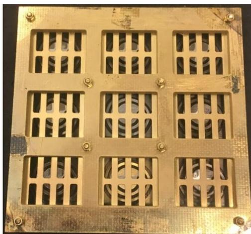
*Figure 3.11.* Mask used for gold back contact coating.
