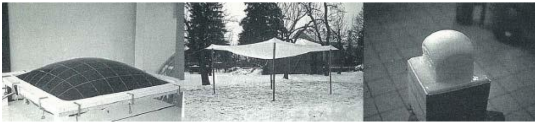
Figure 2.2. Isler's Experimental Forms, based on air pressure, gravity and material flow 58
