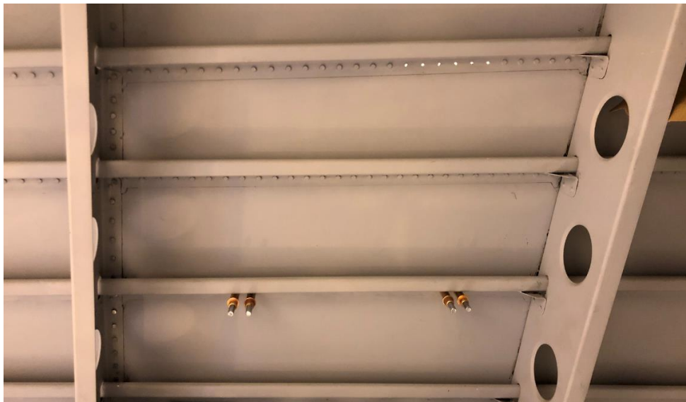
Figure 1.2: Skin-Stringer Structure of a Helicopter
