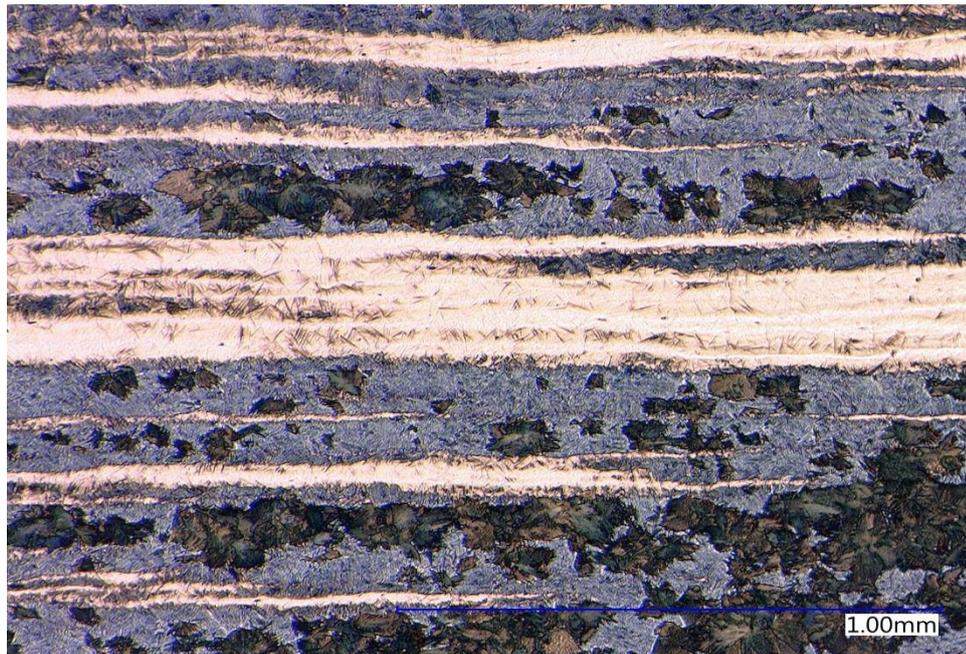
*Figure 4-17. Microstructure of Experiment 10 having the highest banding intensity among the medium cooling experiments (200X, 4% Picral, 60 sec.)*
