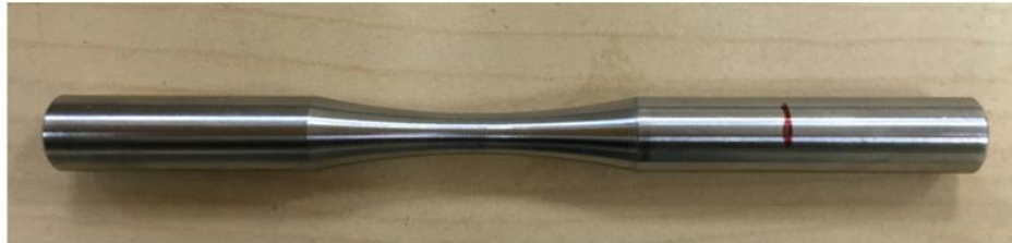
Figure 3.8. Rotating beam fatigue specimen, technical drawing and the actual sample
