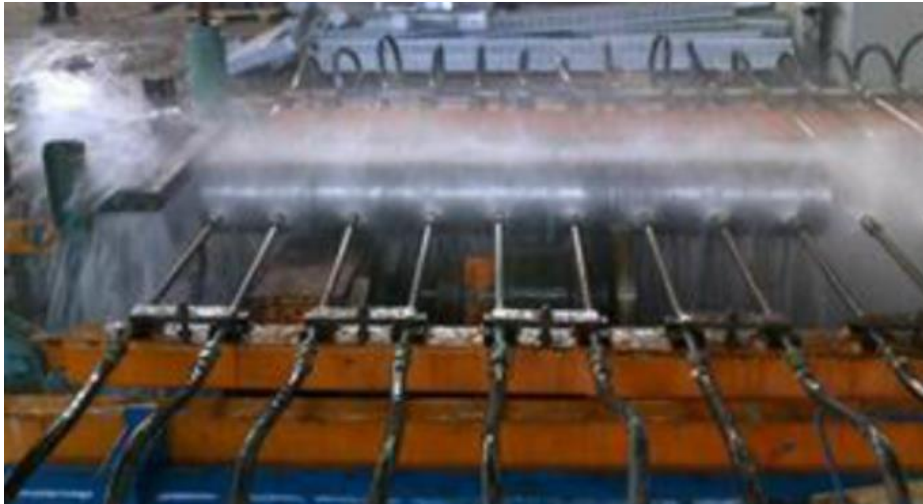
Figure 3.2. Setup used by the entity that manufactured the modified 4340 steel for the water quenching operation
