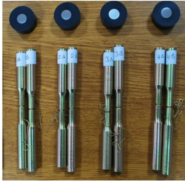
Figure 3.6. Two sets of identical cadmium coated, notched tensile specimens and sections cut to measure thickness molded into Bakelite. Etching and coating parameters are given in Table 3.3
