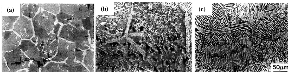
Figure 2-2 Annealed microstructures of (a) 72 at. %Co, (b) 76 at. %Co and (c) 80 at. %Co [22].
