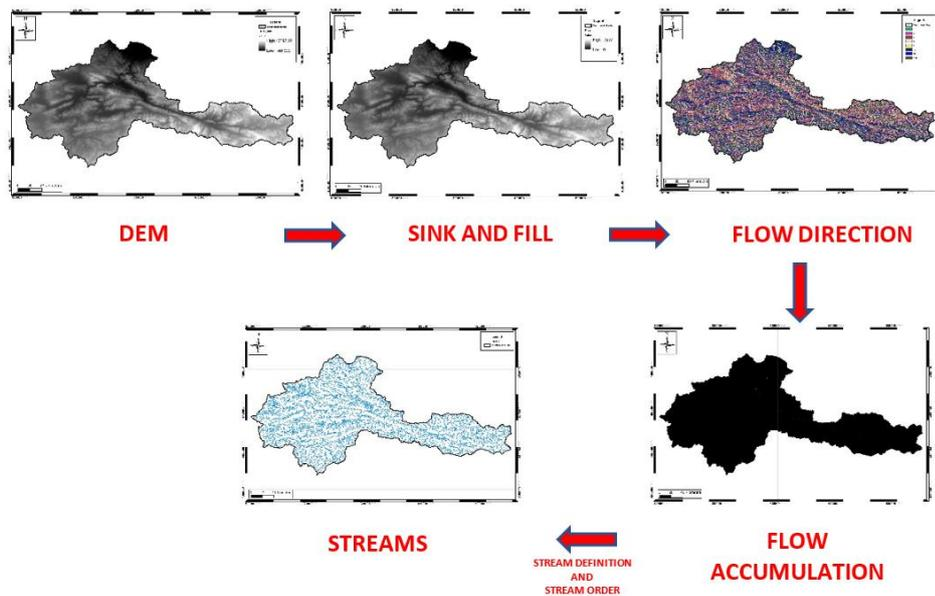
Figure 1.6. Stream Extraction from Digital Elevation Model
