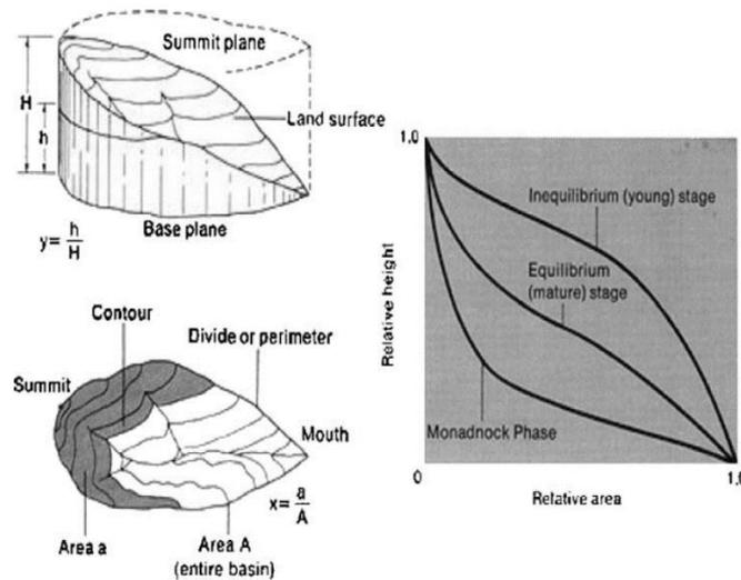
Figure 6.10. Hypsometry Curve and Hypsometry Integral Concept (Ritter et al. 2002)
