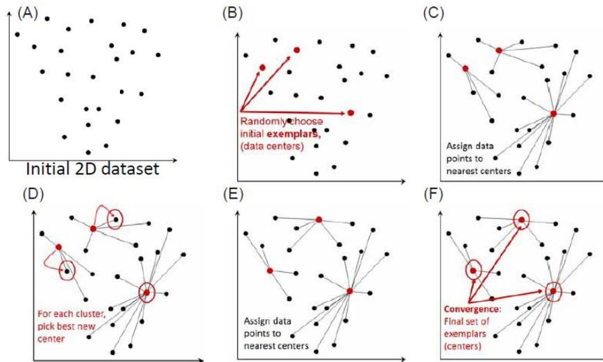
Figure 7.1. K-Means Clustering Algorithm Scheme (Dueck, 2009)
