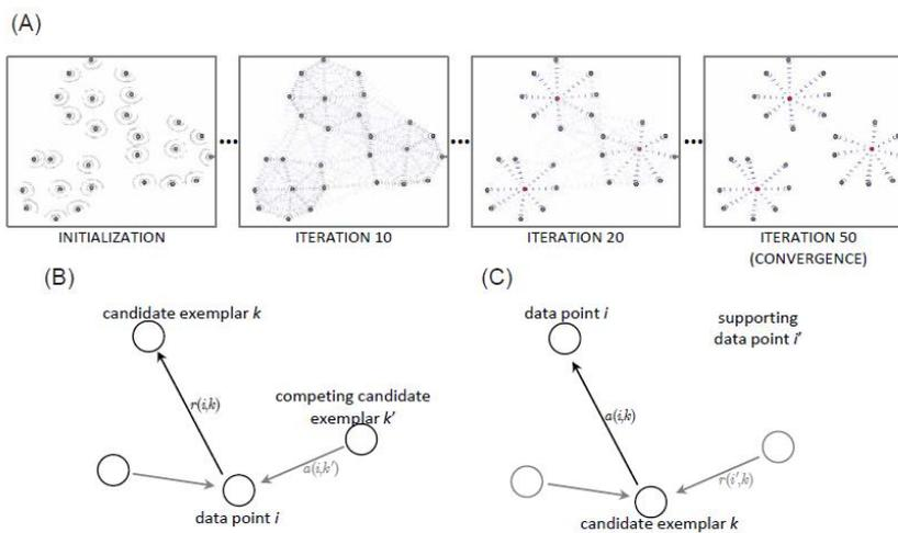
Figure 7.2. Affinity Propagation Clustering Algorithm Scheme (Dueck, 2009)
